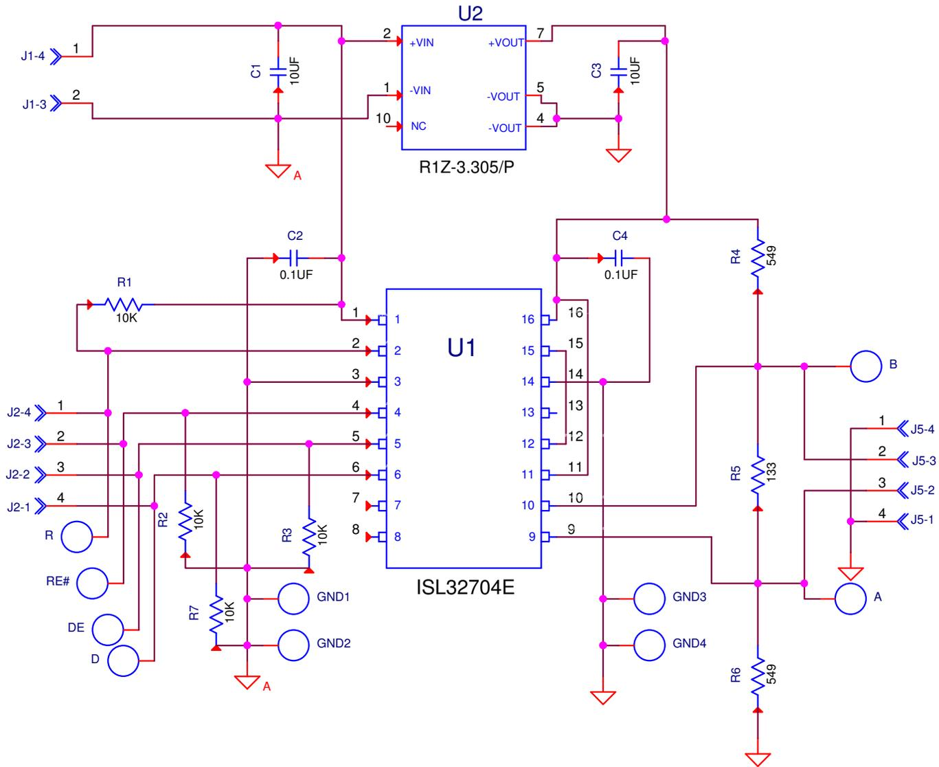
FIGURE 4. ISL32704EVAL1Z SCHEMATIC
