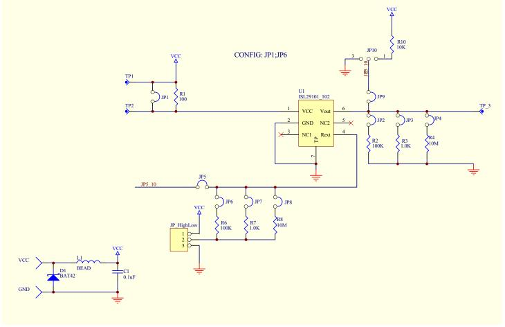
FIGURE 1. ISL291xxIROZ-EVALZ EVALUATION BOARD SCHEMATIC
