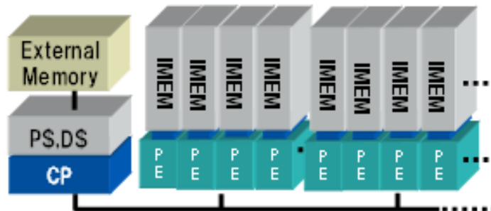
Figure 2 IMAP System Configuration in SIMD Mode
