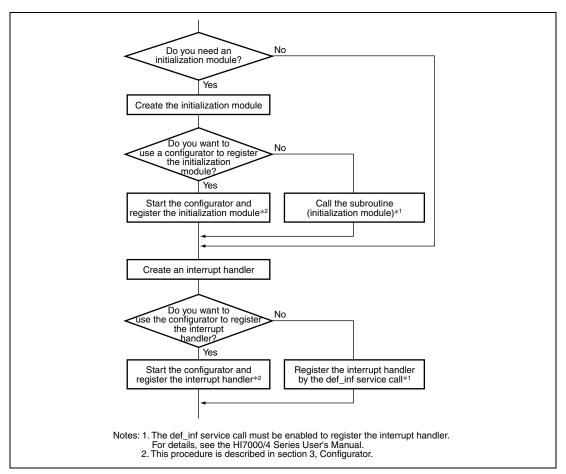
Figure 2.12 Creating and Registering Initialization Module and Interrupt Handler
