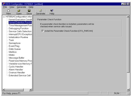
Figure 3.24 Disabling Parameter Check Function
