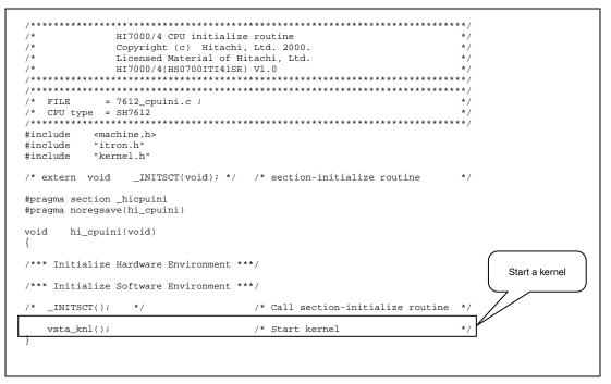
Figure 2.7 Part to be Changed in \_hi\_cpuini (7612\_cpuini.c)
