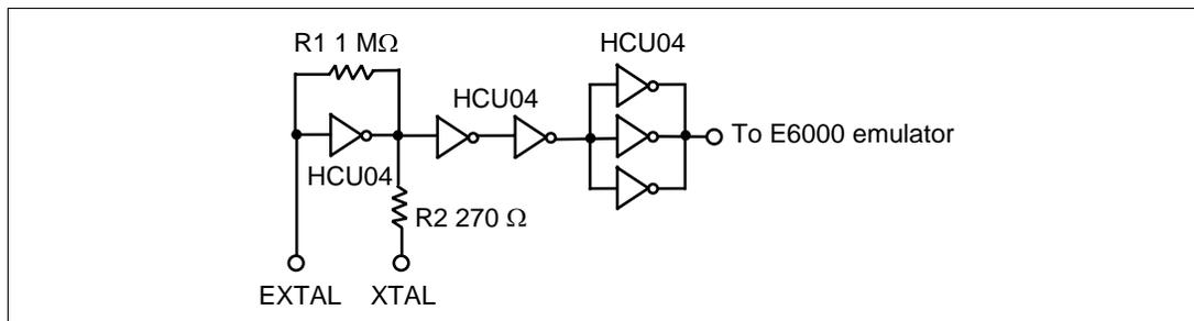
**Figure 9 Oscillator Circuit**
