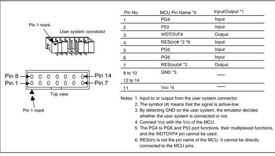
Figure 1.2 Pin Assignments of the User System Connector
