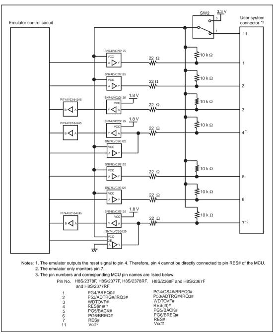
Figure 1.7 Interface Circuit in the Emulator (Reference)
