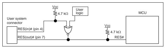
Figure 1.6 Connection of Pin RES#
