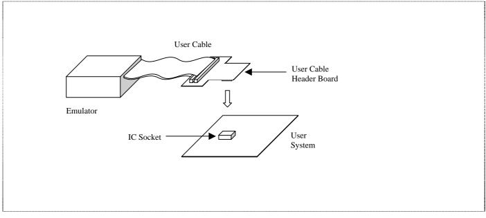
Figure 2.1 Connect User System Interface Cable to the Emulator
