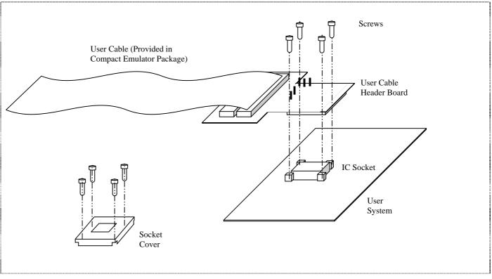
Figure 1.1 SD03UC3048FA0B User System Interface Cable
