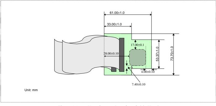
The dimensions for the user system interface cable head are shown in figure 3.2.
