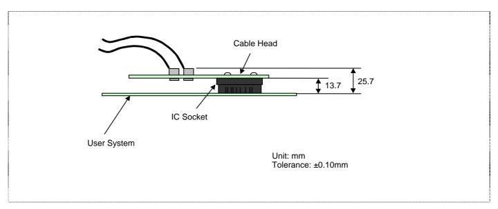
The dimensions after connecting user system interface cable to the user system are shown in figure 3.3.
