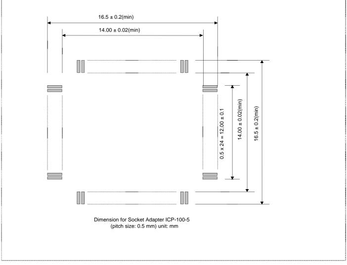
Figure 3.1 PCB Footprint of User System Interface Cable Head
