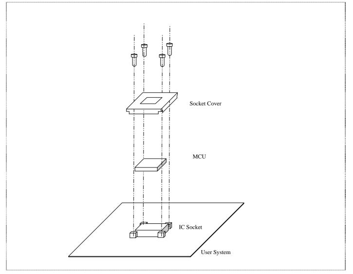
Figure 4.1 Installing MCU to User System
