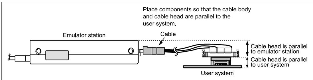
**Figure 10 User System Interface Cable Location Example**
