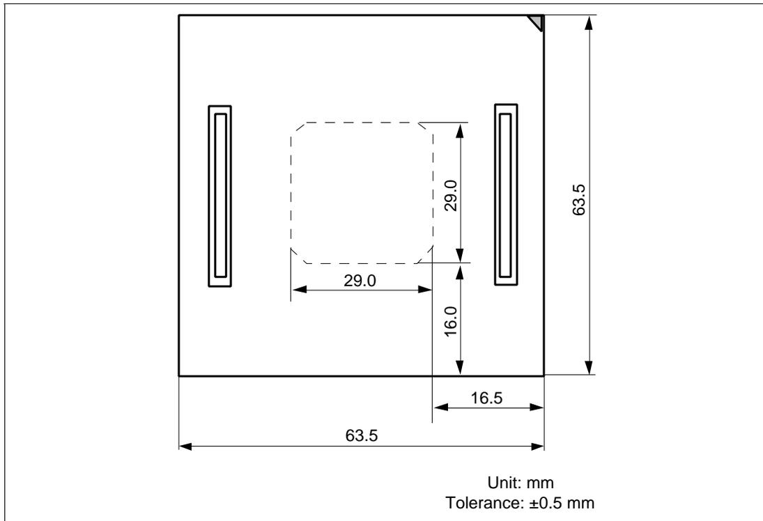
Figure 6 Dimensions for User System Interface Cable Head
