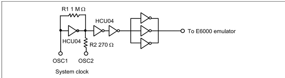
**Figure 9 Oscillator Circuit**
