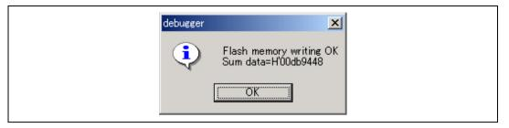
Figure 4.26 Message for Completion of Flash Memory Writing
