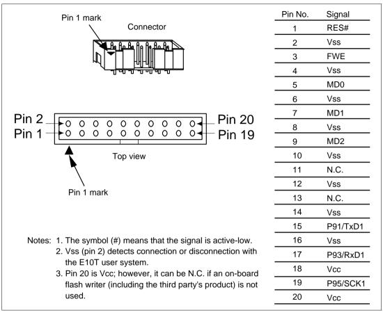
Figure 1.2 Pin Assignments of the Connector
