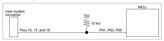
Figure 1.4 Connection of Emulator and MCU
