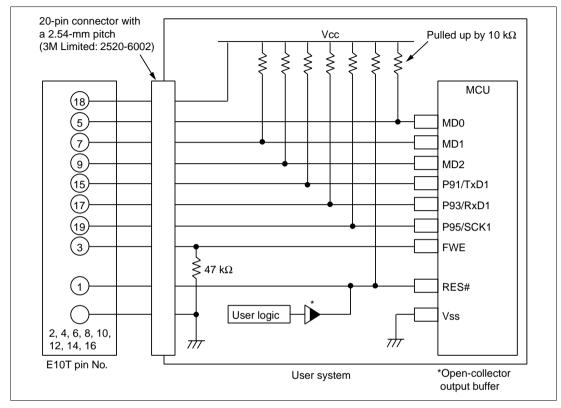
Figure 1.3 Example of Emulator Connection (Mode 7)
