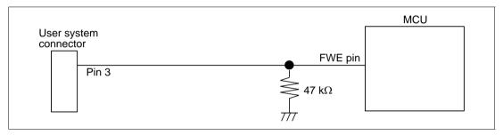
Figure 1.5 Connection of Emulator and FWE Pin
