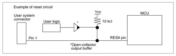
Figure 1.6 Example of Reset Circuits
