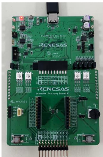
Figure 15. Training Board #2 Connection
