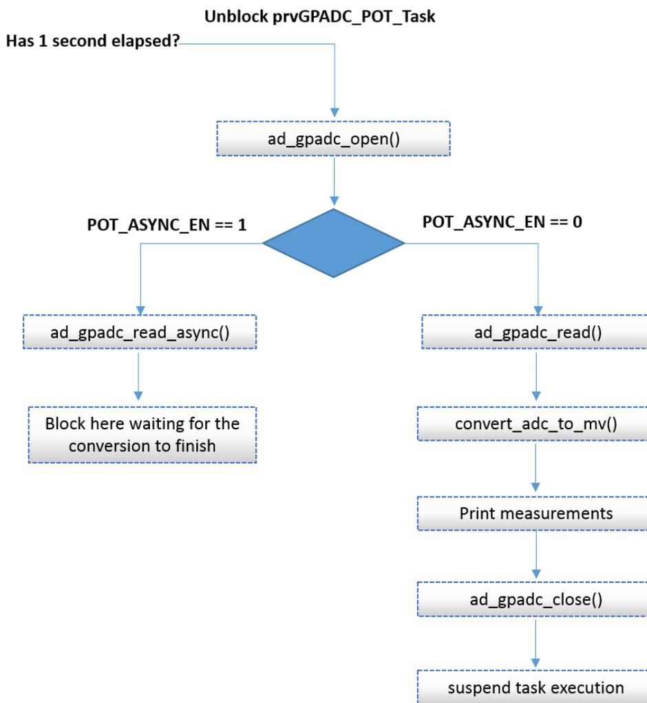
Figure 12: GPADC Conversions SW FSM – Main Execution Path
