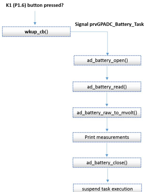
Figure 11: Battery Measurements SW FSM – Main Execution Path
