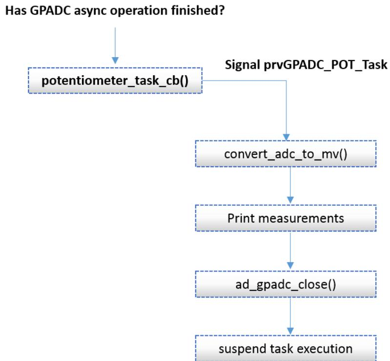
Figure 13: GPADC Async Conversions SW FSM – Callback Function Execution Path
