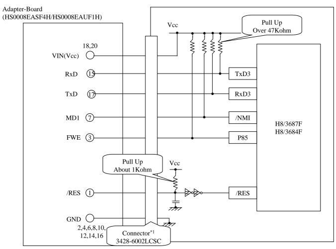
Setting the switches on the HS0008EASF4H on using H8/3687F,H8/3684F
