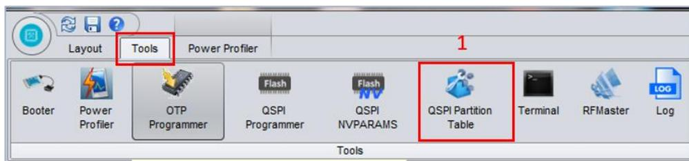
Figure 13: SmartSnippets Toolbox - Display the Partition Table Area
