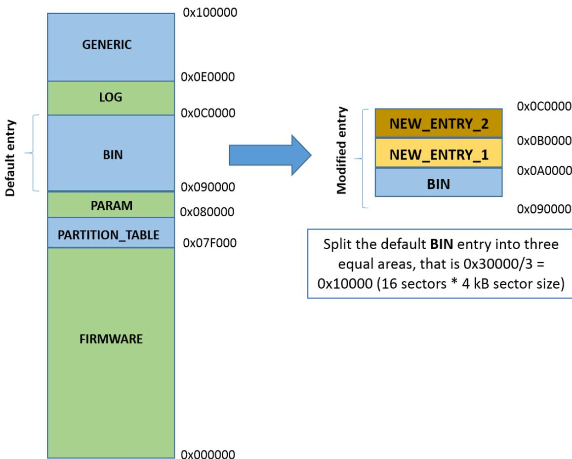
Figure 9: Modifying the 1M Model Partition Table
