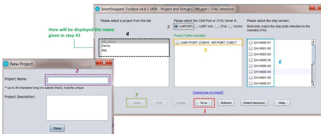
Figure 21: Opening a Project in the SmartSnippets Toolbox
