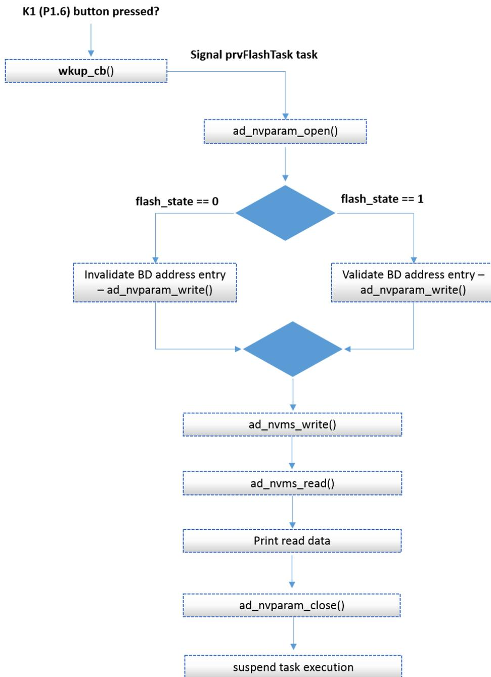
Figure 18: Flash read/write SW FSM – Main Execution Path
