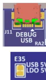
Copper jumper E35 selects the source for the primary power input to the LDO regulator. By default, this jumper is configured to provide power through the Debug USB connector. Copper jumper E35 is closed for this configuration.
