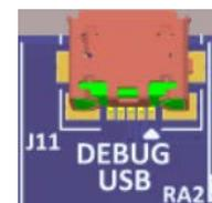
The J-Link OB interface is multiplexed with the JTAG interface, and can collectively be referred to as the Programming Interface. While the J-Link OB interface and the JTAG interface do not conflict, the J-Link OB signals may be isolated from the programming interface by changing the associated copper jumpers.
