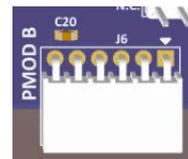
Signals on PMOD B are shared with Main MCU pin header J1 and J2. Care must be taken to ensure that shared signals are not used concurrently.
