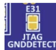
The J-Link OB interface is multiplexed with the JTAG interface, and can collectively be referred to as the Programming Interface. While the J-Link OB interface and the JTAG interface do not conflict, the J-Link OB signals may be isolated from the programming interface by changing the copper jumpers as described in section 5.4.2, Debug USB.
