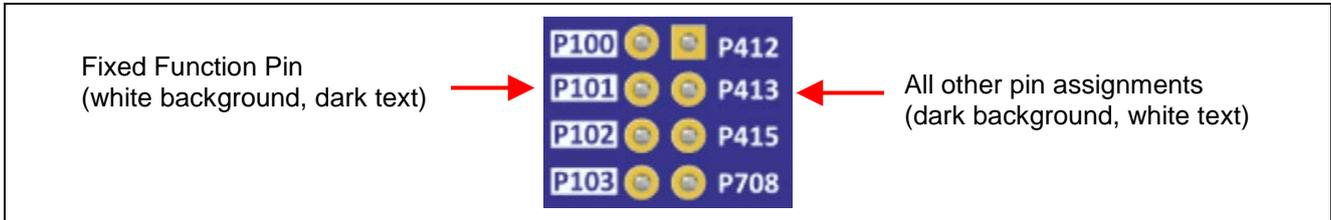
**Figure 24. Fixed Function Pin Label Example**
