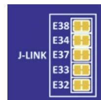
J-Link Disconnect Copper Jumpers E32, E33, E34, E37, and E38 connect the J-Link signals to the MCU programming interface. To isolate the J-Link signals from the JTAG interface, these copper jumpers must be open. To allow use of the J-Link interface, each copper jumper must be closed.
