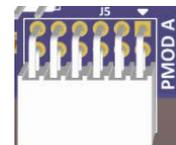
Signals on PMOD A are shared with Main MCU pin header J1 and J2. Care must be taken to ensure shared signals are not used concurrently.
