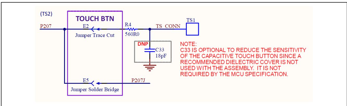
Figure 21. Capacitive Touch Button Circuit
