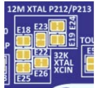
The 32.768 kHz clock crystal may be replaced by an external clock source connected to XCIN. To disconnect the 32.768 kHz crystal, open copper jumpers E25 and E26, and close copper jumper E22.
