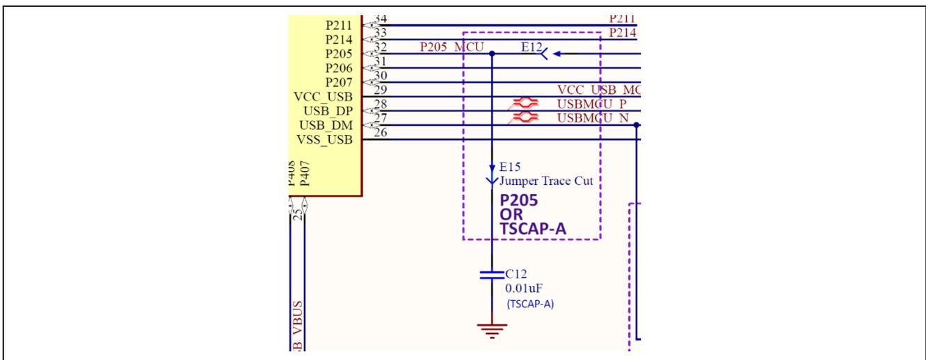
Figure 22. Capacitive Touch TSCAP Circuit
