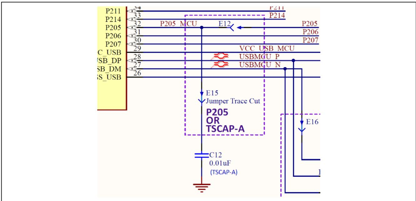
Figure 33. P205 Circuit
