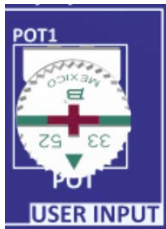
Figure 27. User Potentiometer on the Evaluation Kit Board (top)
