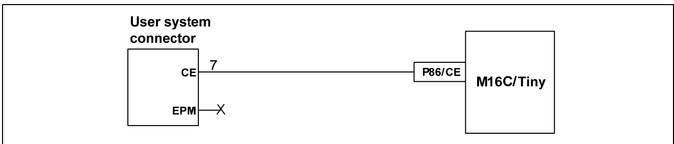
Figure 5.3 Connection of E8 Emulator and Pin P86
