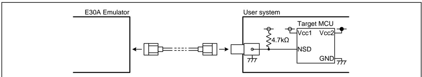
Figure 2.4 Connection Diagram when Using the Coaxial Connector
