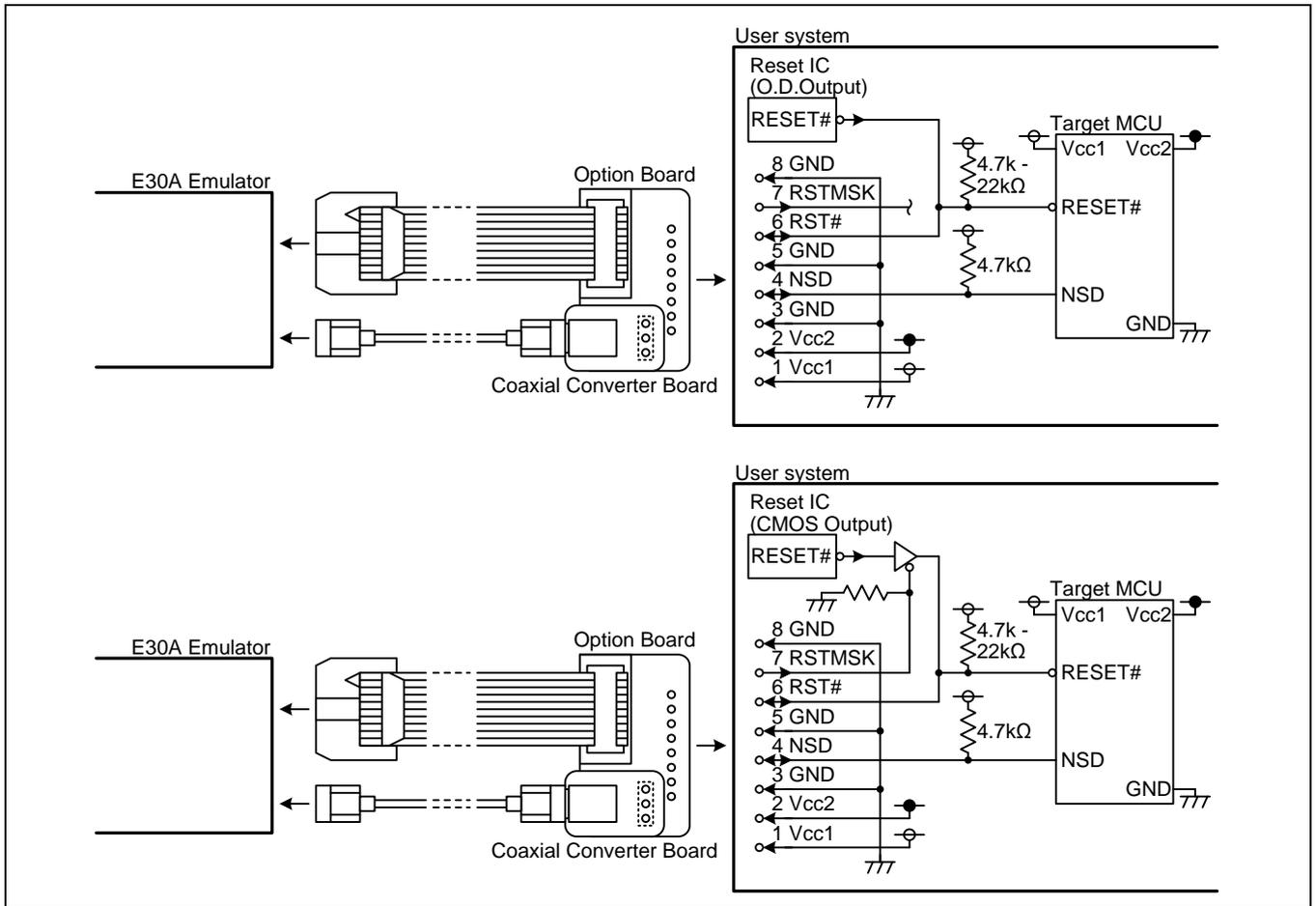
Figure 2.6 Connection Diagram when Using the Option Board
