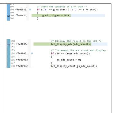
The program proceeds to display the result of the A/D conversion on the LCD and in the terminal window. In addition, the running count of A/D conversions performed is displayed in binary form using LEDs 0-3 on the RSSK. Adjust the potentiometer and press SW1 or SW2 on the RSSK and an additional A/D conversion will be performed.
