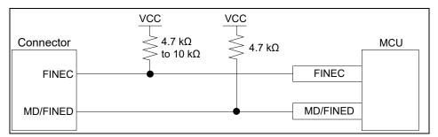
Figure 2.25 Connection of the FINEC and MD/FINED Pins
