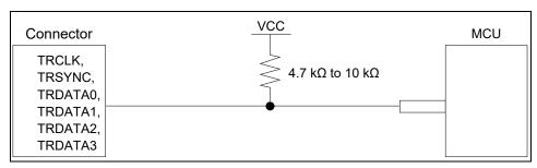
Figure 2.26 Connection of the Trace Pins
