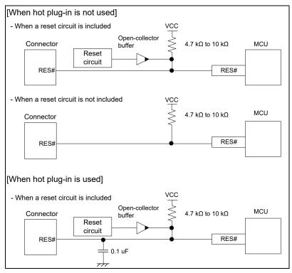
Figure 2.17 Connection of the Reset Circuit
