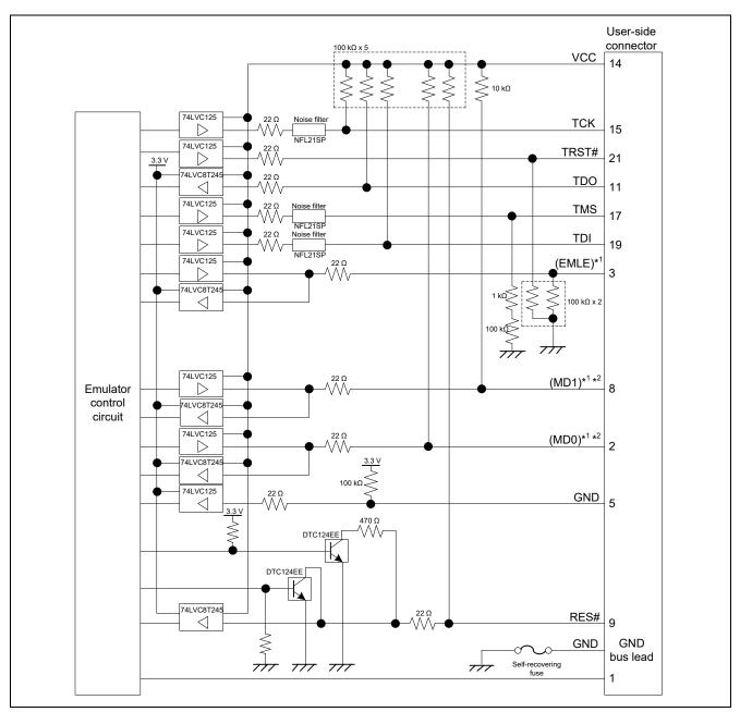
Figure 2.31 shows the internal circuits of the E20 in the tracing circuit section.
