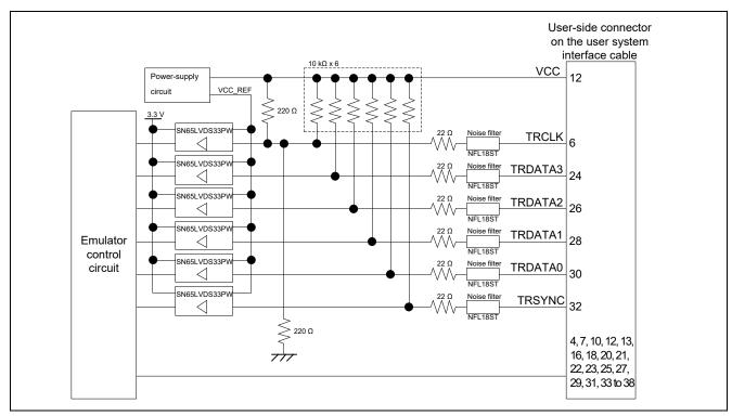
Figure 2.31 Internal Circuits of the E20 in the Tracing Circuit Section
