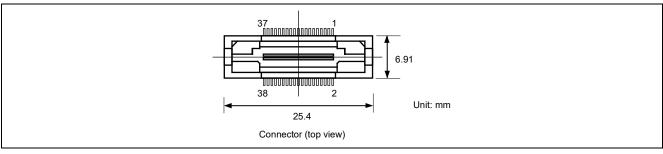
Figure 2.6 Emulator Connector Specifications (38 Pins)
