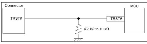
Figure 2.24 Connection of the TRST# Pin
