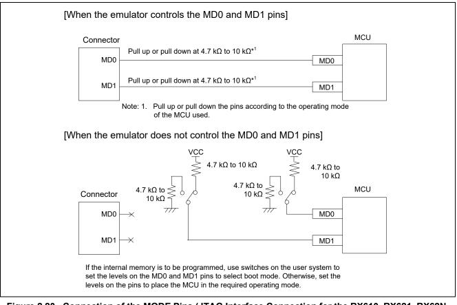
Figure 2.20 Connection of the MODE Pins (JTAG Interface Connection for the RX610, RX621, RX62N, RX62T, and RX62G Groups)
