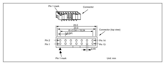
Figure 2.5 Emulator Connector Specifications (14 Pins)
