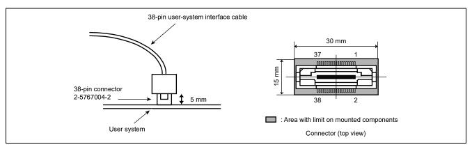
Figure 2.4 Connecting the User System Interface Cable to the 38-Pin Connector of the E20 Emulator
