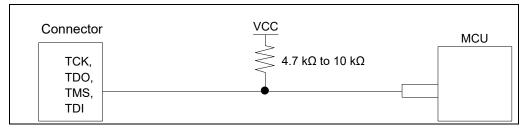
Figure 2.23 Connection of the TCK, TDO, TMS, and TDI Pins
