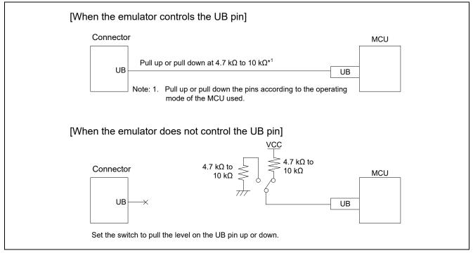
Figure 2.22 Connection of the UB Pin
