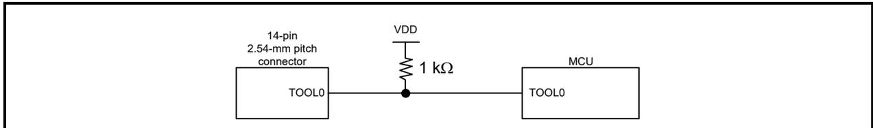
Figure 2-8 Connection Example of the TOOL0 Pin
