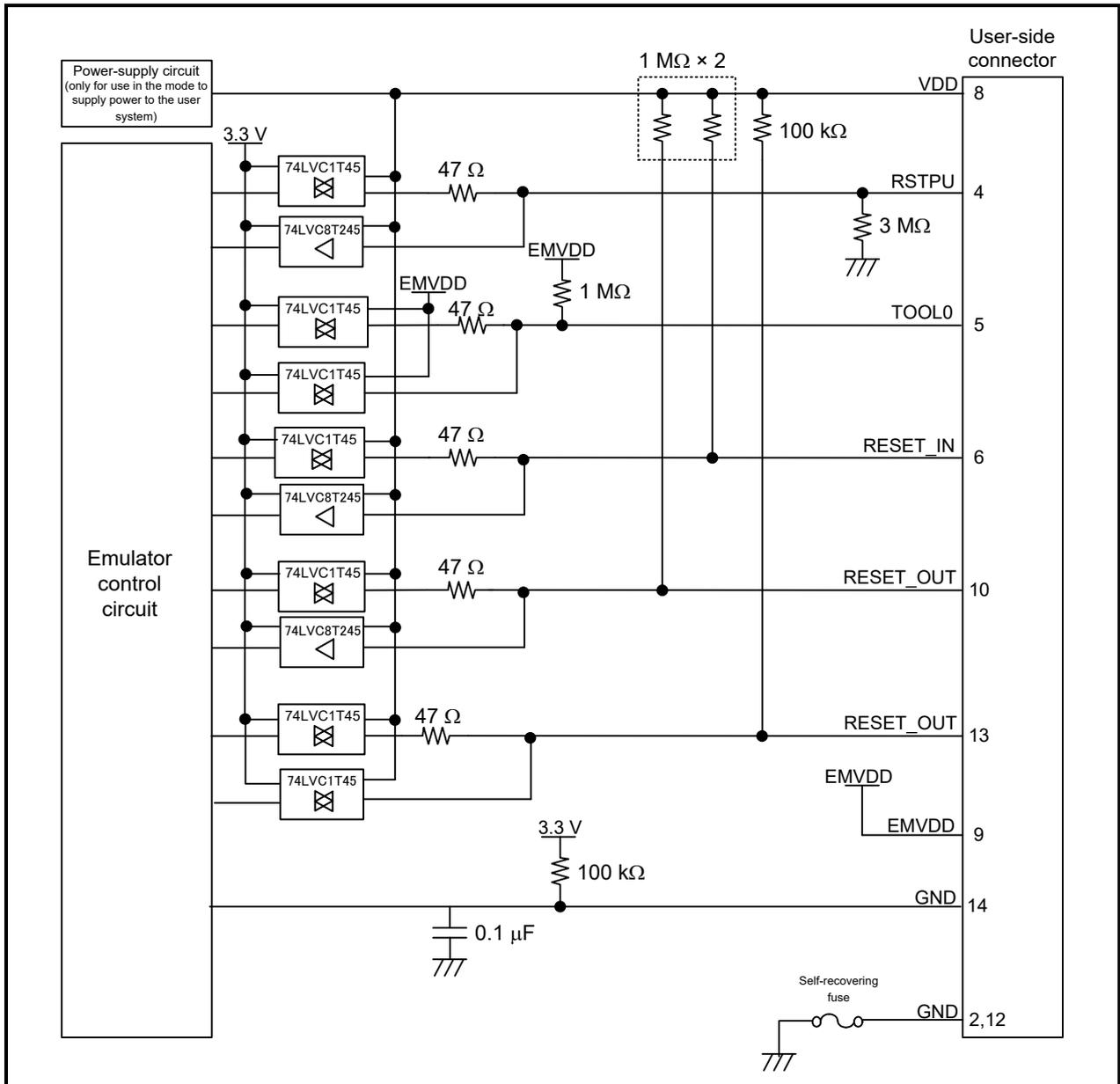
Figure 2-11 Internal Circuits of the E2 (RL78 Family)
