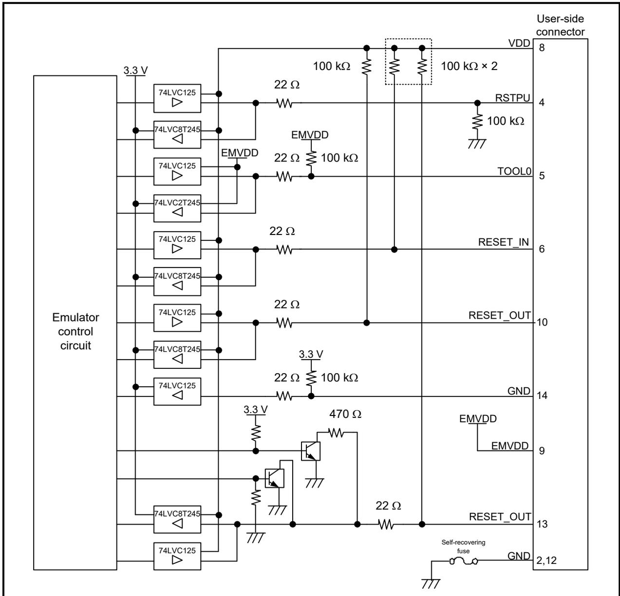
Figure 2-10 Internal Circuits of the E20 (RL78 Family)
