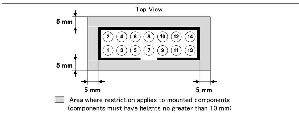
Figure 2-1 Area where Restriction Applies to Mounted Components
