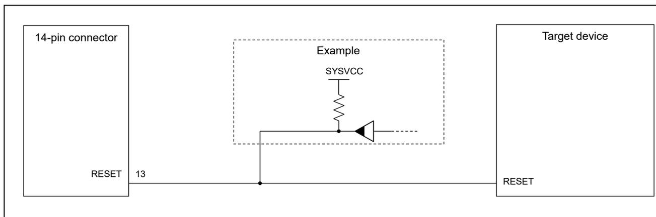
**Figure 2-7 Example of Connecting Reset Circuit**
