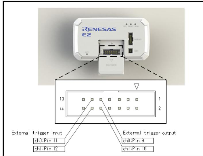
**Figure 3-1 Expansion Interface of the E2 Emulator**
