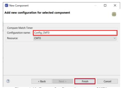
Figure 4-12 Ensure Configuration name - CMT0
