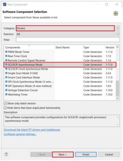
Figure 4-33 Select SCI/SCIF Asynchronous Mode
