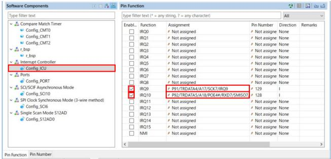
Figure 4-50 Configure pin assignment - Config\_ICU
