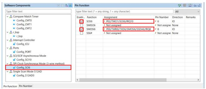
Figure 4-52 Configure pin assignment - Config\_SCI6
