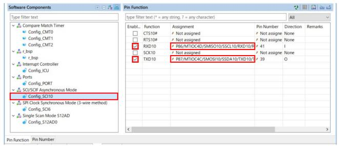
Figure 4-51 Configure pin assignment - Config\_SCI10
