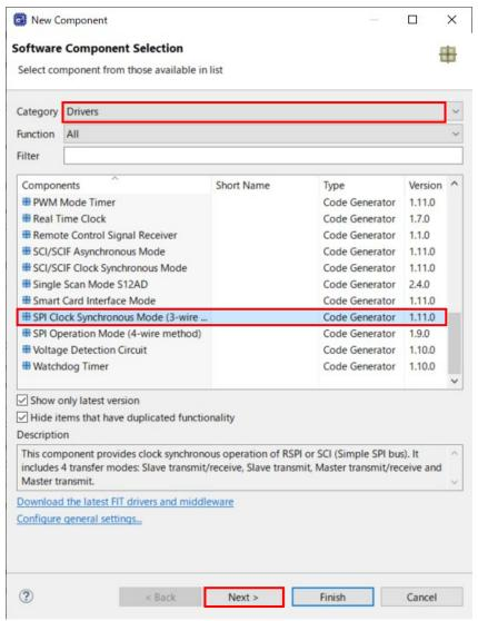
Figure 4-38 Select SPI Clock Synchronous Mode
