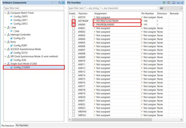
Figure 4-53 Configure pin assignment - Config\_S12AD0
