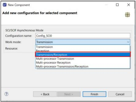
Figure 4-34 Select Work mode - Transmission/Reception
