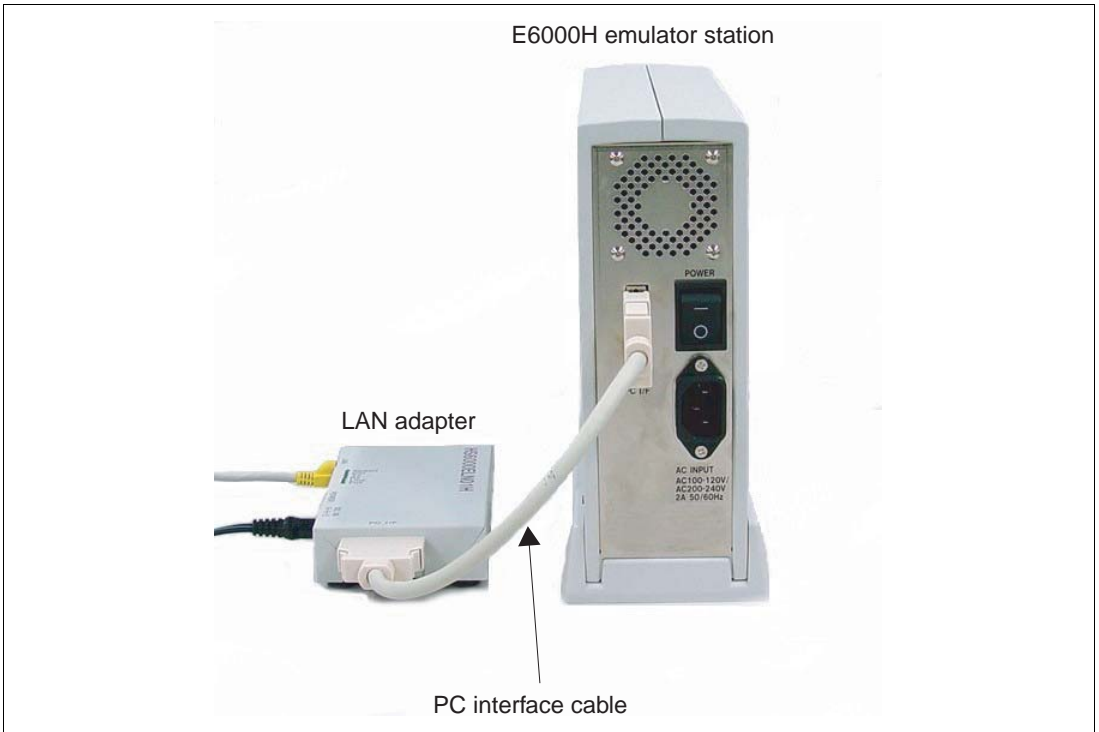
Figure 3.4 Connecting LAN Adapter to E6000H Emulator
