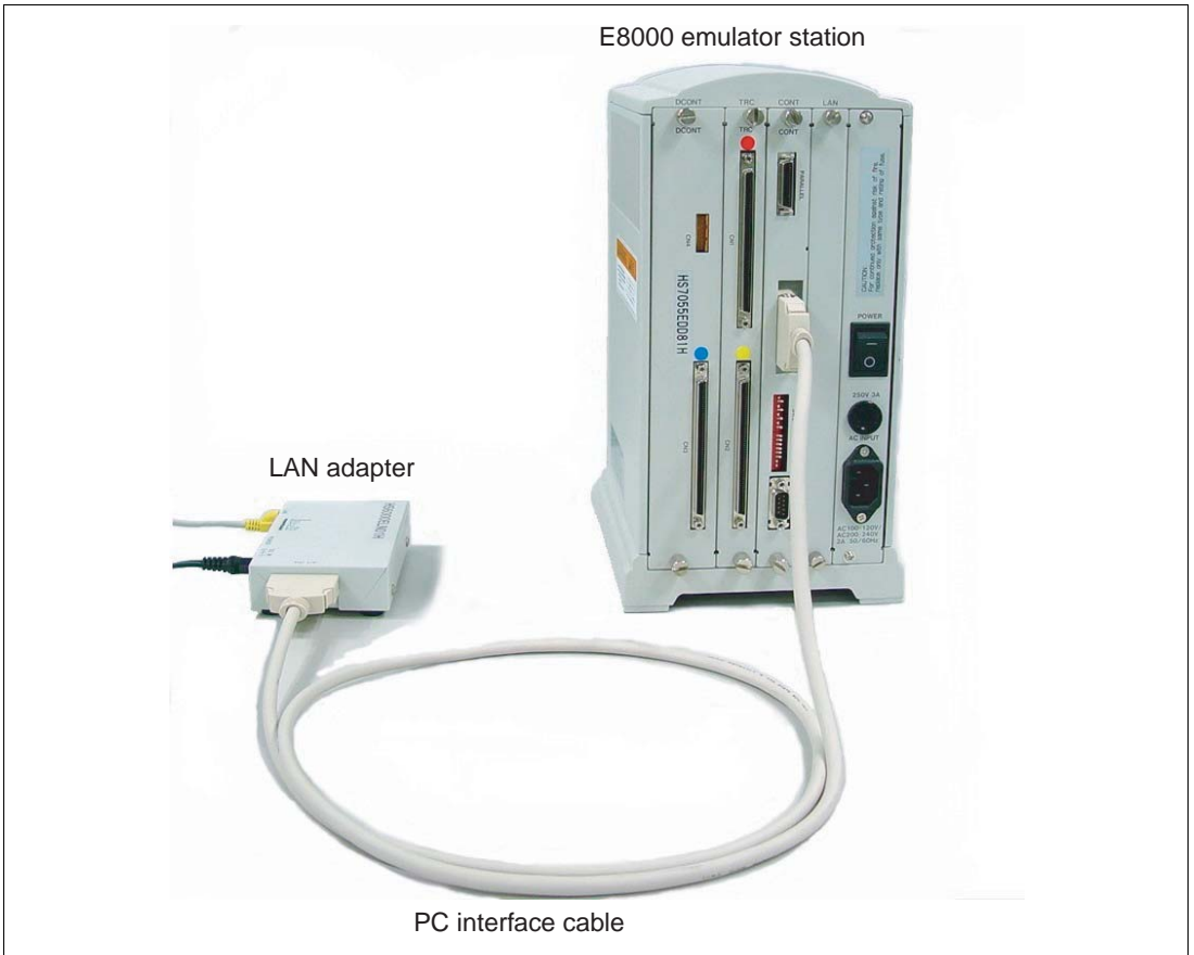
Figure 3.5 Connecting LAN Adapter to E8000 Emulator
