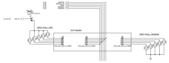
Figure 7: GPIOs control schematics
