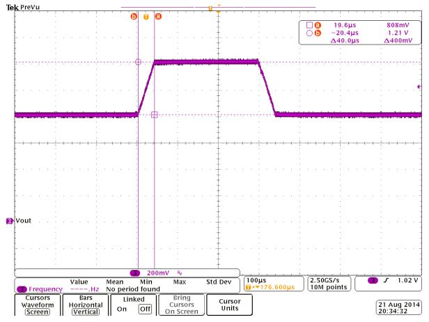
Figure 16: DVC transition of the buck
