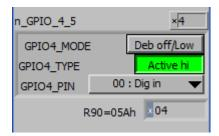
You can simply change the connection of the green cable in Figure 17 and this will be reflected into a change of the output voltage of buck 1 between VBUCK1\_CTRL\_A and VBUCK1\_CTRL\_B. So the BUCK SEL bit functionality has been replaced by the GPI4 input port.
