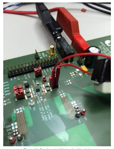
Figure 12: Sensing the LX signals of buck A
