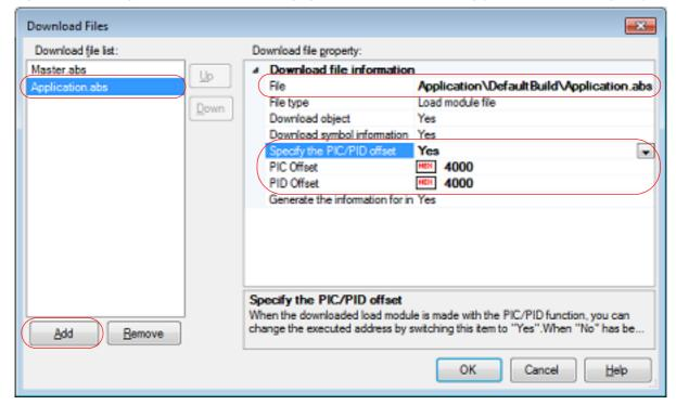
When the load module is downloaded after the values of [PIC Offset] and [PID Offset] have been changed, the allocation of addresses for the P section and external or static variables is changed as shown in the figure below.
