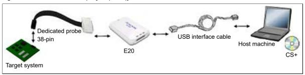
Figure 2.3 Connection Example [E20(Serial)]
