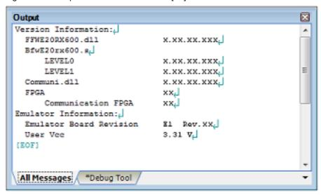
Figure 2.57 Output Panel after Connection [E2 Lite]
