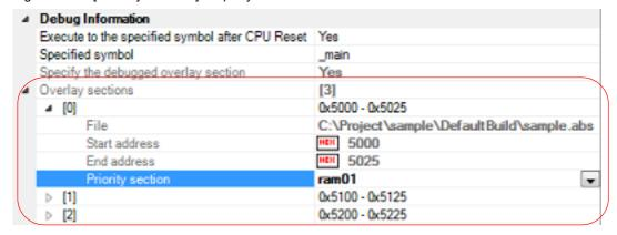
This property shows the current information of overlay sections per address group in detail. Only [Priority section] can be changed.
