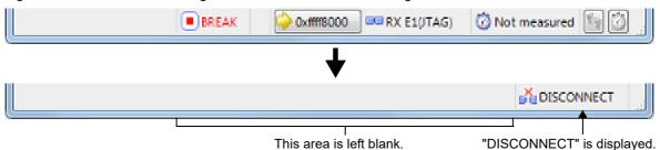
**Caution 1.** The debug tool cannot be disconnected from CS+ while the program is running. If you wish to disconnect the debug tool, stop the program in advance.
