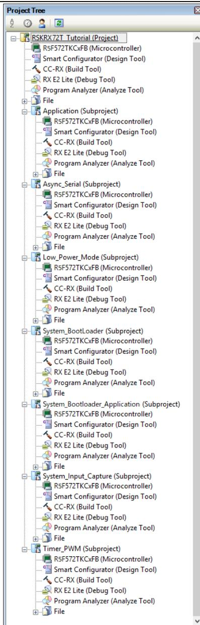
Note: 'Smart Configurator (Design Tool)' node is shown in the 'Project Tree' and indicates an optional plug-in has been enabled previously.
