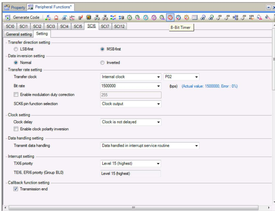
Figure 4-10 SCI6 SPI Master Setting
