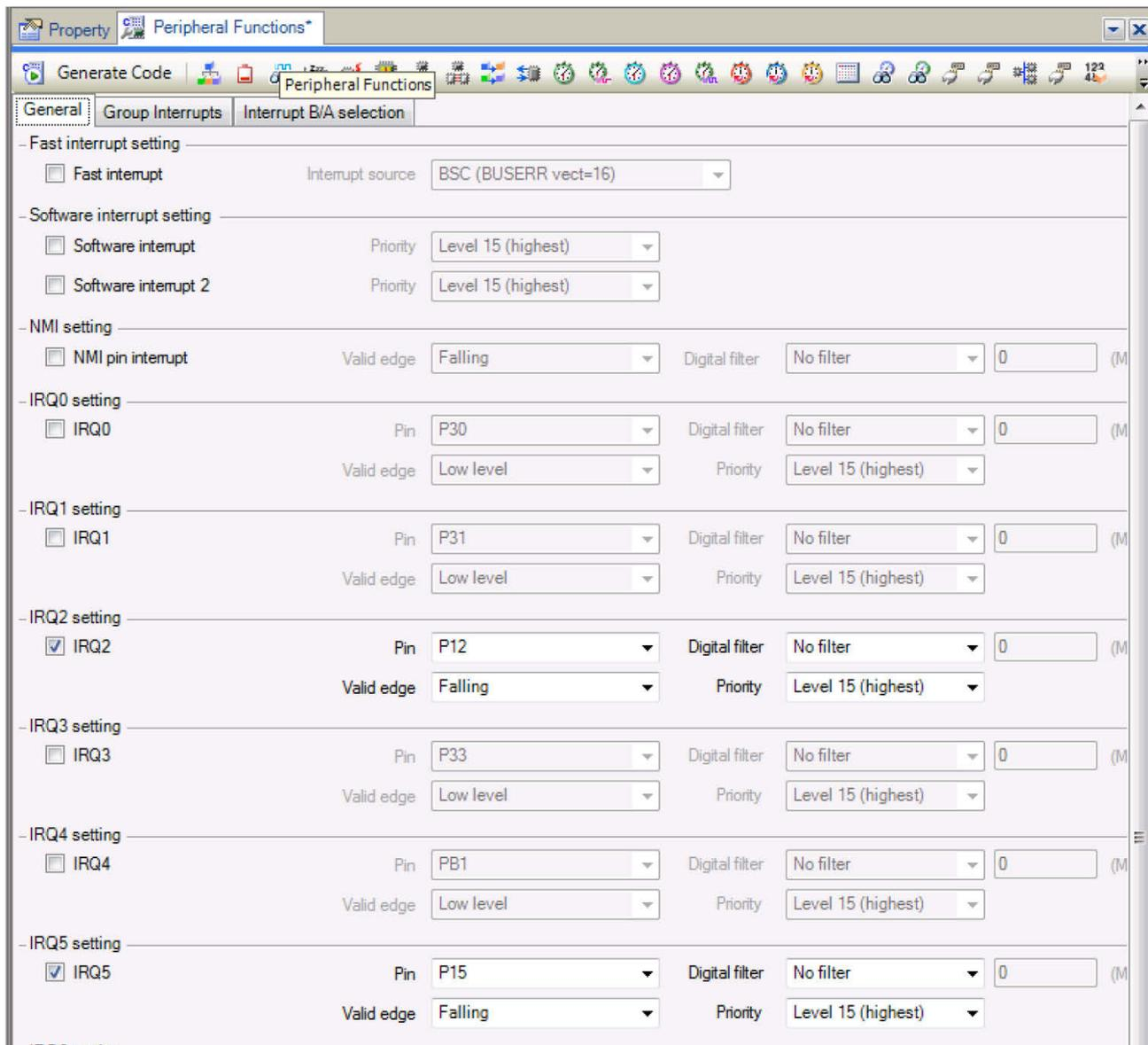
**Figure 4-3 Interrupt Functions tab**
