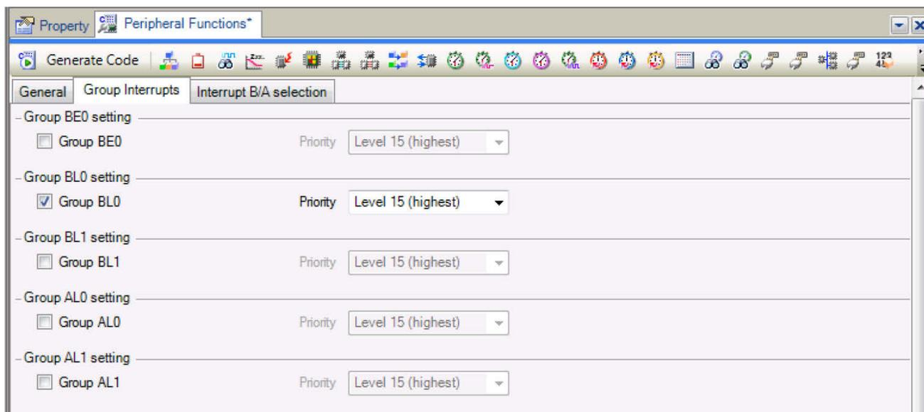
Figure 4-4 Group Interrupt Functions tab
