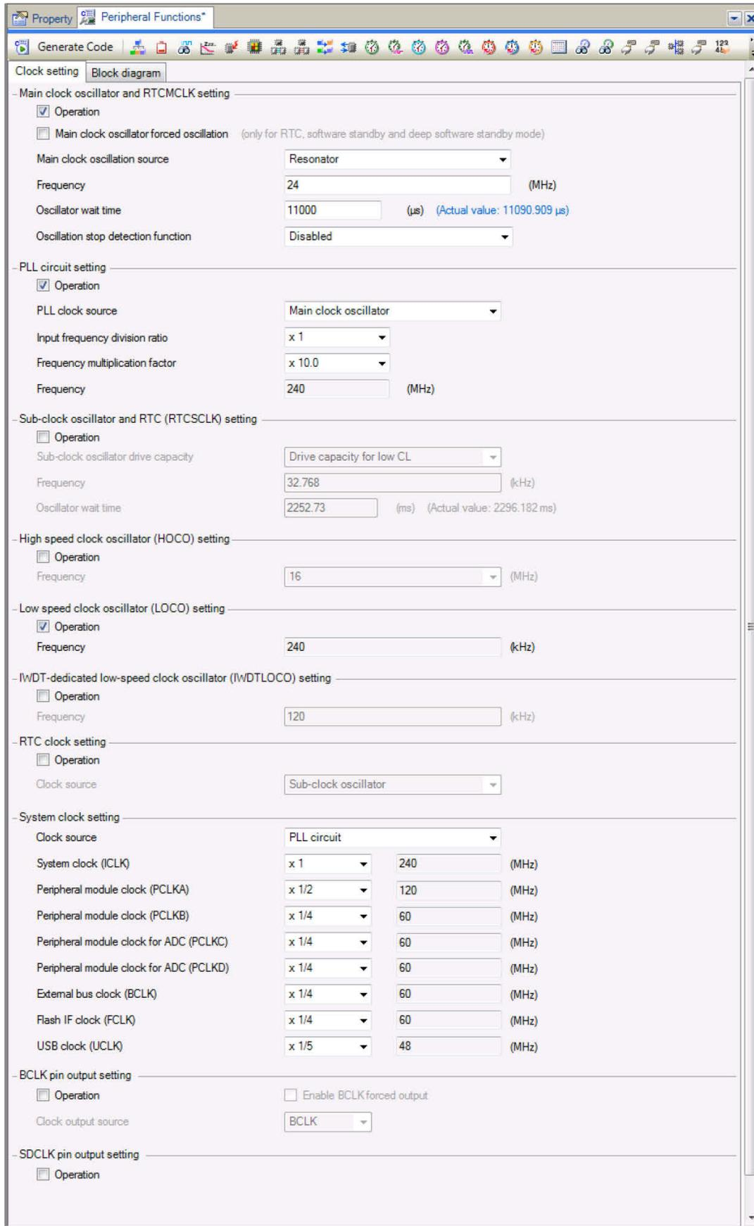
Figure 4-2 Clock setting tab
