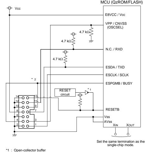
\*2 : To write data on the Flash ROM and QzROM using the same IC socket board / user board, connect Pin No. 4 and No. 9.
