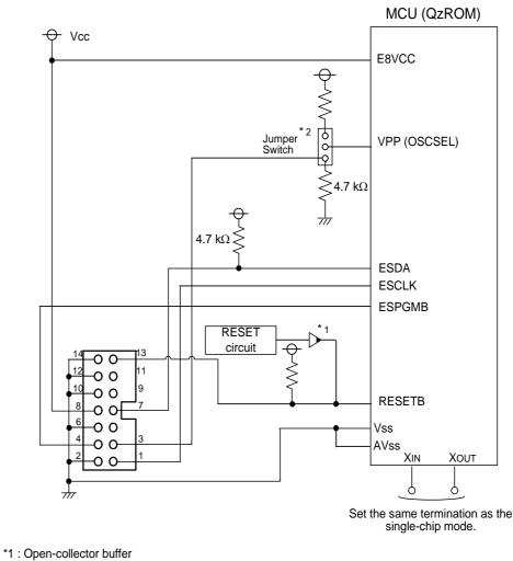
\*2 : When programming QzROM is performed, disconnect Vcc from OSCSEL by a jumper switch.
