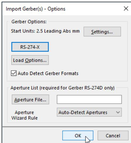
If the file is not imported properly, change the file format to RS-274 or Fire9000 and check the options selected under the “Load Options” button as shown in Figure 8.
