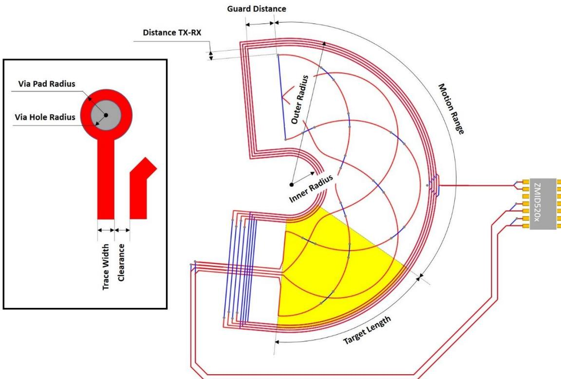
**Figure 6. Rotary Design Help Diagram**
