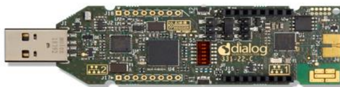
Figure 25. DA14695 USB Kit components with ZOR antenna
