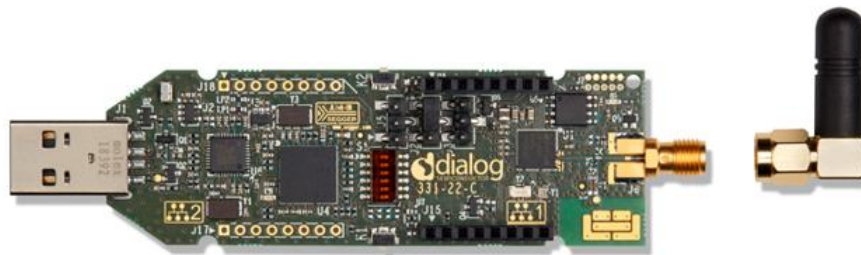
Figure 24. DA14695 USB Kit hardware components with external antenna
