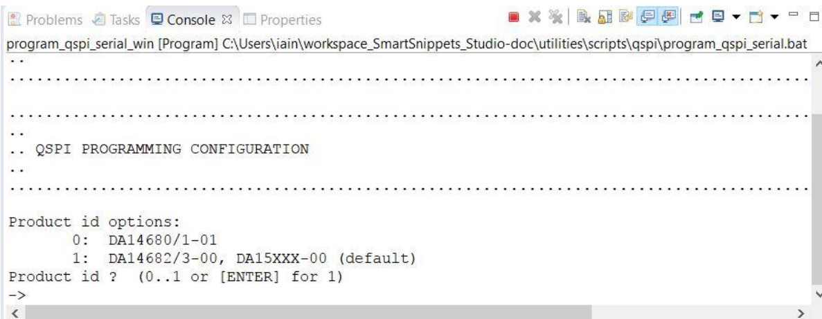
Figure 7: QSPI programming configuration
