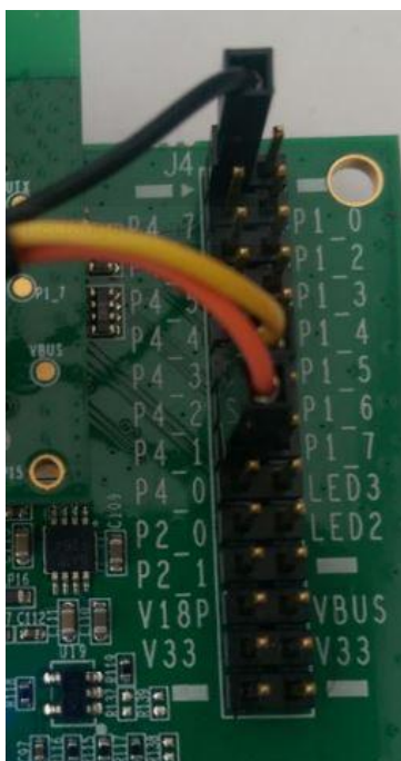
Figure 16: Connecting USB-UART cable to UART2
