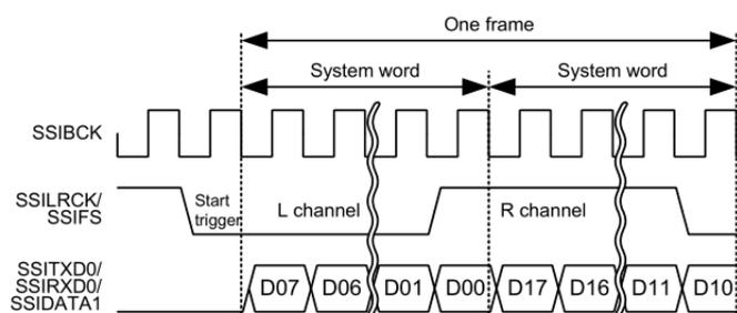
Figure 184: SSI Frame Diagram (8-bit word, 8-bit samples)
