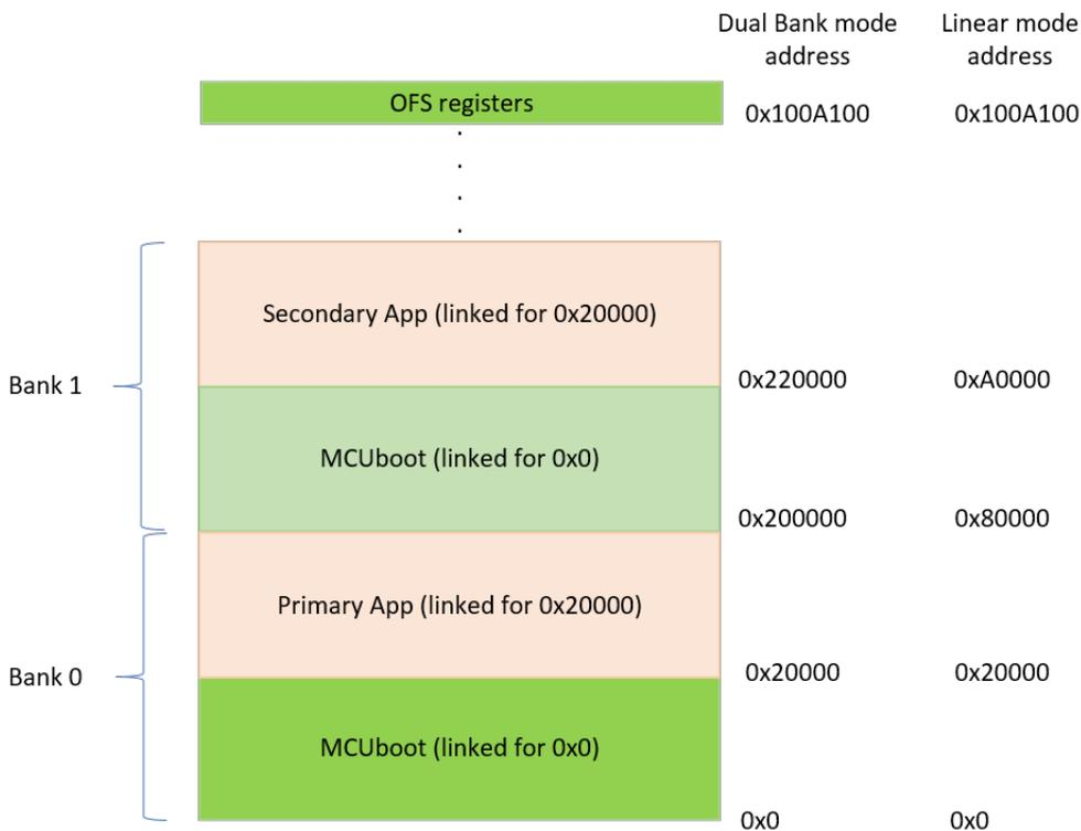
Figure 150: MCUboot Dual Bank layout for 1 MB Memory
