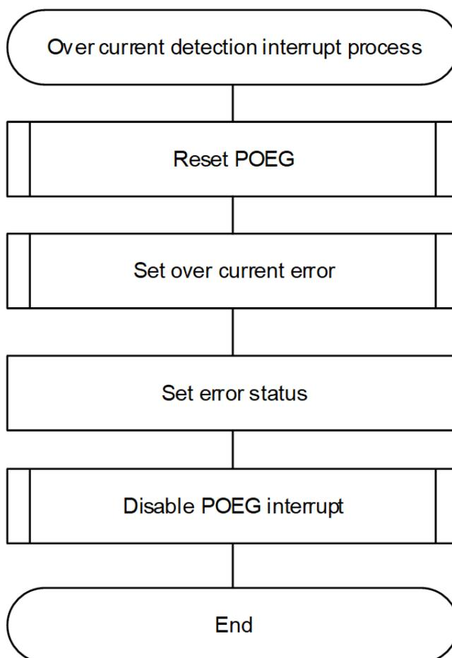
Figure 229: Over current detection interrupt process
