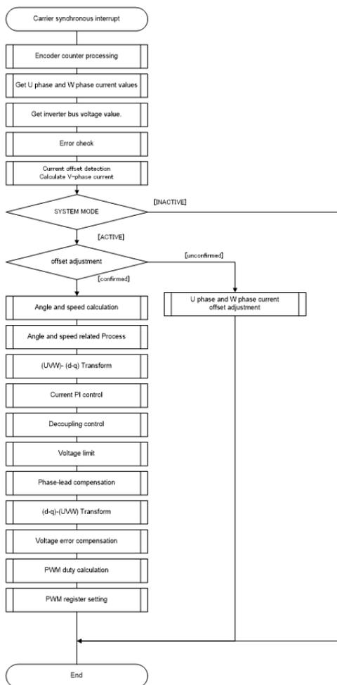
Figure 236: Current control process
