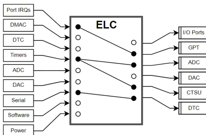
Figure 282: Event Link Controller Conceptual Diagram
