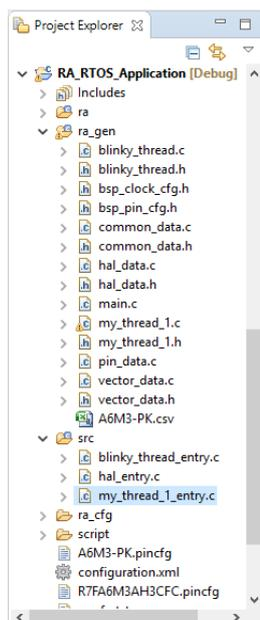
Figure 53: Generated files for an RTOS application
