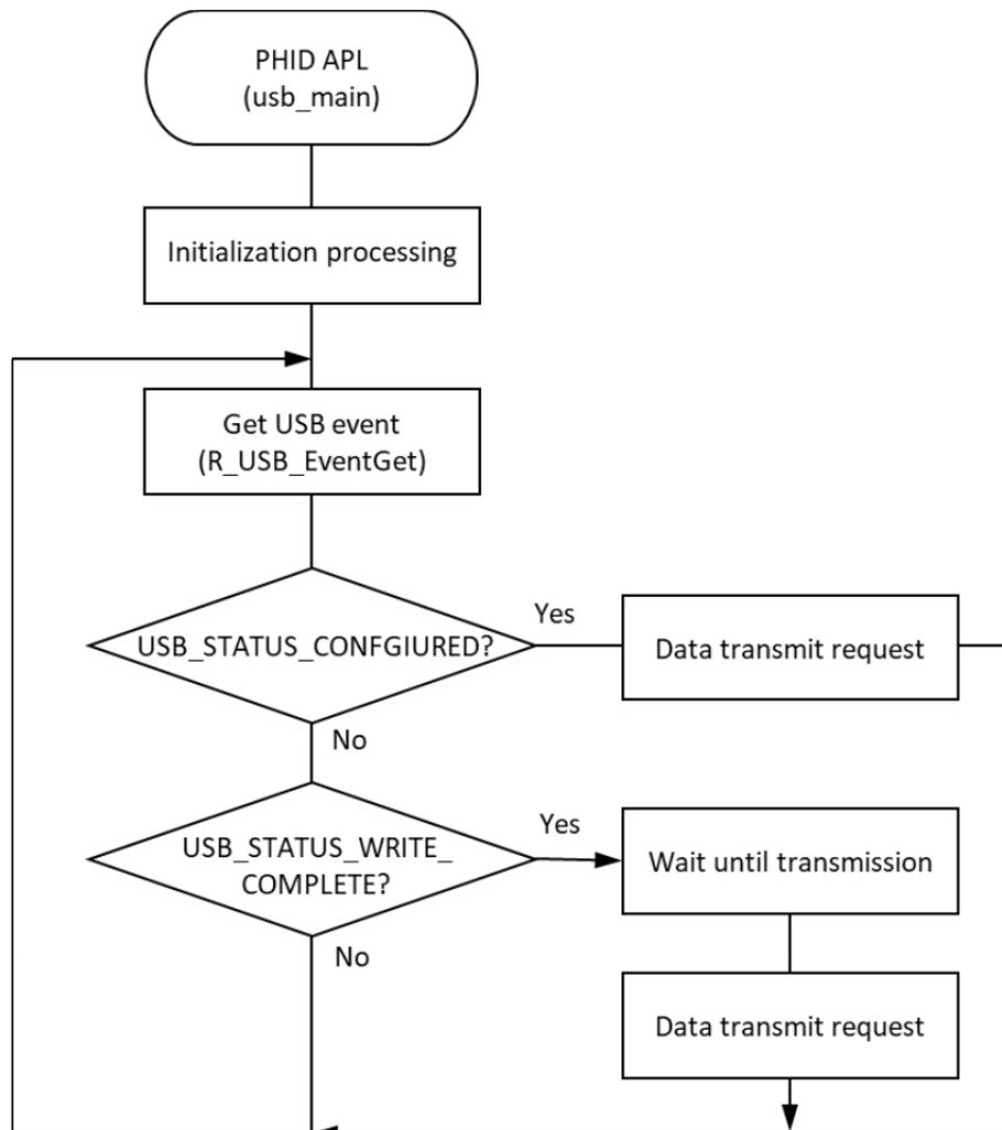
Figure 207: Main Loop processing for non-RTOS example
