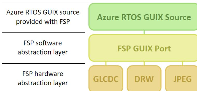
Figure 213: Azure RTOS GUIX Port Block Diagram
