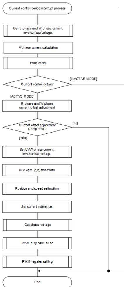
Figure 247: Current control process
