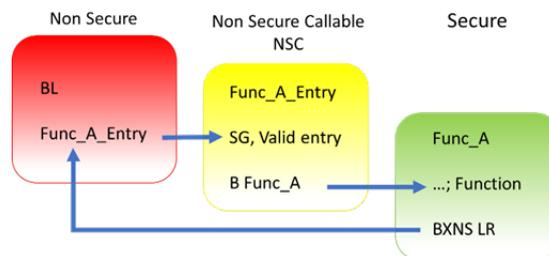
Figure 105: Calling from Non-Secure to Secure Functions
