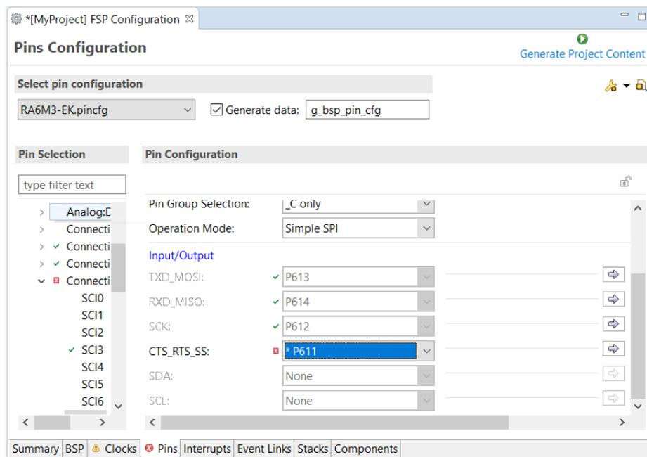
Figure 25: e² studio Pin configurator
