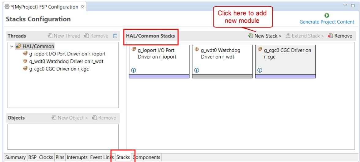
Figure 33: e² studio Project configurator - Adding drivers
