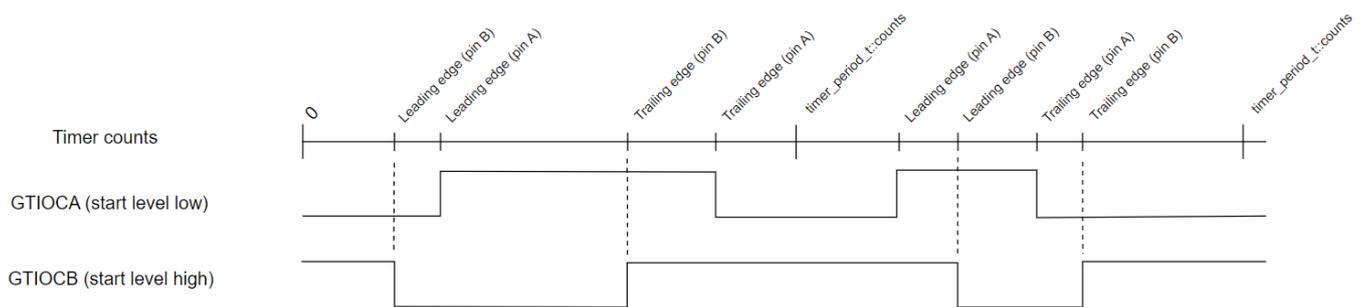
Figure 285: GPT One-Shot Pulse Output (without dead time)
