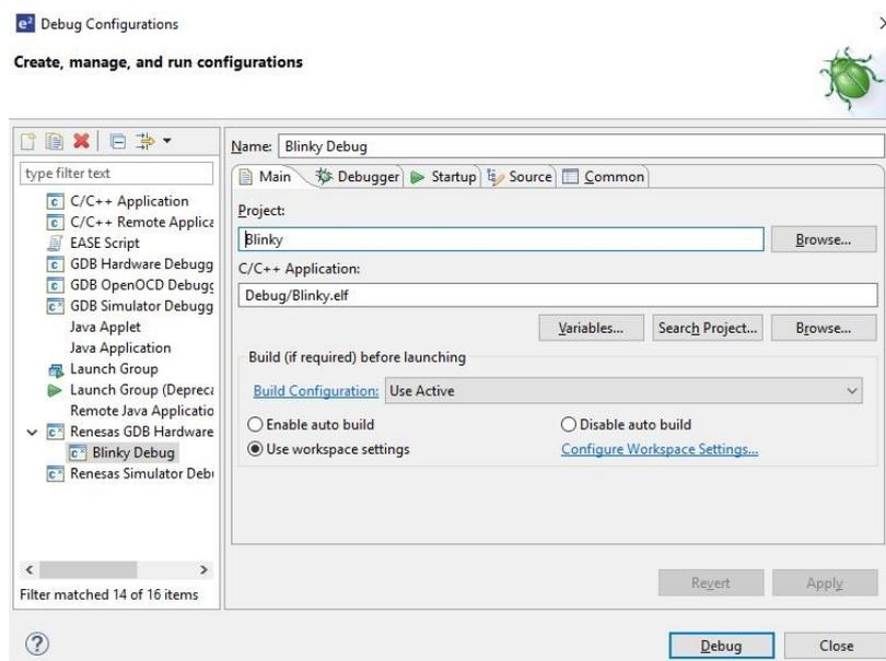
Figure 83: e<sup>2</sup> studio Debugger Configurations window with Blinky project
