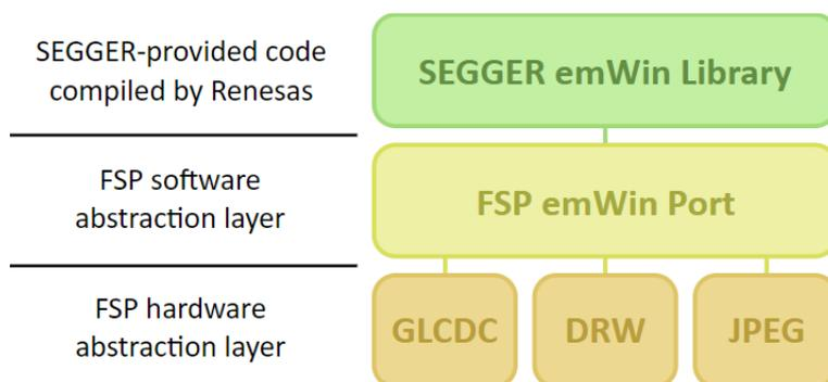
Figure 217: SEGGER emWin FSP Port Block Diagram
