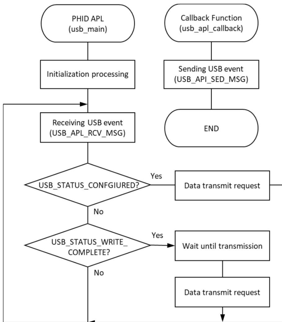
Figure 208: Main Loop processing for RTOS example
