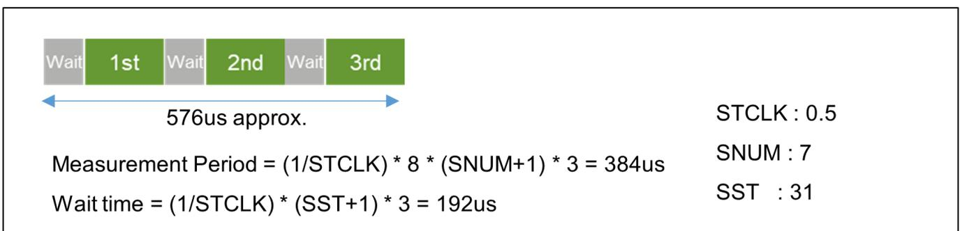
Figure 159: Self-capacitance Measurement Period (CTSU2)
