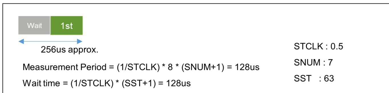
Figure 161: Current Measurement Period
