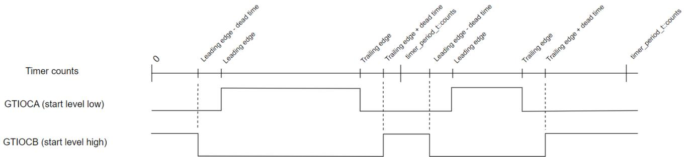
Figure 286: GPT One-Shot Pulse Output (with dead time)
