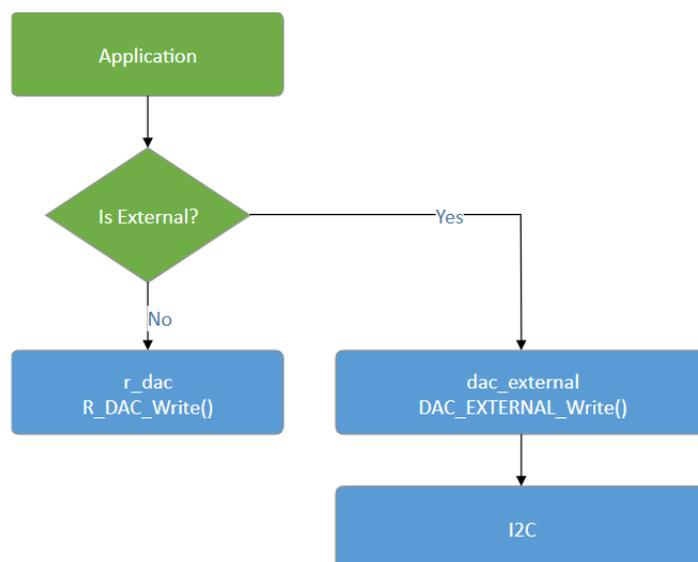
Figure 144: DAC Write with two write modules
