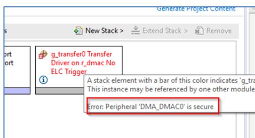
Figure 118: Error Message when Selecting a Secure Channel
