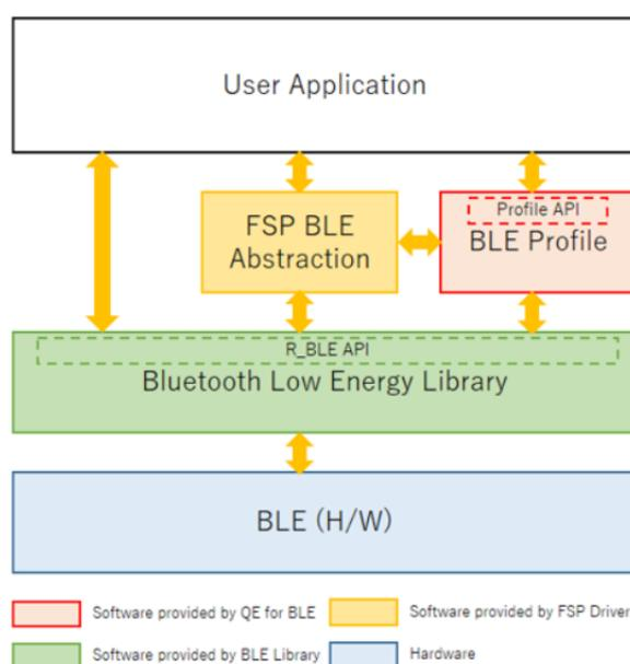
Figure 268: BLE software structure
