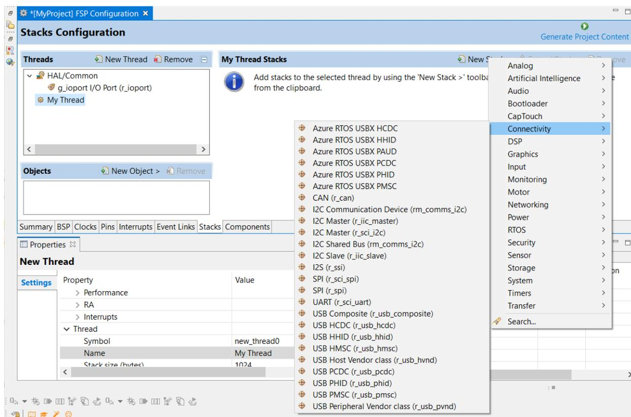
Figure 36: Adding Modules and Drivers to a thread
