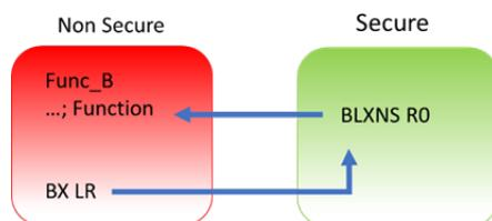
Figure 106: Calling from Secure to Non-Secure Functions
