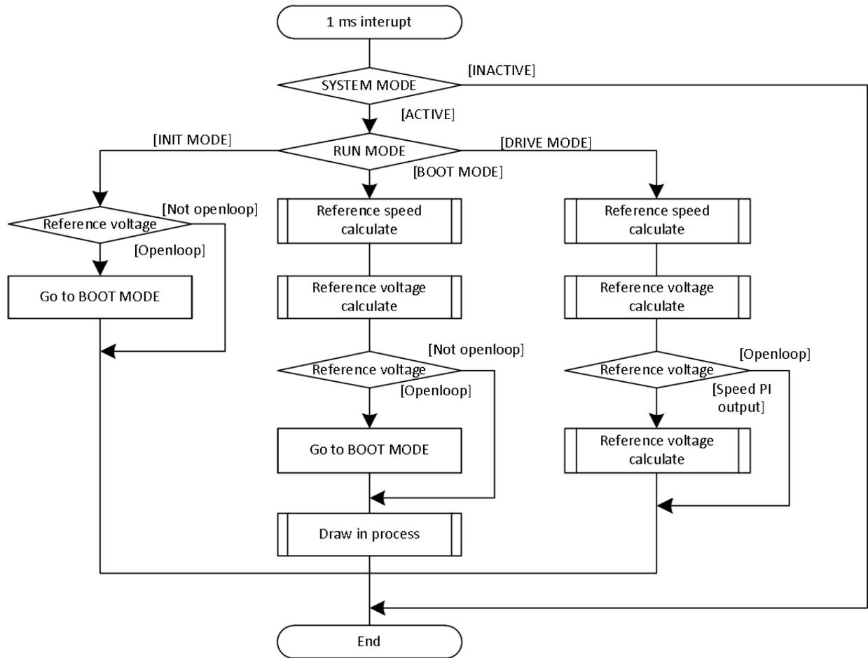
Figure 226: Speed control process of 120-degree sensorless
