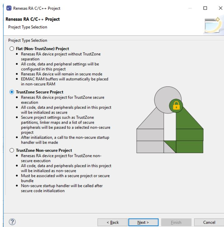
Figure 107: Secure Project (following Arm notation as green)
