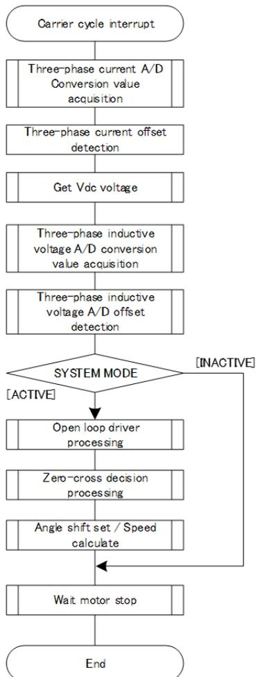
Figure 225: Current control process of 120-degree sensorless
