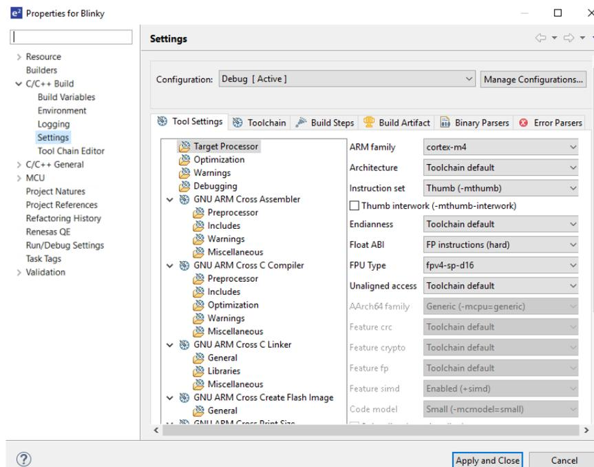
Figure 57: e<sup>2</sup> studio Project toolchain settings for GNU Arm
