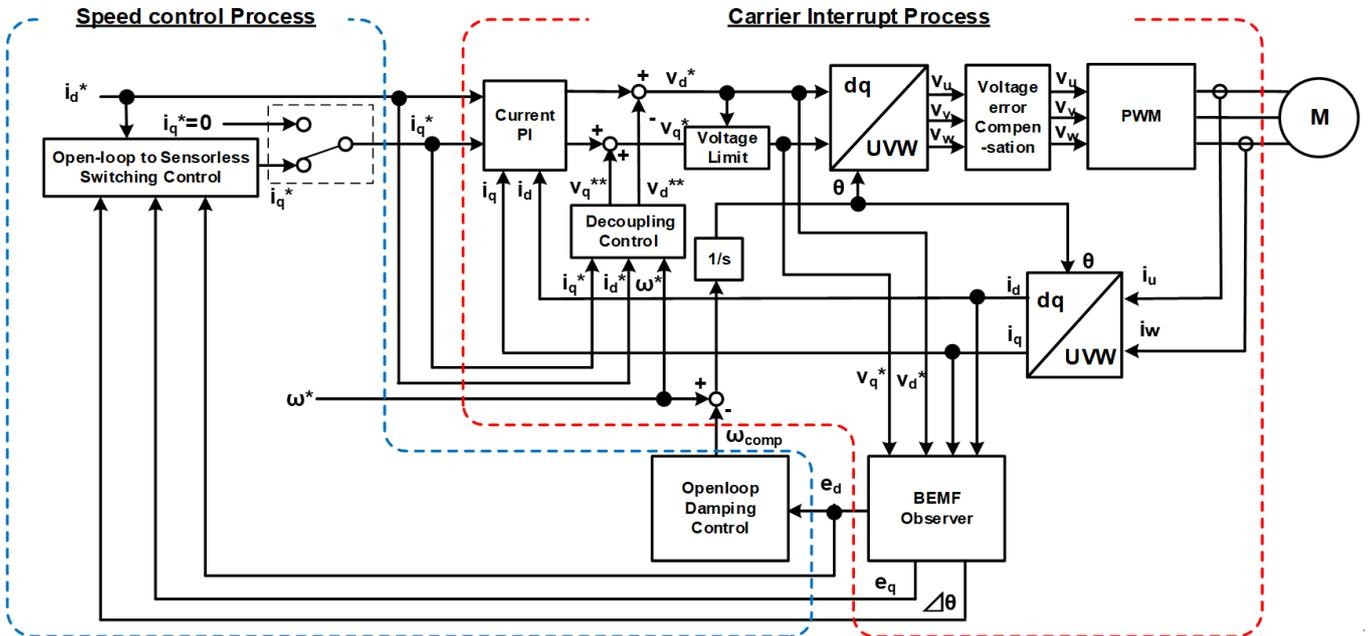
Figure 241: Block diagram of sensorless vector control (open-loop)
