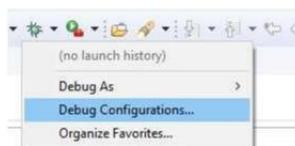
Figure 82: e<sup>2</sup> studio Debugger Configurations selection option
