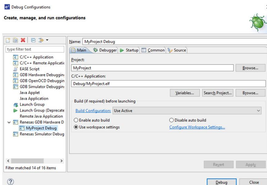
3. Connect the board to your PC via either a standalone Segger J-Link debugger, a Segger J-Link On-Board (included on all RA EKs), or an E2 or E2 Lite and click **Debug**.
