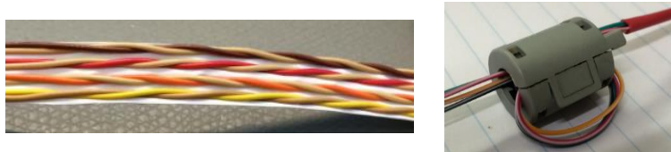
Figure 123: Example of Twisted Pair Cable with 4 Pairs and Ferrite
