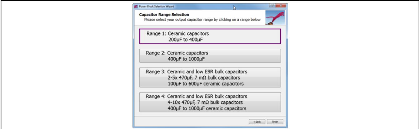
Note: The “Capacitor Range Selection” setting must match the configuration selected by the J106 connector.
