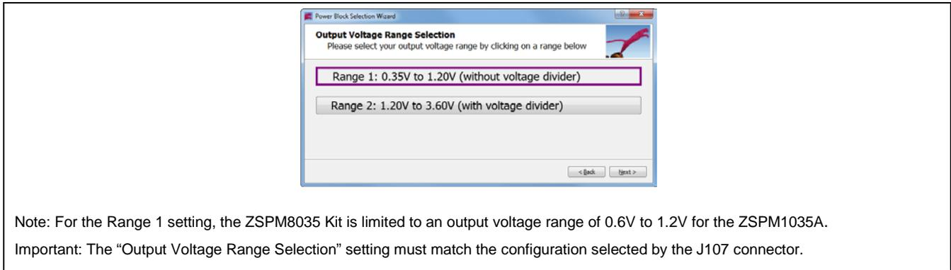
Note: For the Range 1 setting, the ZSPM8035 Kit is limited to an output voltage range of 0.6V to 1.2V for the ZSPM1035A. Important: The "Output Voltage Range Selection" setting must match the configuration selected by the J107 connector.
