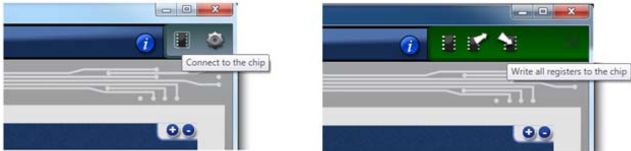
Figure 3. Connecting to the chip: Left: click on the chip symbol to make the connection; Right: A green area appears if I 2 C communication is established.
