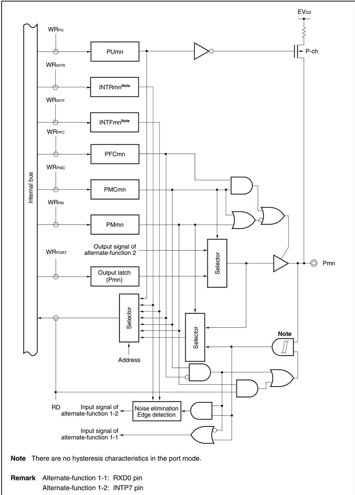
Figure 4-28. Block Diagram of Type E10-SULT
