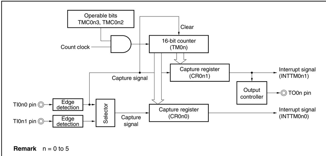
**Figure 8-20. Timing Example of Clear & Start Mode Entered by TI0n0 Pin Valid Edge Input (CR0n0 Register: Capture Register, CR0n1 Register: Capture Register) (1/3)**
