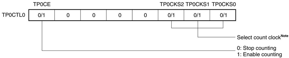
**Note** The setting is invalid when the TP0CTL1.TP0EEE bit = 1.
