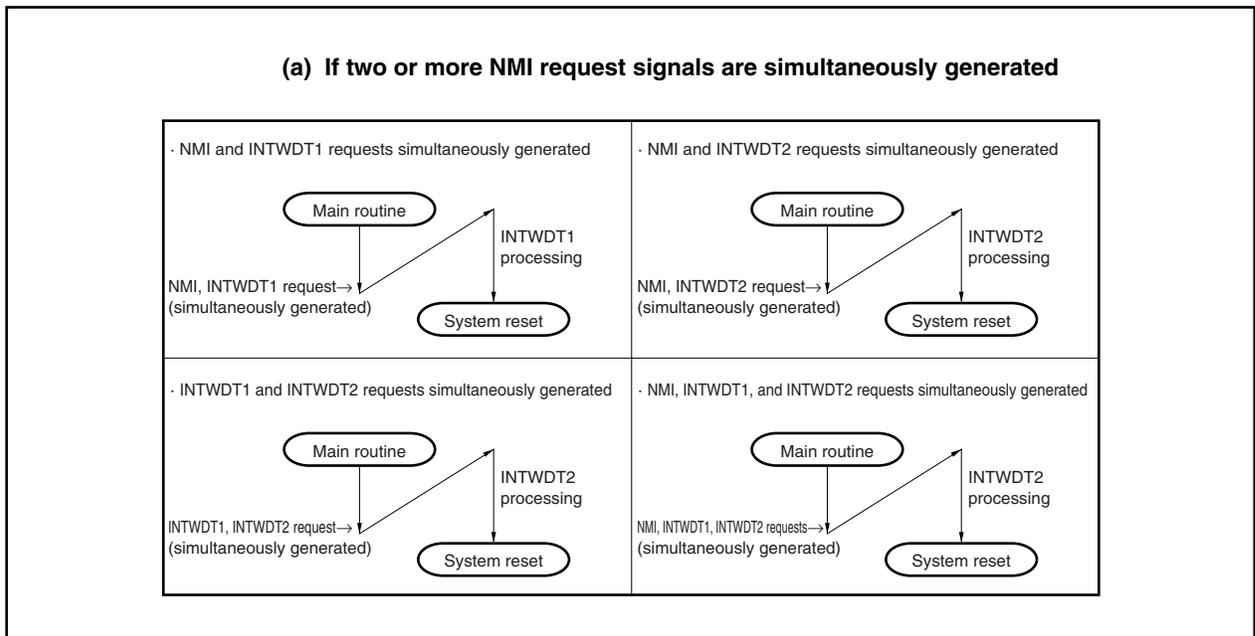
Figure 21-1. Acknowledging Non-Maskable Interrupt Request Signals (2/2)
