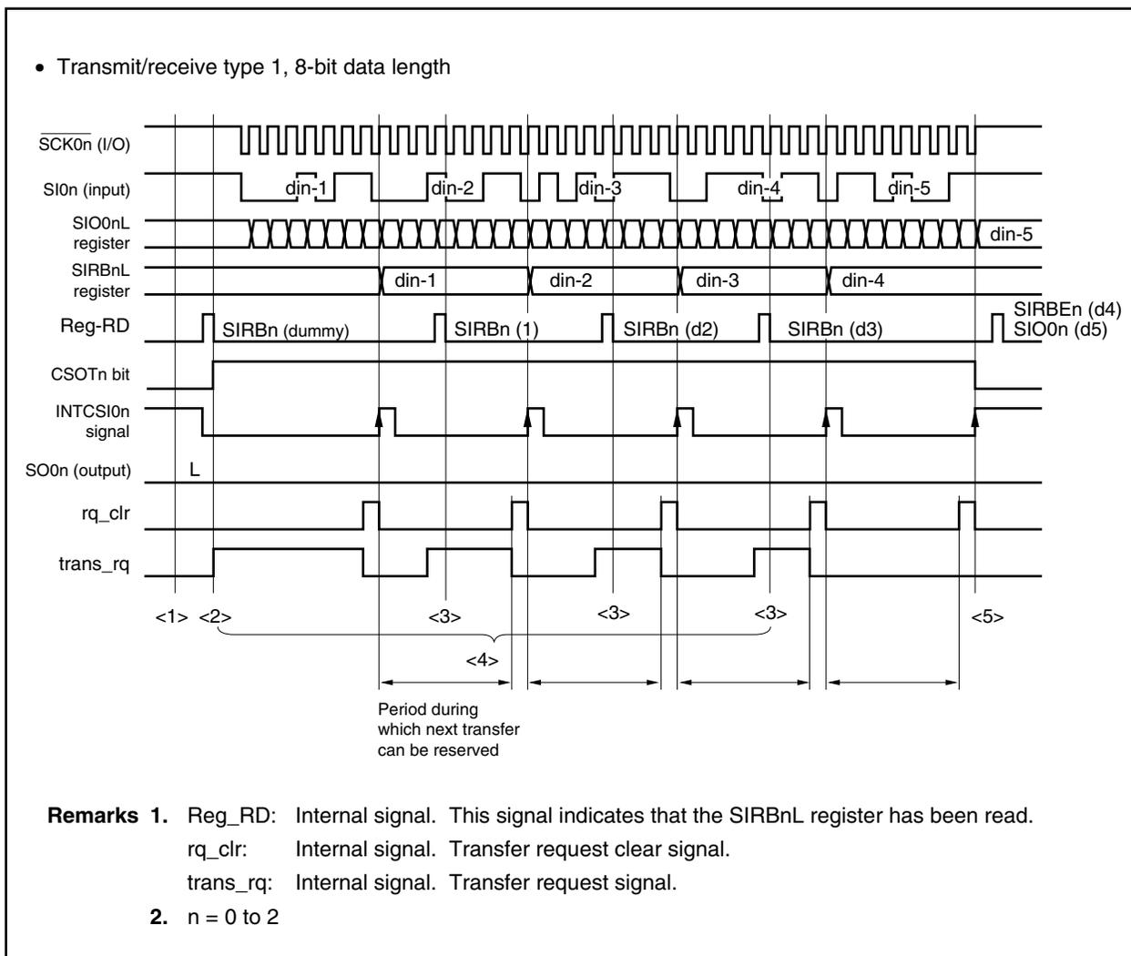
In the case of the continuous transfer mode, two transfer requests are set at the start of the first transfer. Following the INTCSIO0n signal, transfer is continued if the SIRBnL register can be read within the next transfer reservation period. If the SIRBnL register cannot be read, transfer ends and the SIRBnL register does not receive the new value of the SIO0nL register.
