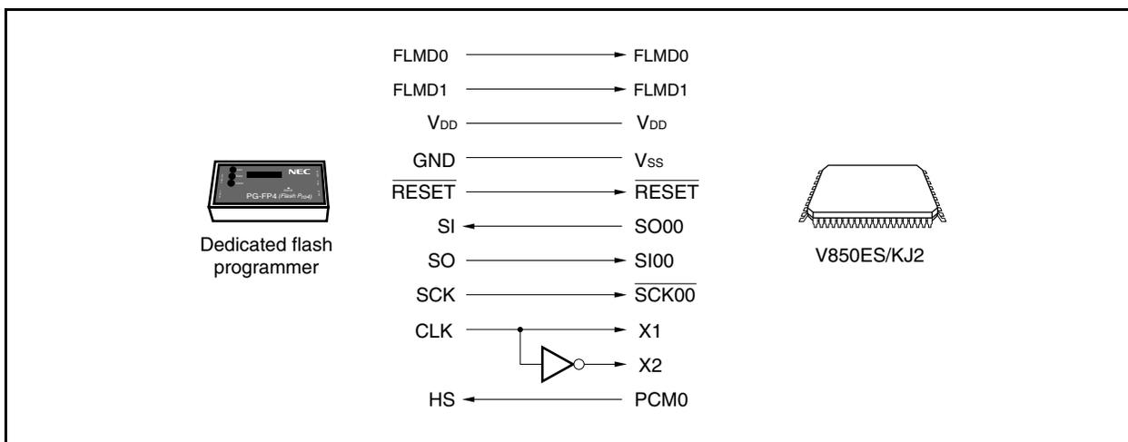
The dedicated flash programmer outputs the transfer clock, and the V850ES/KJ2 operates as a slave.
