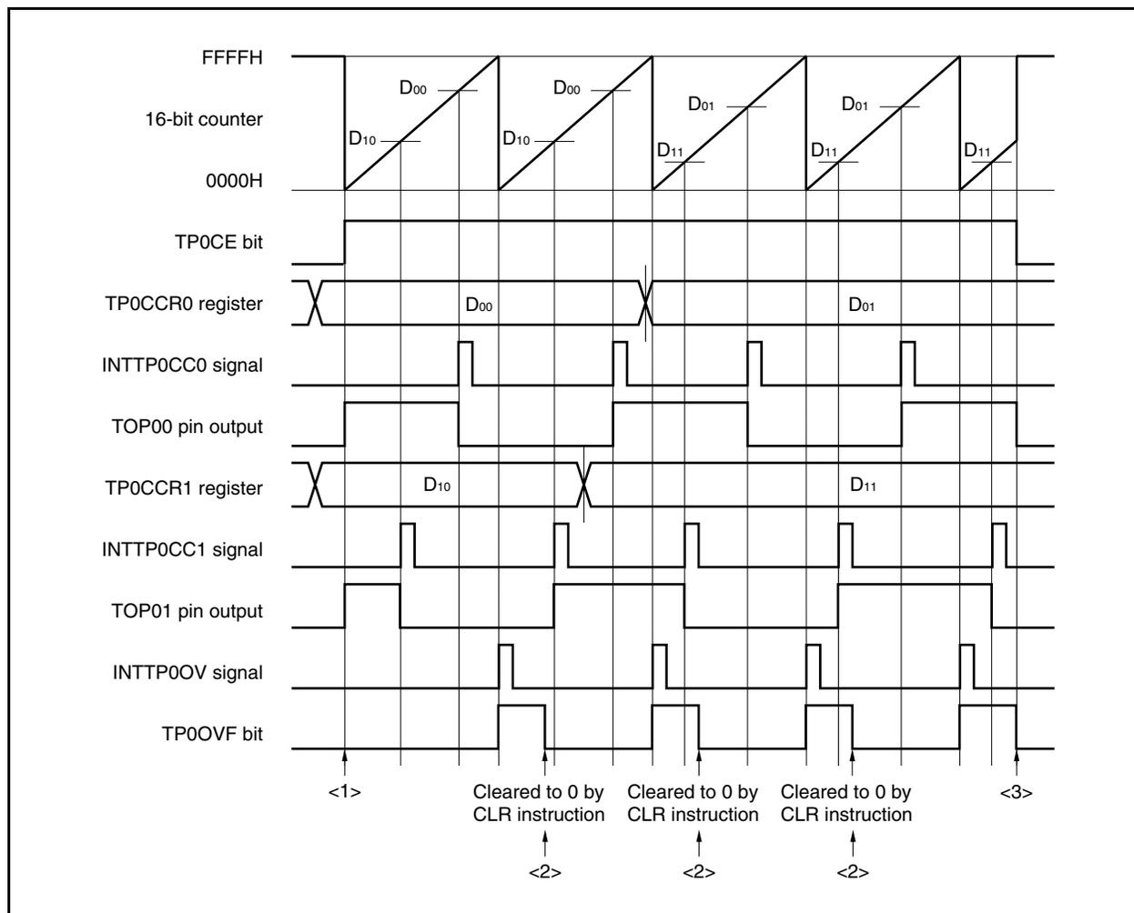
Figure 7-32. Software Processing Flow in Free-Running Timer Mode (Compare Function) (2/2)
