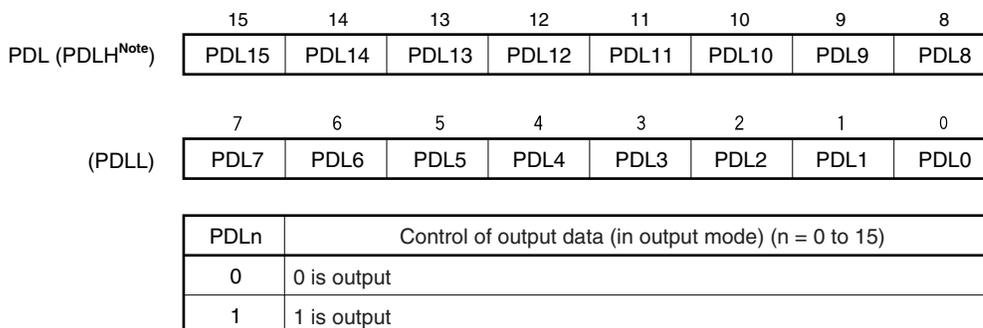
**Note** When reading from or writing to bits 8 to 15 of the PDL register in 8-bit or 1-bit units, specify these bits as bits 0 to 7 of the PDLH register.
