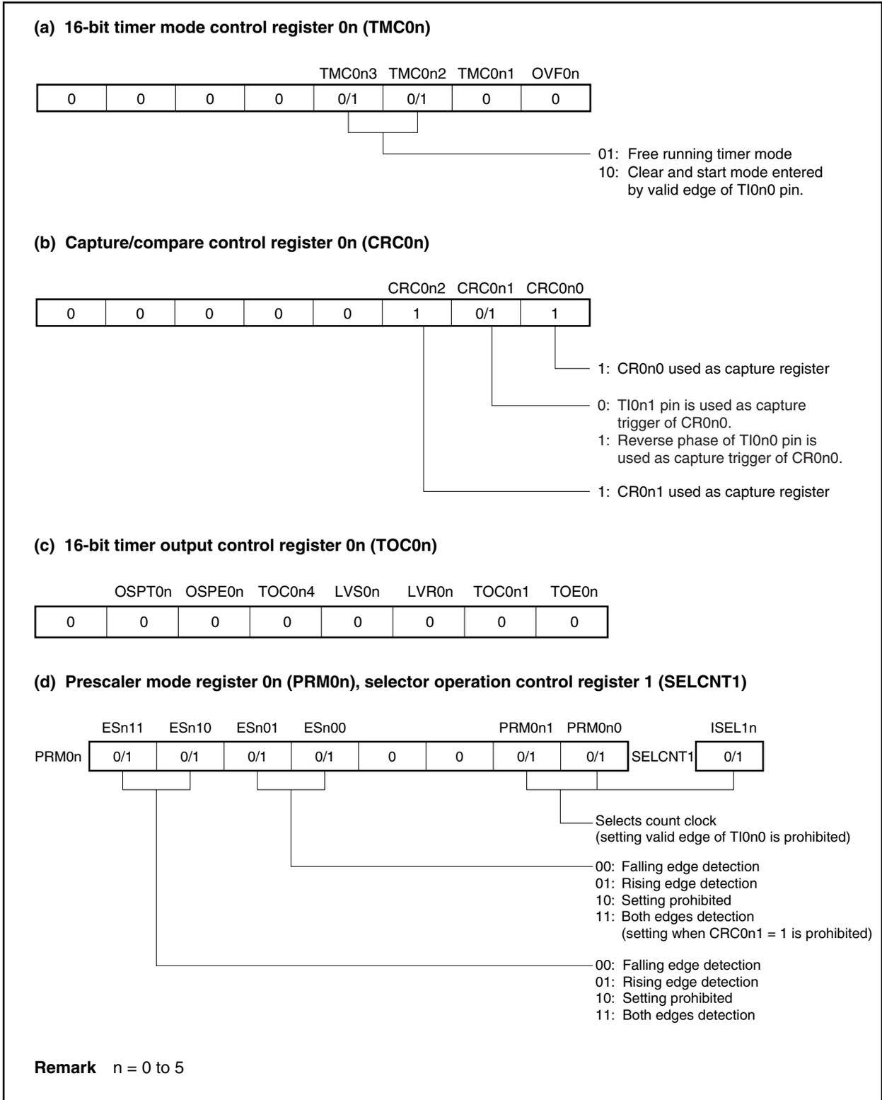
Figure 8-42. Example of Register Settings for Pulse Width Measurement (2/2)
