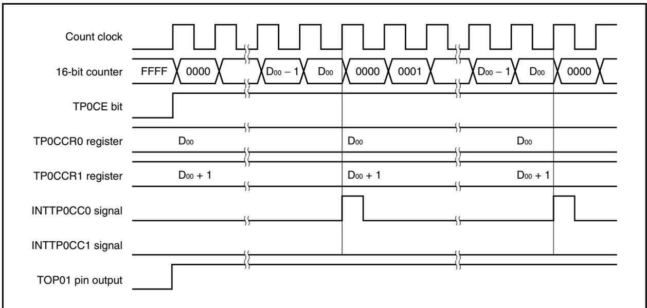
**(c) Generation timing of compare match interrupt request signal (INTTP0CC1)**
