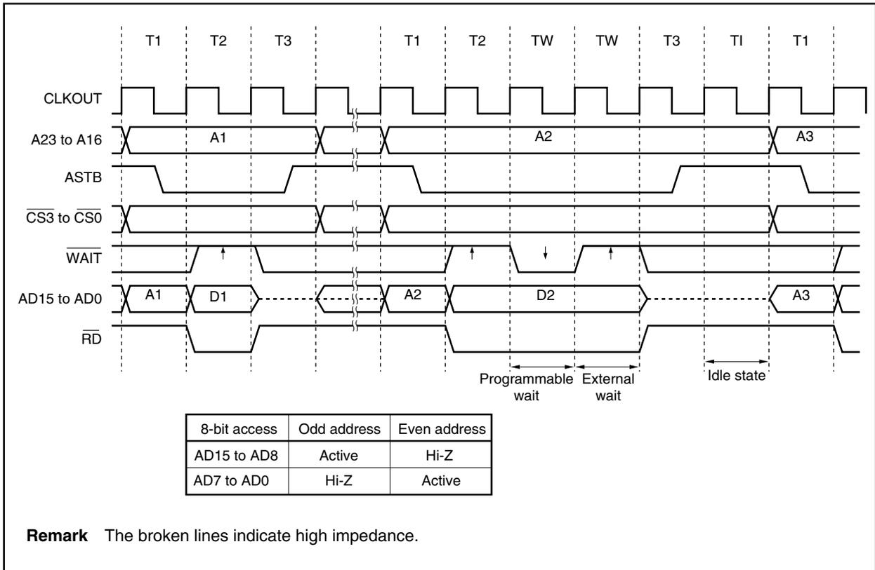
Figure 5-5. Multiplex Bus Read Timing (Bus Size: 8 Bits)
