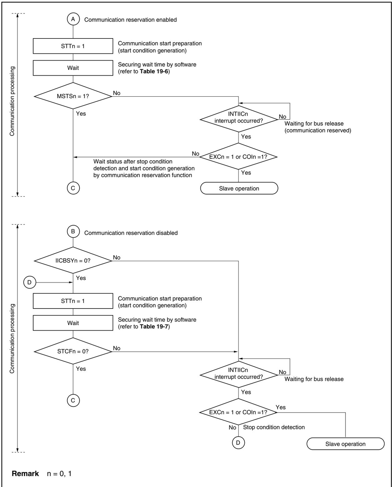
Figure 19-17. Master Operation in Multimaster System (3/3)
