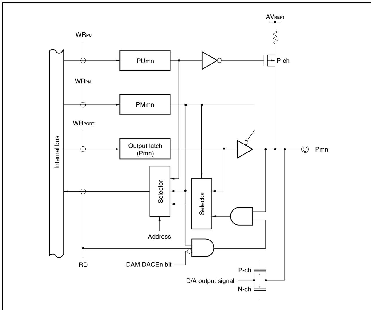
Figure 4-6. Block Diagram of Type D0-U
