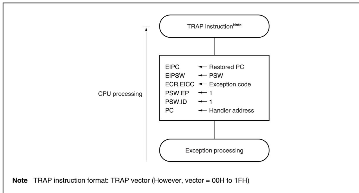
The handler address is determined by the operand (vector) of the TRAP instruction. If the vector is 00H to 1FH, the handler address is 00000040H, and if the vector is 10H to 1FH, the handler address is 00000050H.
