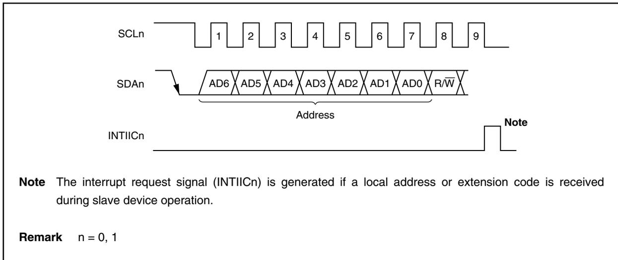
The slave address and the eighth bit, which specifies the transfer direction as described in **19.6.3 Transfer direction specification** below, are together written to the IIC<sub>n</sub> register and are then output. Received addresses are written to the IIC<sub>n</sub> register.
