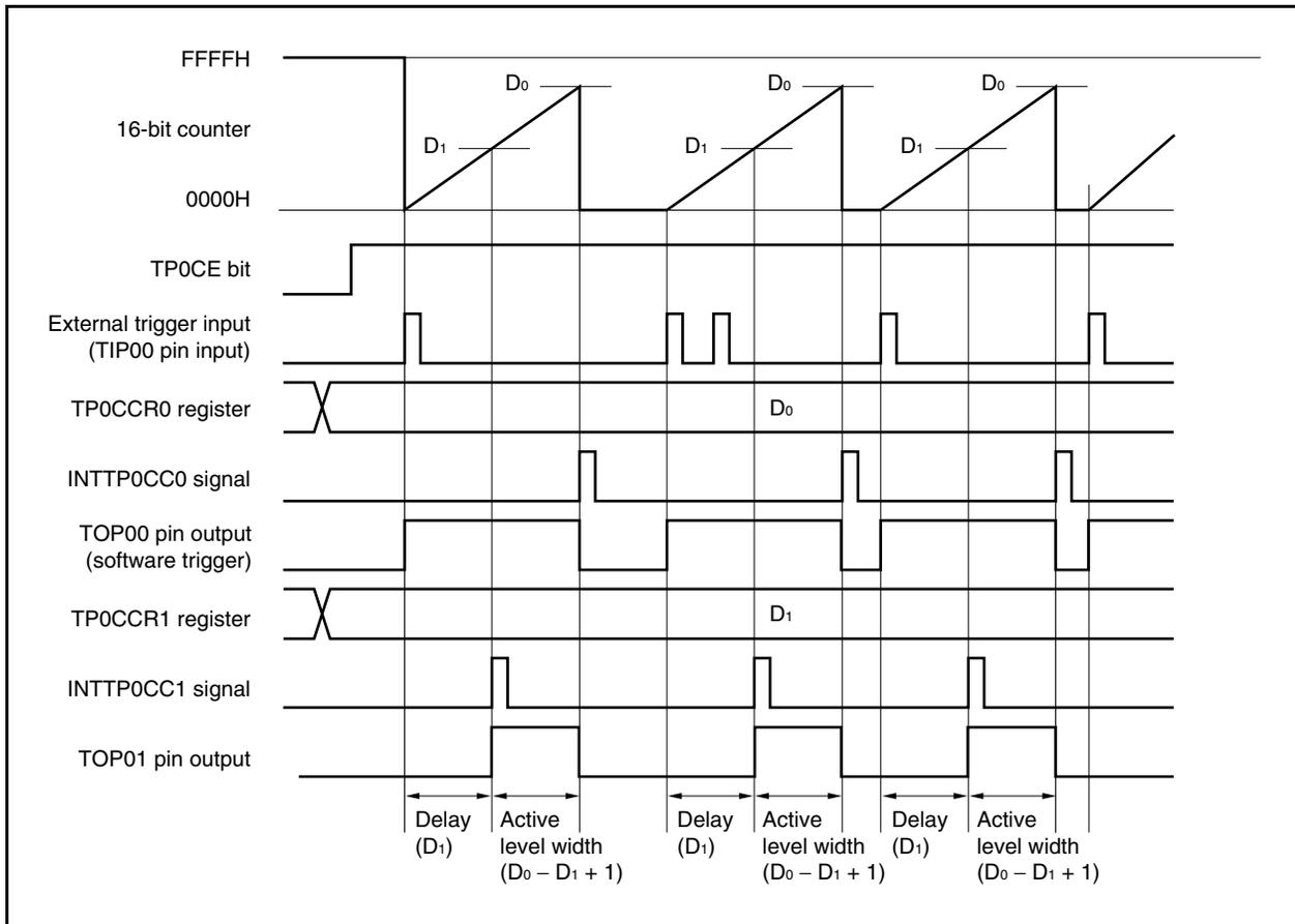
When the TP0CE bit is set to 1, 16-bit timer/event counter P waits for a trigger. When the trigger is generated, the 16-bit counter is cleared from FFFFH to 0000H, starts counting, and outputs a one-shot pulse from the TOP01 pin. After the one-shot pulse is output, the 16-bit counter is set to FFFFH, stops counting, and waits for a trigger. If a trigger is generated again while the one-shot pulse is being output, it is ignored.
