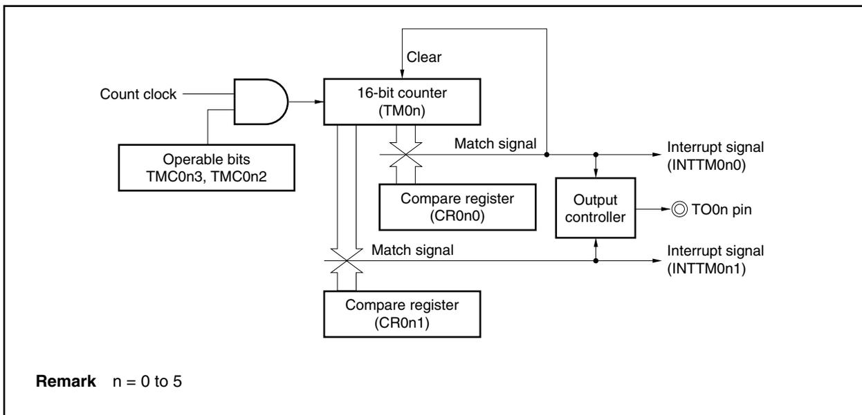
Figure 8-32. Example of Register Settings for PPG Output Operation
