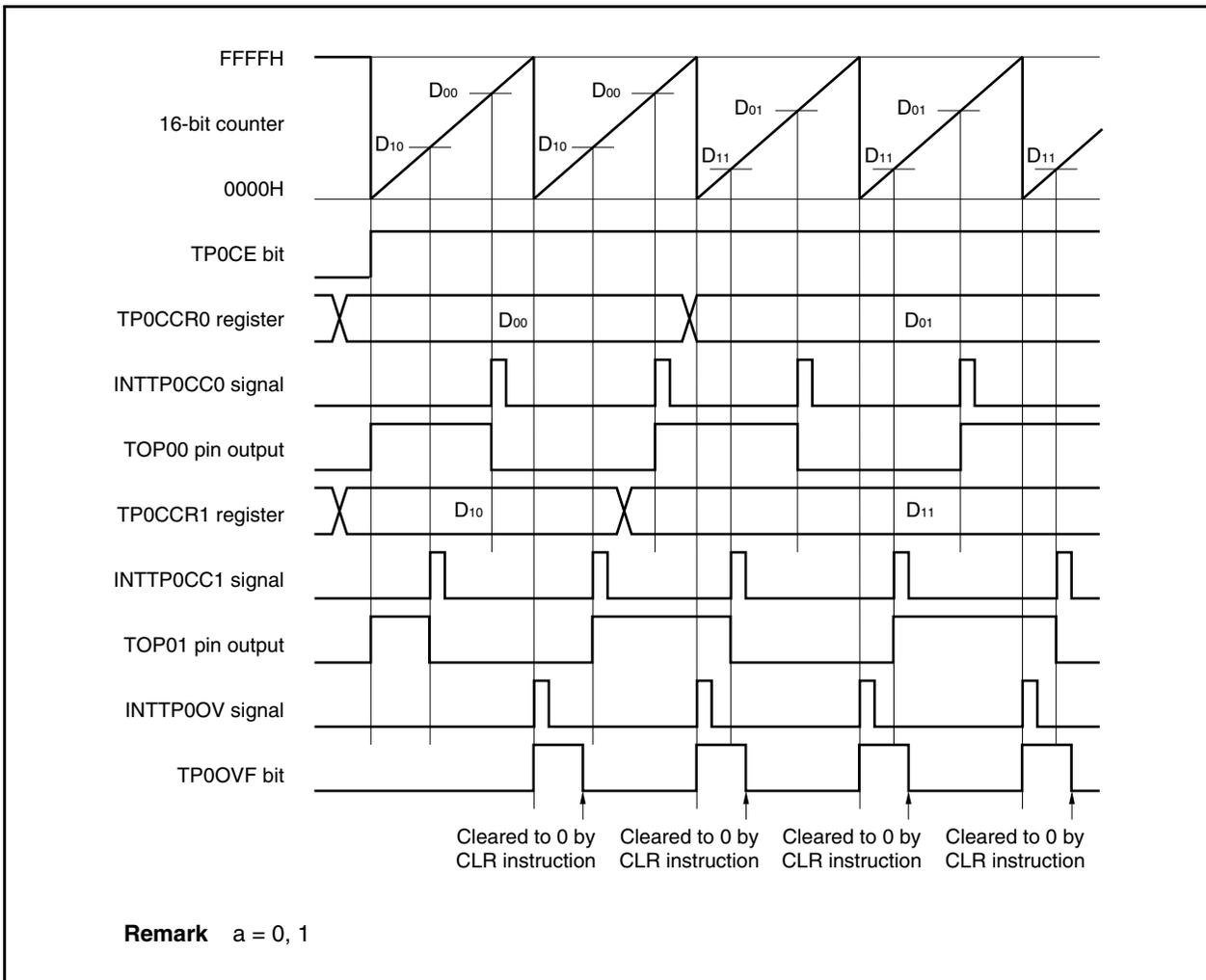
When the TP0CE bit is set to 1, the 16-bit counter starts counting. When the valid edge input to the TIP0a pin is detected, the count value of the 16-bit counter is stored in the TP0CCR0 register, and a capture interrupt request signal (INTTP0CCa) is generated.
