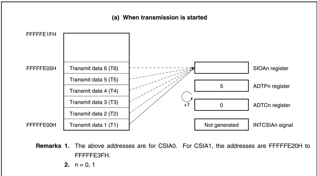
**Figure 18-13. Buffer RAM Operation in 6-Byte Transmission
