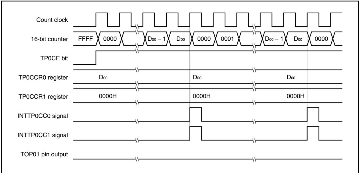
To output a 100% waveform, set a value of (set value of TP0CCR0 register + 1) to the TP0CCR1 register. If the set value of the TP0CCR0 register is FFFFH, 100% output cannot be produced.
