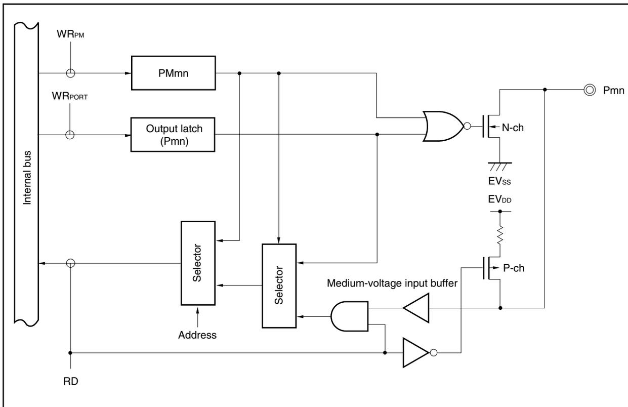
Figure 4-4. Block Diagram of Type C-U
