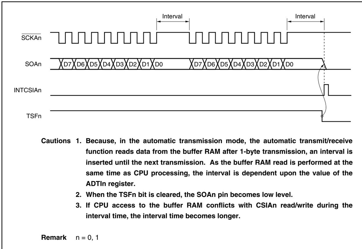
Figure 18-9. Automatic Transmission Mode Flowchart
