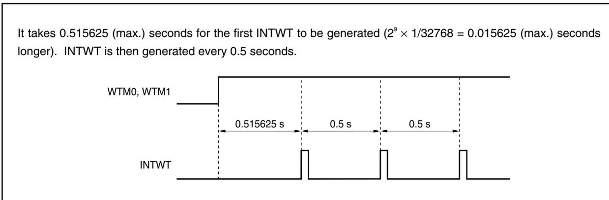
**(2) When watch timer and interval timer BRG operate simultaneously**
