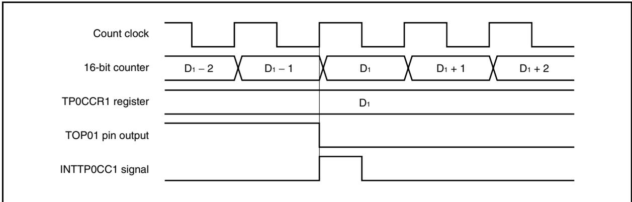
Usually, the INTTP0CC1 signal is generated when the 16-bit counter counts up next time after its count value matches the value of the TP0CCR1 register.
