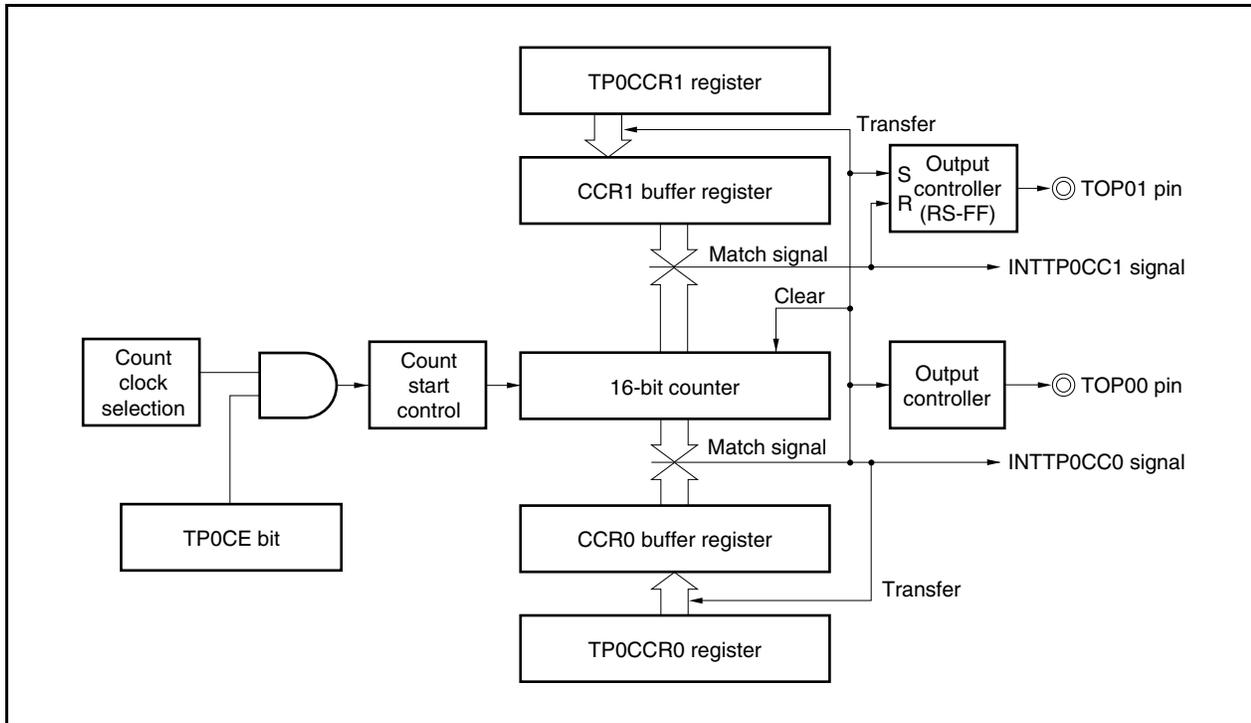
Figure 7-25. Basic Timing in PWM Output Mode
