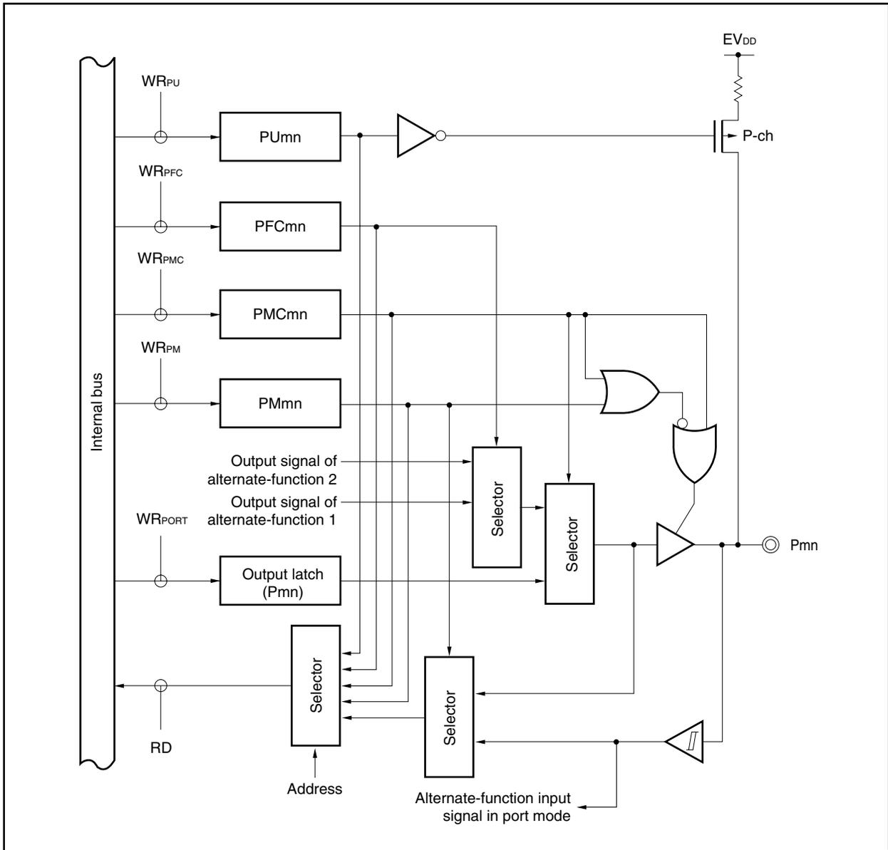
Figure 4-17. Block Diagram of Type E00-SUTZ
