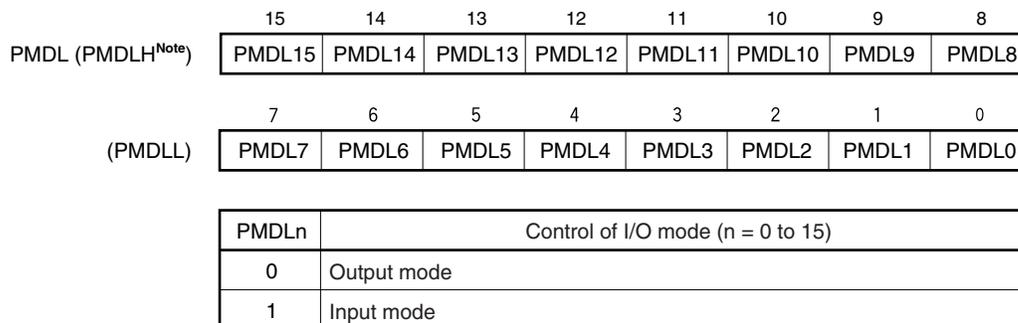
**Note** When reading from or writing to bits 8 to 15 of the PMDL register in 8-bit or 1-bit units, specify these bits as bits 0 to 7 of the PMDLH register.
