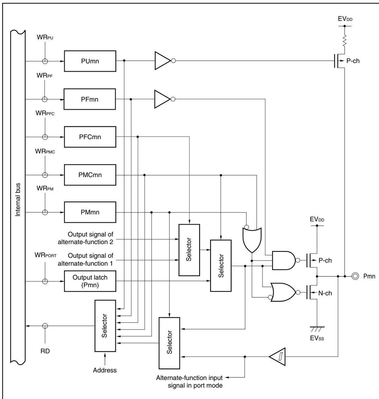
Figure 4-16. Block Diagram of Type E00-SUT
