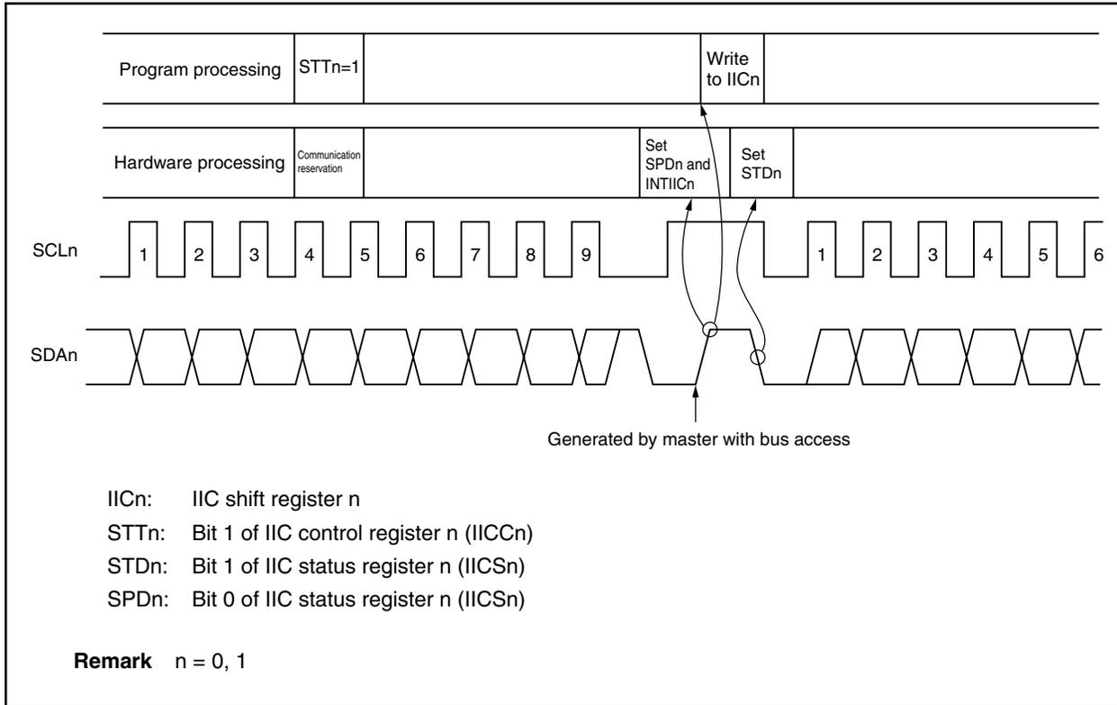
Communication reservations are accepted via the following timing. After the IICSn.STDn bit is set to 1, a communication reservation can be made by setting the IICn.STTn bit to 1 before a stop condition is detected (n = 0, 1).
