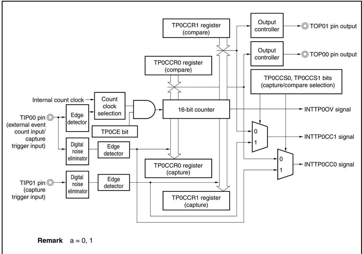
When the TP0CE bit is set to 1, 16-bit timer/event counter P starts counting, and the output signals of the TOP00 and TOP01 pins are inverted. When the count value of the 16-bit counter later matches the set value of the TP0CCRa register, a compare match interrupt request signal (INTTP0CCa) is generated, and the output signal of the TOP0a pin is inverted.
