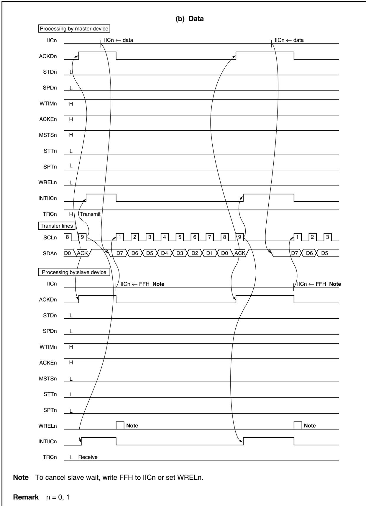
**Figure 19-21. Example of Master to Slave Communication
