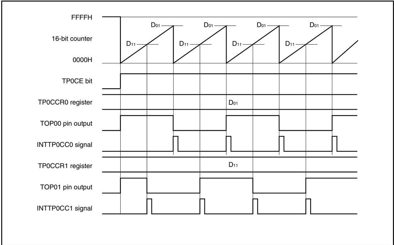
If the set value of the TP0CCR1 register is greater than the set value of the TP0CCR0 register, the count value of the 16-bit counter does not match the value of the TP0CCR1 register. Consequently, the INTTP0CC1 signal is not generated, nor is the output of the TOP01 pin changed.
