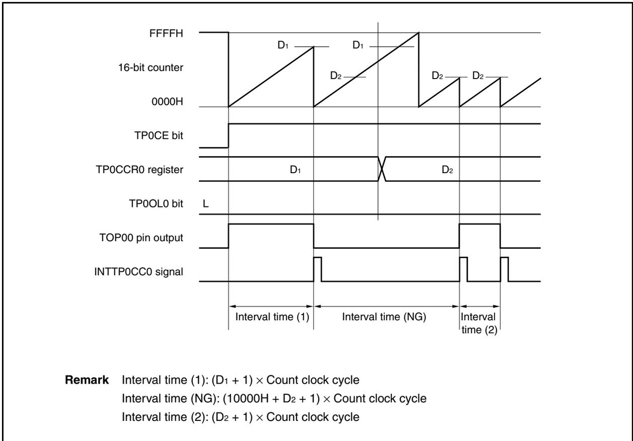
If the value of the TP0CCR0 register is changed from  $D_1$  to  $D_2$  while the count value is greater than  $D_2$  but less than  $D_1$ , the count value is transferred to the CCR0 buffer register as soon as the TP0CCR0 register has been rewritten. Consequently, the value of the 16-bit counter that is compared is  $D_2$ .
