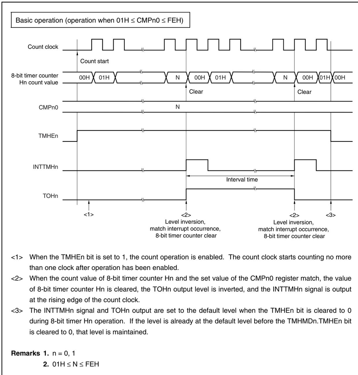
Figure 10-3. Timing of Interval Timer/Square Wave Output Operation (2/2)
