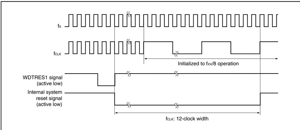
Figure 24-5. Timing of Reset Operation by Watchdog Timer 2
