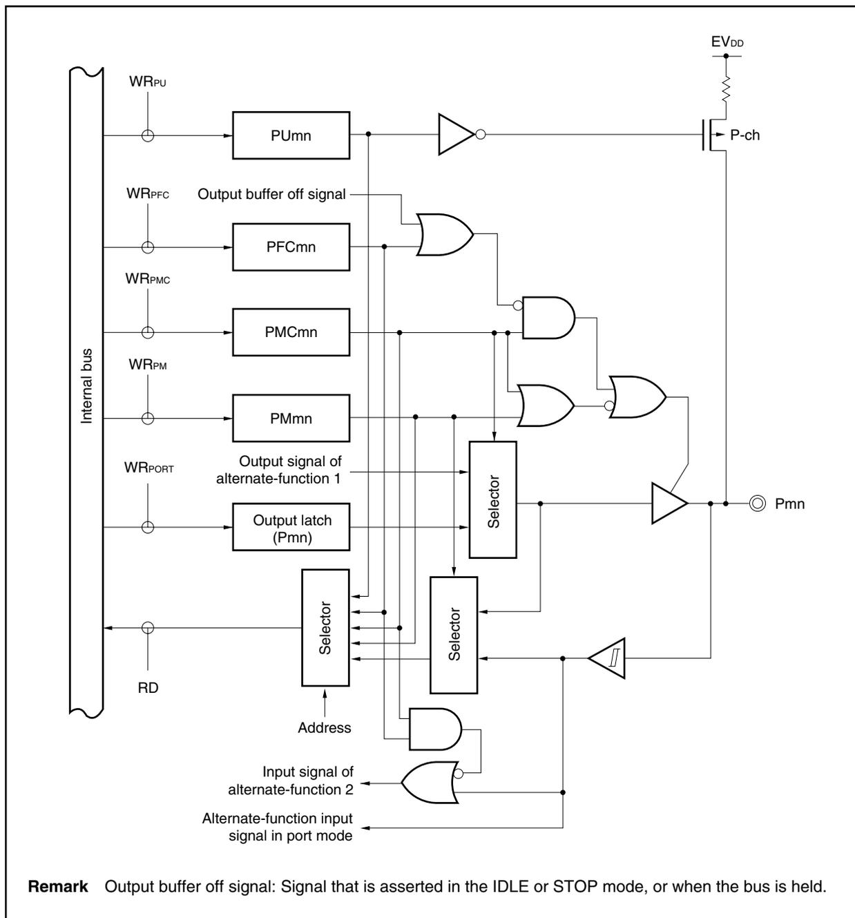
**Remark** Output buffer off signal: Signal that is asserted in the IDLE or STOP mode, or when the bus is held.
