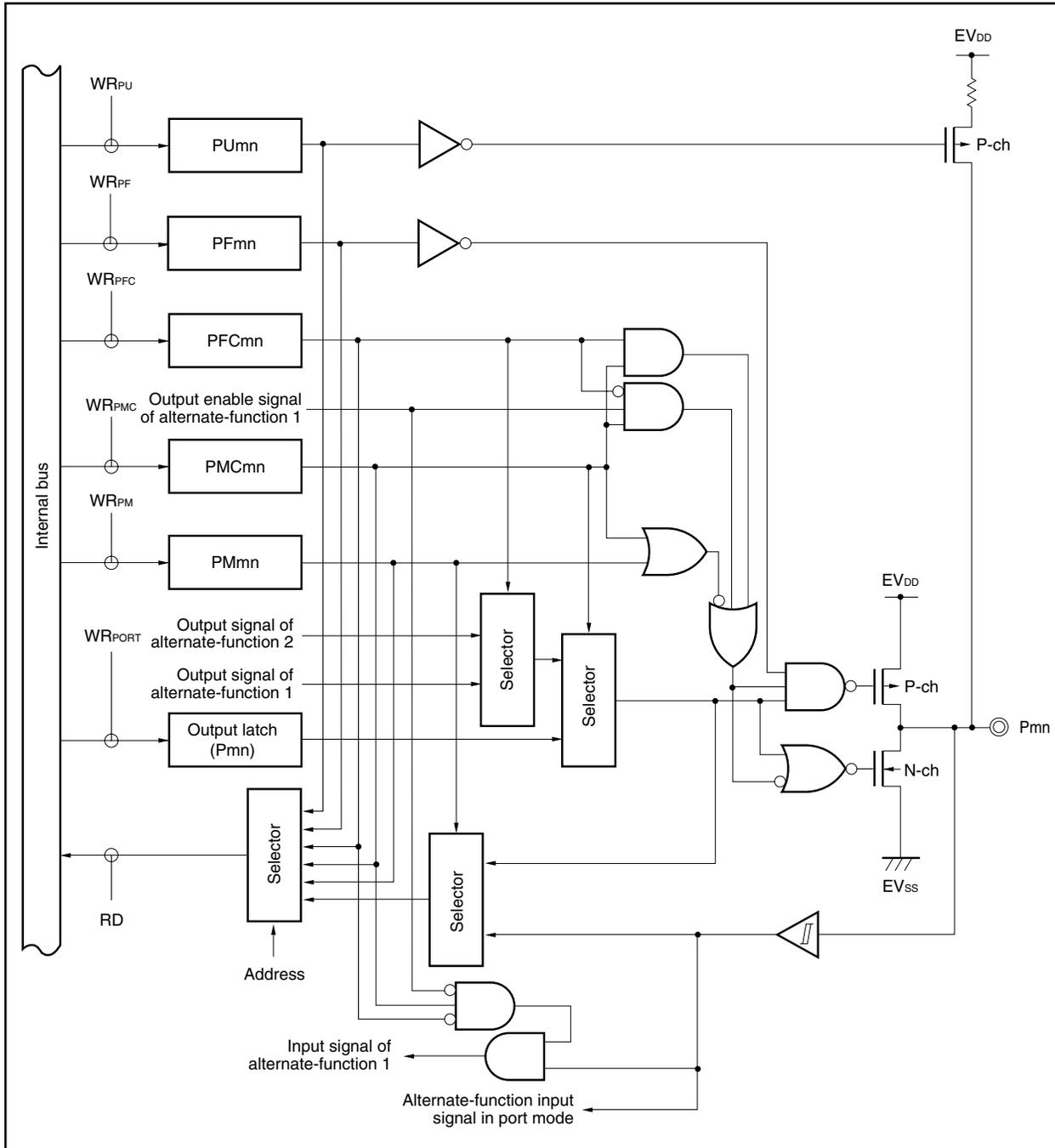
Figure 4-32. Block Diagram of Type G1010-SUL
