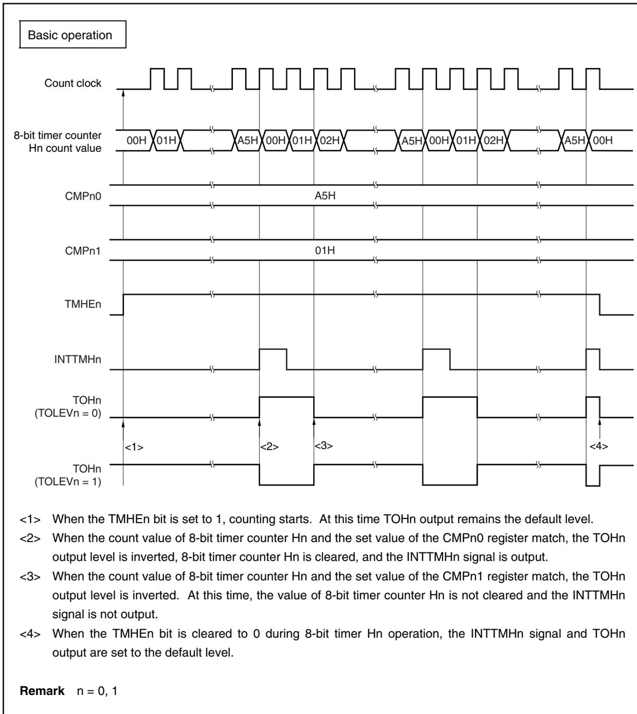
Figure 10-5. Operation Timing in PWM Output Mode (2/4)
