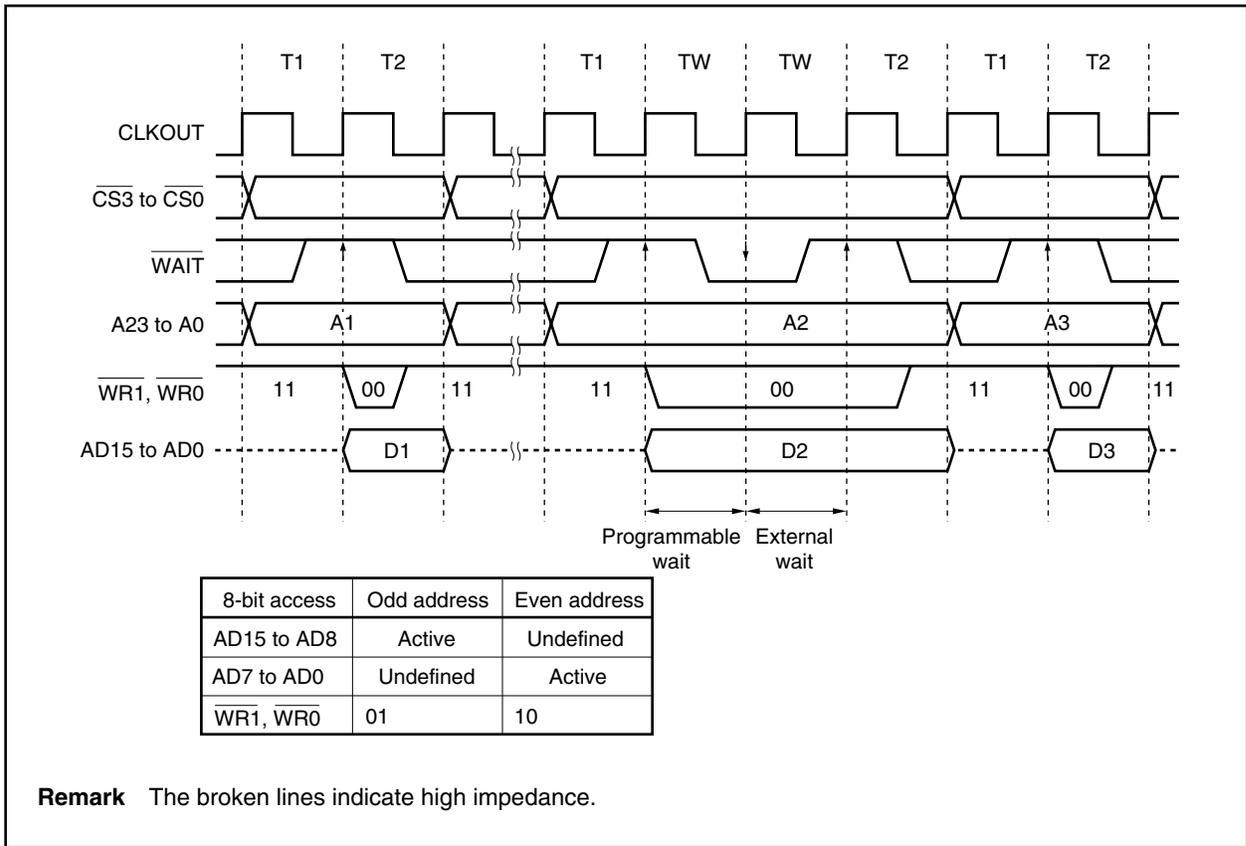
Figure 5-12. Separate Bus Write Timing (Bus Size: 8 Bits)
