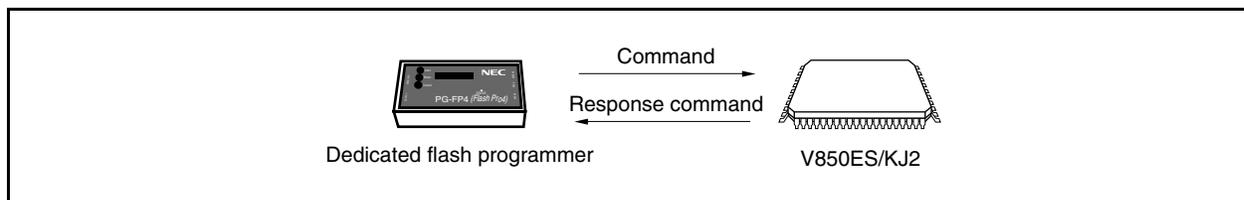
The following shows the commands for flash memory control in the V850ES/KJ2. All of these commands are issued from the dedicated flash programmer, and the V850ES/KJ2 performs the processing corresponding to the commands.
