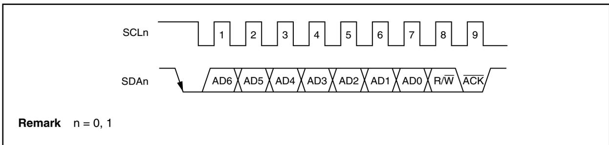
When the local address is received,  $\overline{\text{ACK}}$  is automatically generated regardless of the value of the ACKEn bit. No  $\overline{\text{ACK}}$  is generated if the received address is not a local address (NACK).
