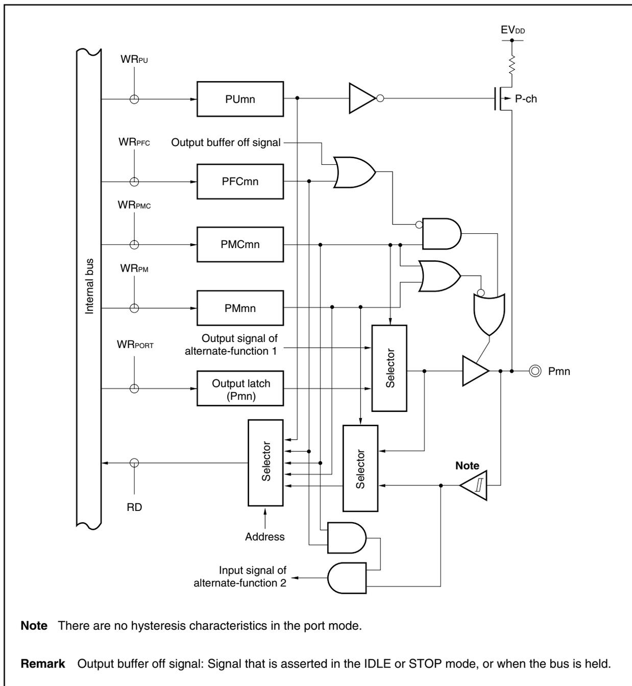
Figure 4-24. Block Diagram of Type E02-SUFH
