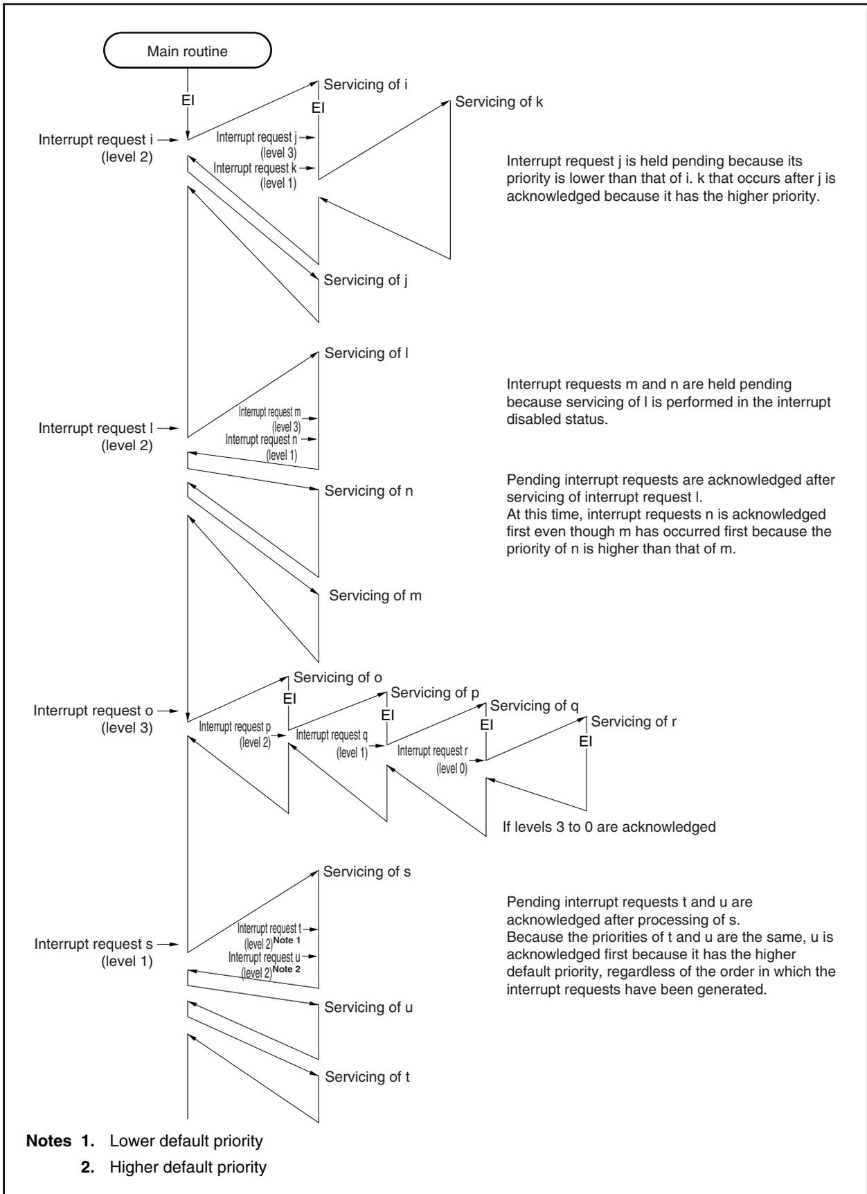
Figure 21-7. Example of Servicing Simultaneously Generated Interrupt Request Signals
