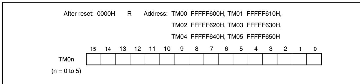
The count value of the TM0n register can be read by reading the TM0n register when the values of the TMC0n.TMC0n3 and TMC0n.TMC0n2 bits are other than 00. The value of the TM0n register is 0000H if it is read when the TMC0n3 and TMC0n2 bits are 00.
