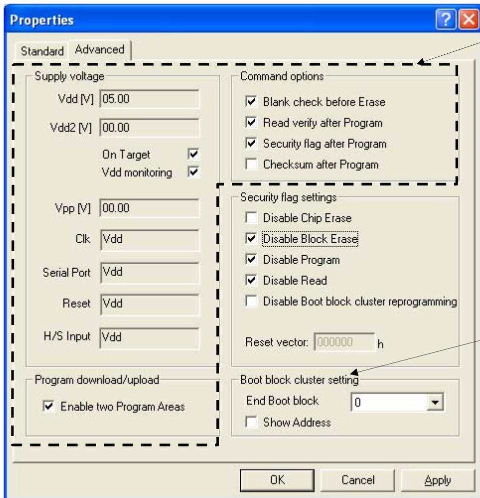
**Notes 1.** Set "Supply voltage", "Program download/upload", and "Command options" in broken lines in accordance with the use conditions.
