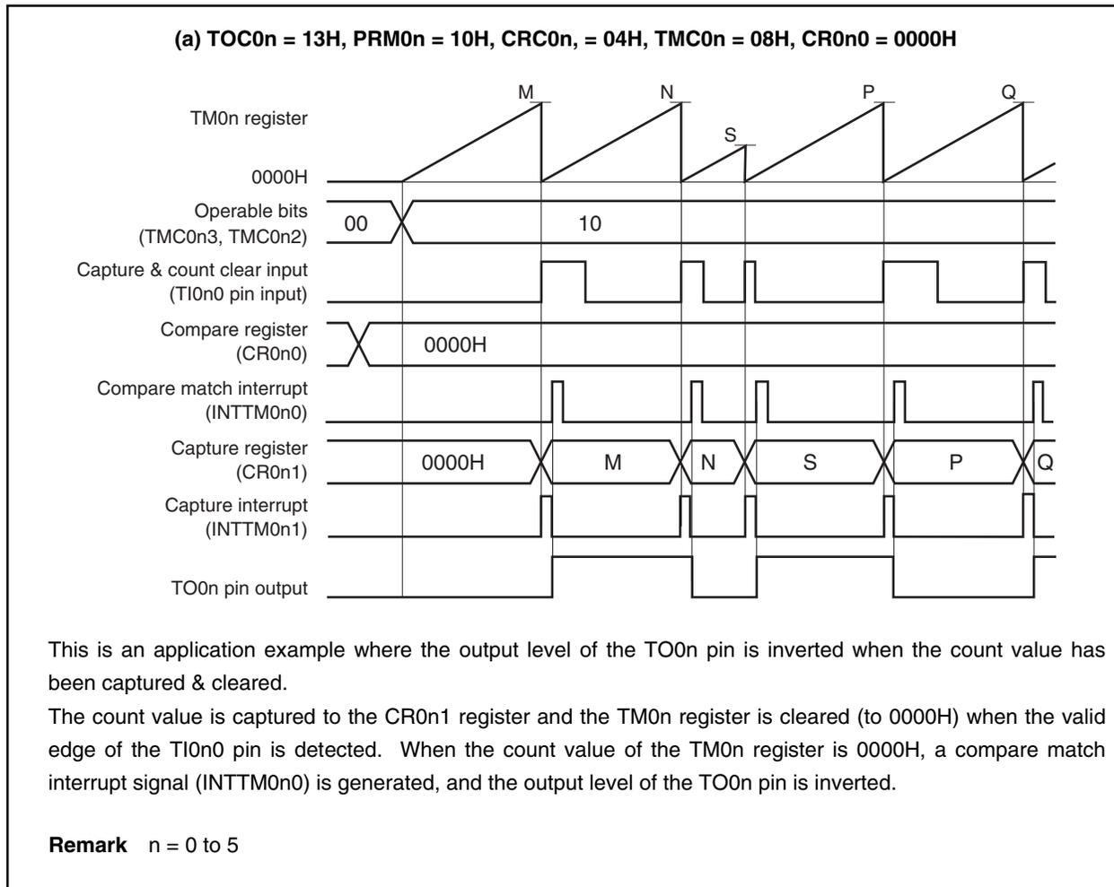
**Figure 8-16. Timing Example of Clear & Start Mode Entered by TIO<sub>n</sub> Pin Valid Edge Input
