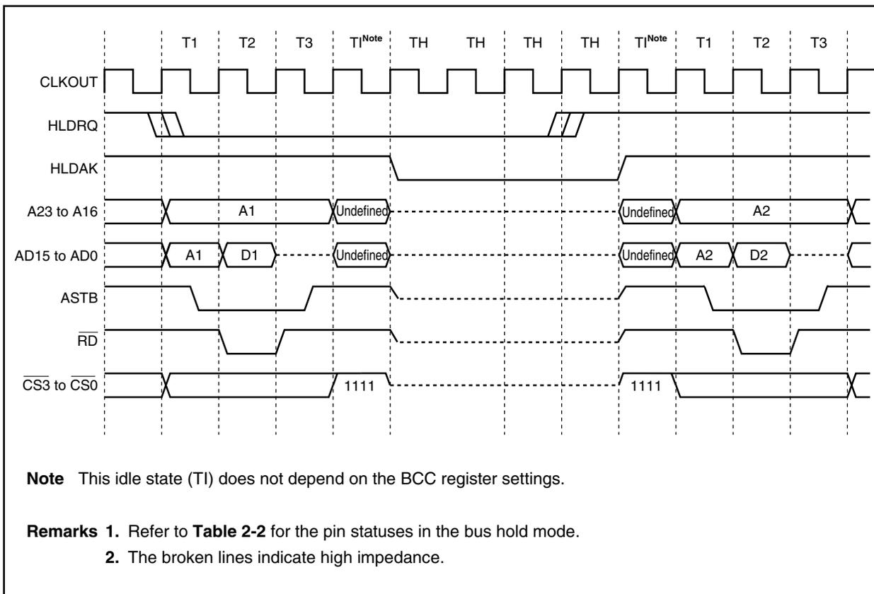
Figure 5-9. Separate Bus Read Timing (Bus Size: 16 Bits, 16-Bit Access)
