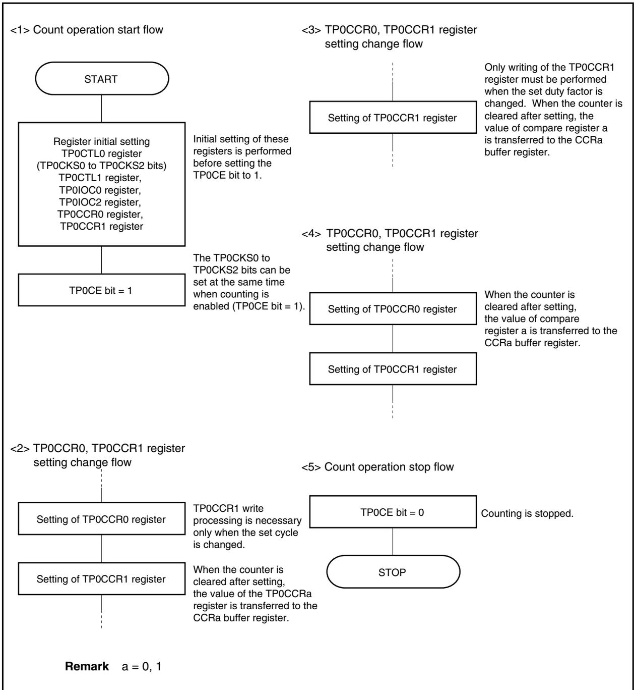
**(2) PWM output mode operation timing****(a) Changing pulse width during operation**
