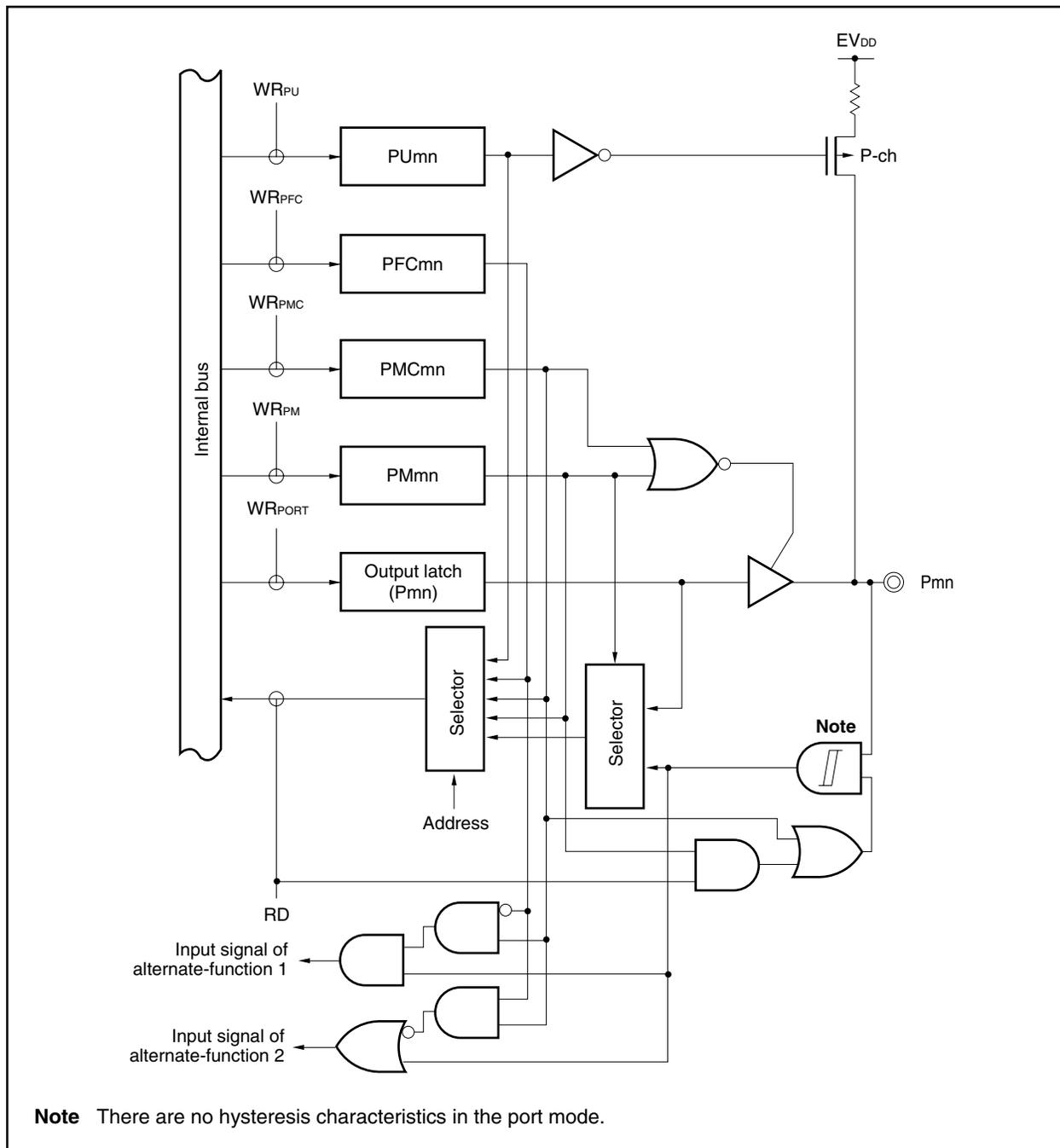
Figure 4-30. Block Diagram of Type E12-SUFHH
