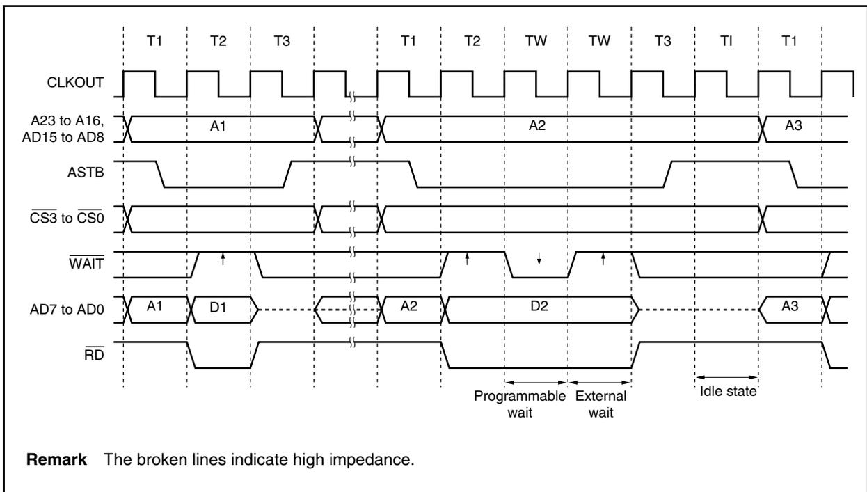
Figure 5-6. Multiplex Bus Write Timing (Bus Size: 16 Bits, 16-Bit Access)
