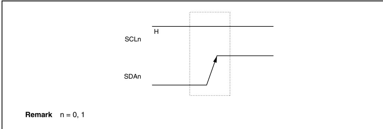
A stop condition is generated when the IICn.SPTn bit is set to 1. When the stop condition is detected, the IICn.SPEn bit is set to 1 and the interrupt request signal (INTIICn) is generated when the IICn.SPIEn bit is set to 1.
