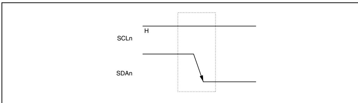
A start condition is generated when the IICn.STTn bit is set to 1 after a stop condition has been detected (IICn.SPdn bit = 1). When a start condition is detected, IICn.STDn bit is set to 1.
