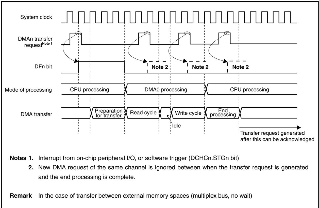
Figure 20-4. Period in Which DMA Transfer Request Is Ignored (2)
