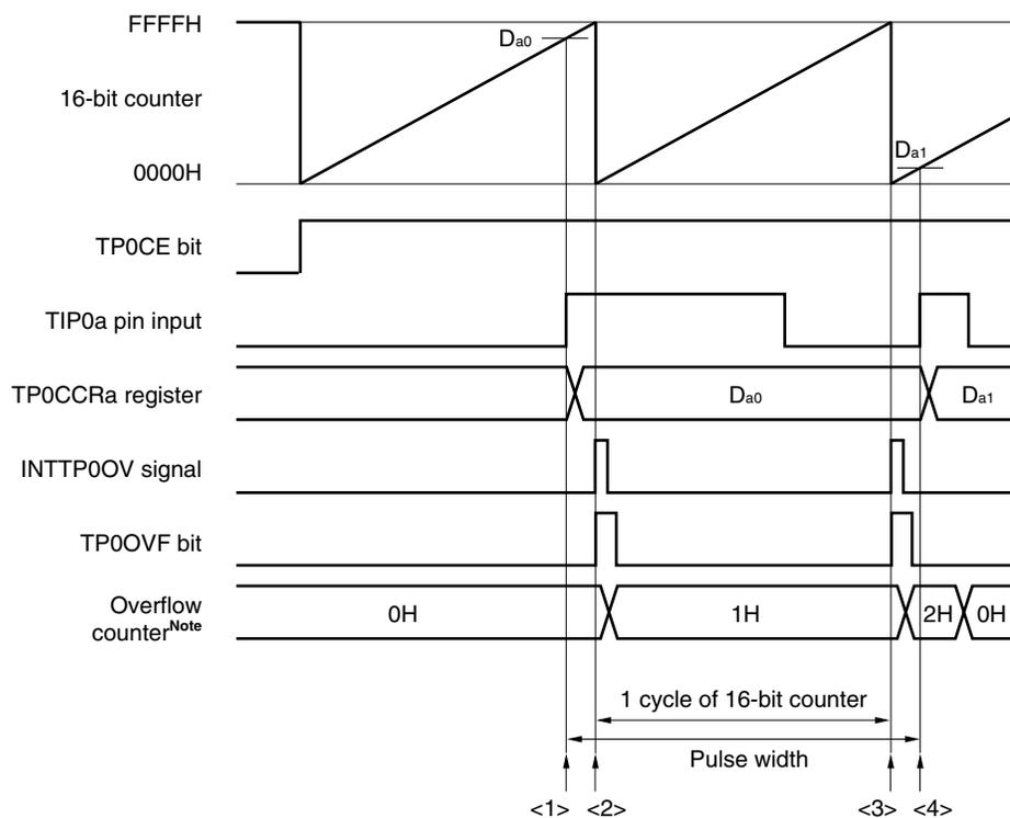
**Note** The overflow counter is set arbitrarily by software on the internal RAM.
