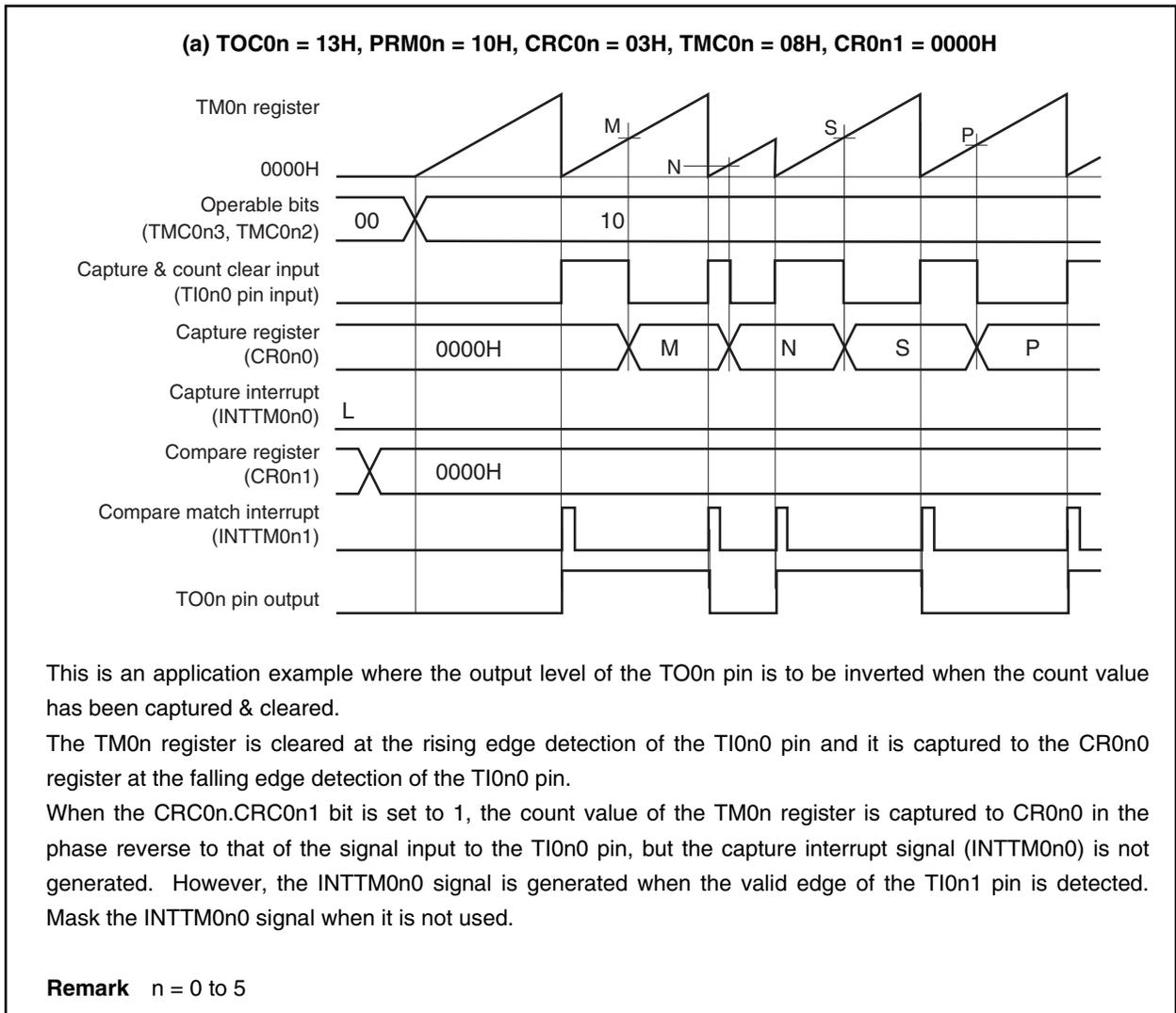
**Figure 8-18. Timing Example of Clear & Start Mode Entered by TIO<sub>n</sub>0 Pin Valid Edge Input
