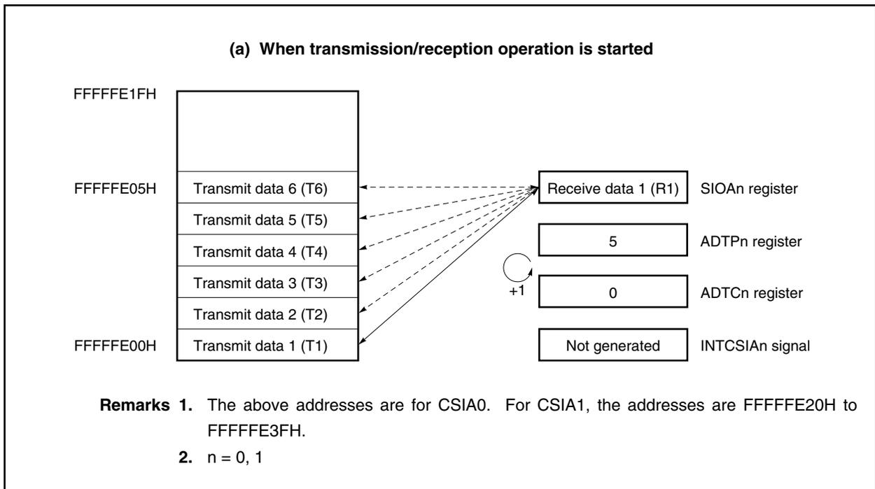
Figure 18-7. Buffer RAM Operation in 6-Byte Transmission/Reception (in Automatic Transmission/Reception Mode) (2/2)
