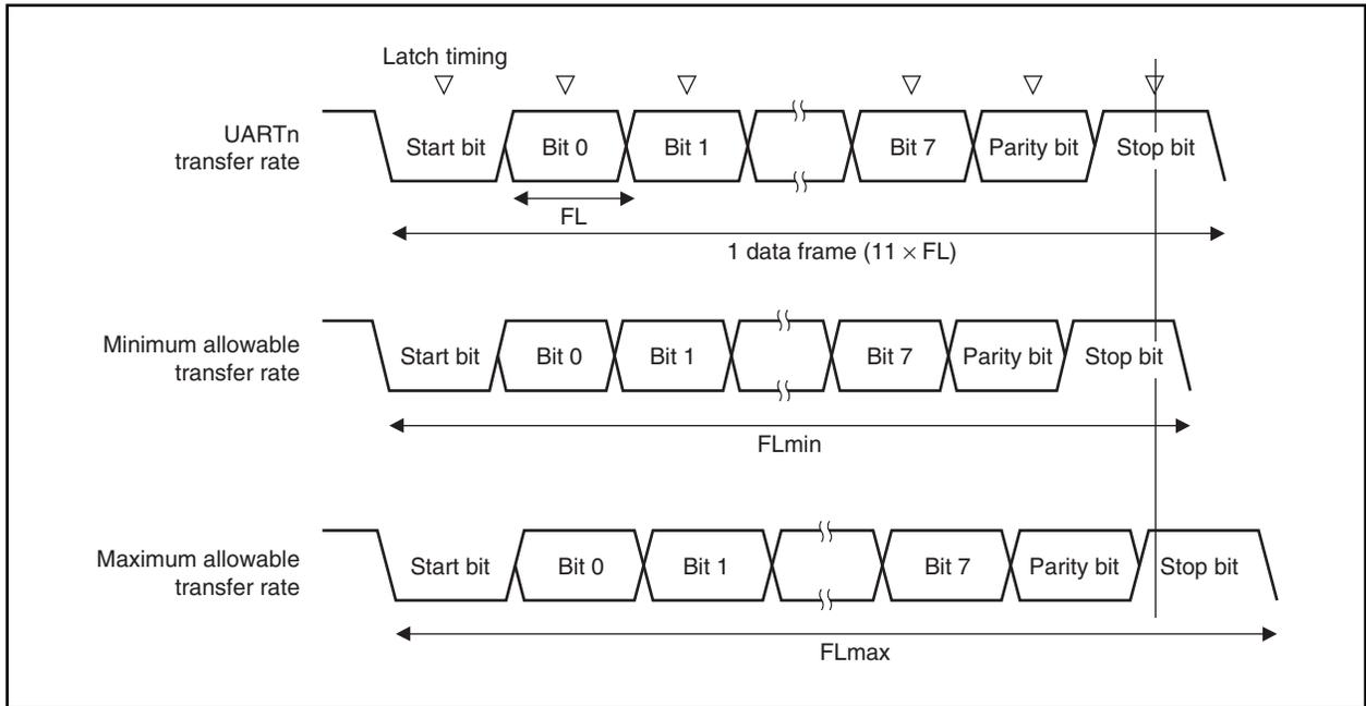
As shown in Figure 16-15, after the start bit is detected, the receive data latch timing is determined according to the counter that was set by the BRGCn register. If all data up to the final data (stop bit) is in time for this latch timing, the data can be received normally.
