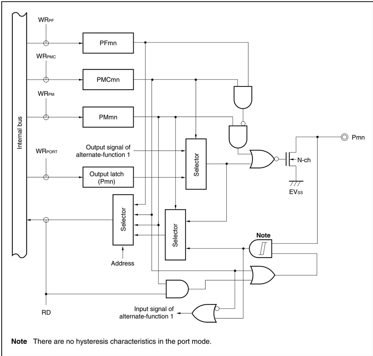
Figure 4-13. Block Diagram of Type D2-SUFL
