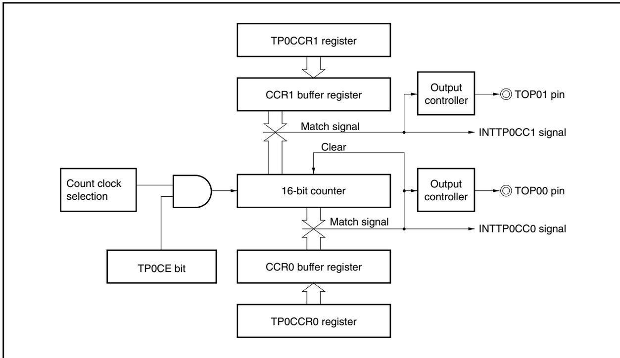
If the set value of the TP0CCR1 register is less than the set value of the TP0CCR0 register, the INTTP0CC1 signal is generated once per cycle. At the same time, the output of the TOP01 pin is inverted. The TOP01 pin outputs a square wave with the same cycle as that output by the TOP00 pin.
