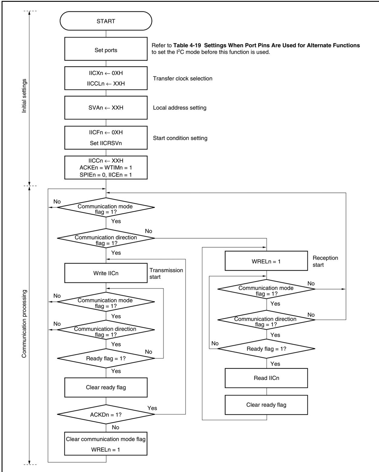
The following shows an example of the processing of the slave device by an INTIICn interrupt (it is assumed that no extension codes are used here). During an INTIICn interrupt, the status is confirmed and the following steps are executed.
