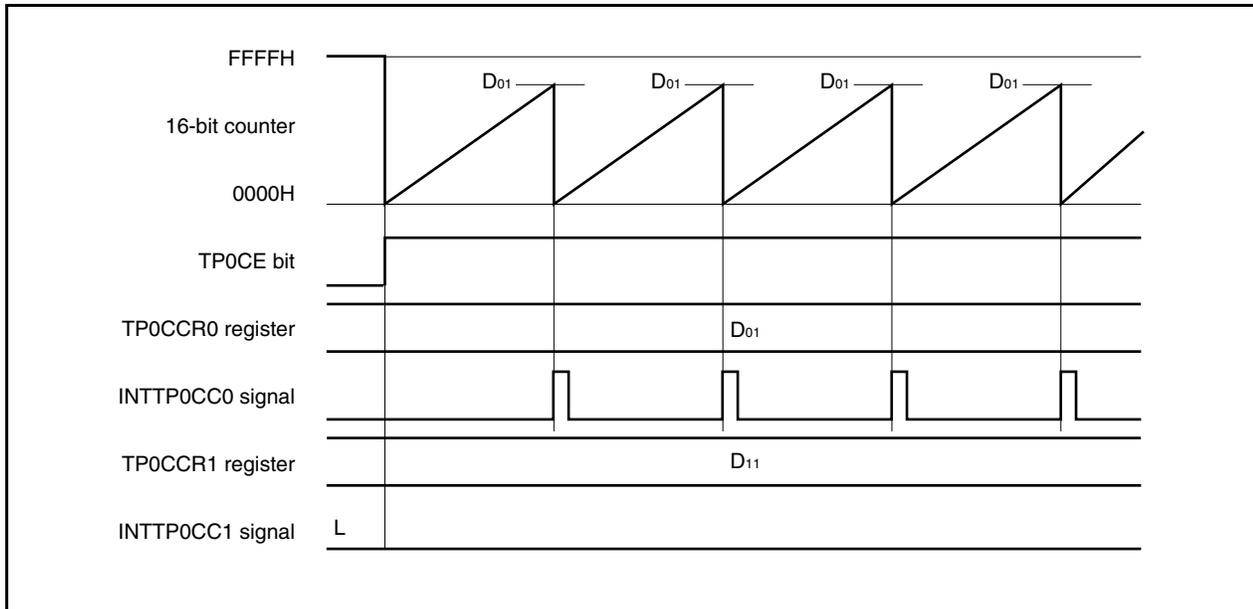
**7.5.3 External trigger pulse output mode (TP0MD2 to TP0MD0 bits = 010)**
