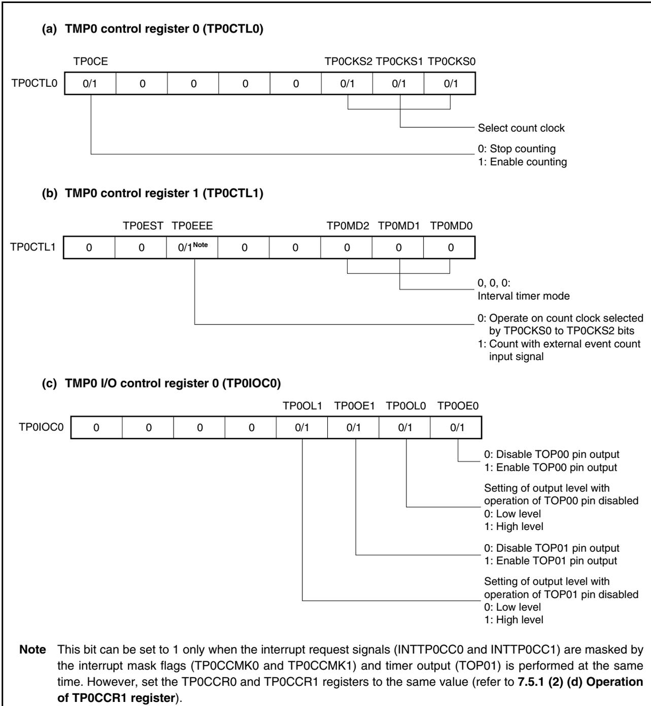
Figure 7-4. Register Setting for Interval Timer Mode Operation (2/2)
