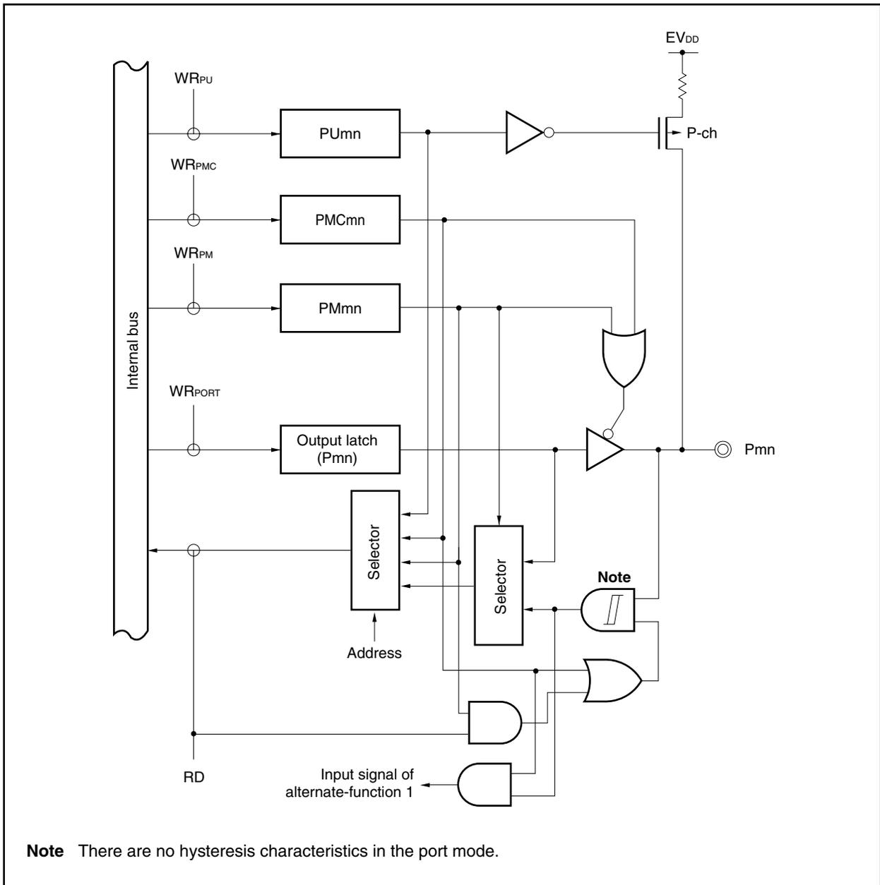
Figure 4-12. Block Diagram of Type D2-SNFH
