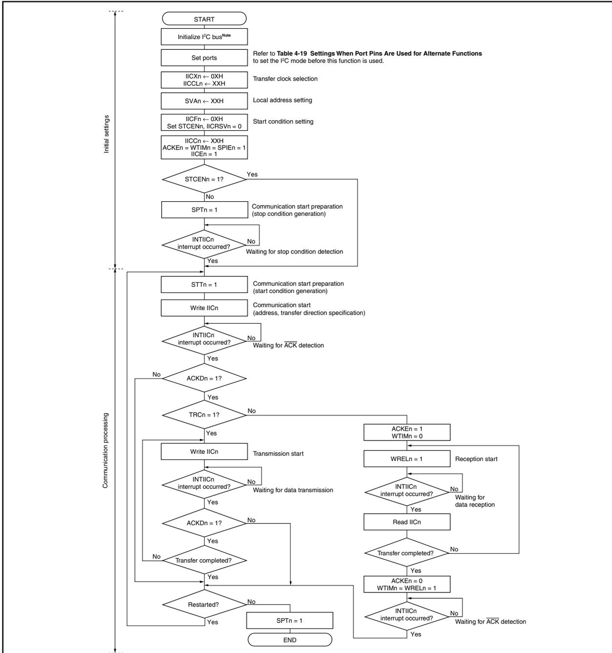
**Note** Release the I<sup>2</sup>Cn bus (SCLn, SDAn pins = high level) in conformity with the specifications of the product in communication.
