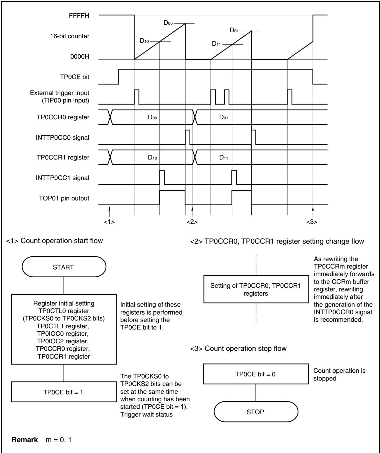
**(b) Generation timing of compare match interrupt request signal (INTTP0CC1)**
