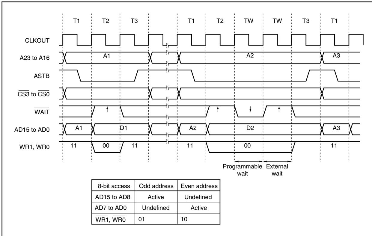
Figure 5-7. Multiplex Bus Write Timing (Bus Size: 8 Bits)
