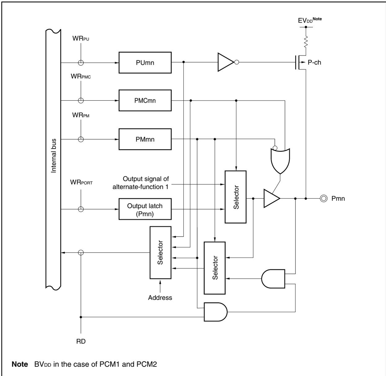
Figure 4-7. Block Diagram of Type D0-UF
