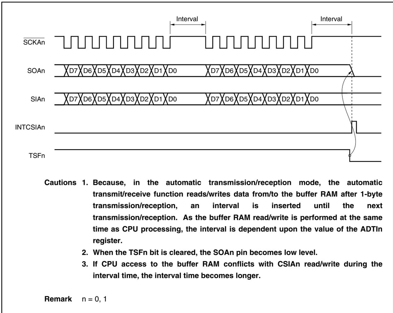
Figure 18-6. Automatic Transmission/Reception Mode Flowchart
