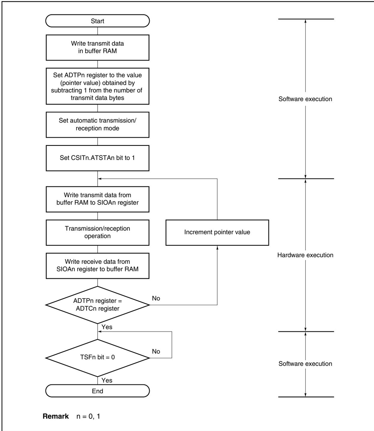
In 6-byte transmission/reception (CSIMAn.ATMn bit = 0, CSIMAn.RXEAn bit = 1, CSIMAn.TXEAn bit = 1) in automatic transmission/reception mode, buffer RAM operates as follows.
