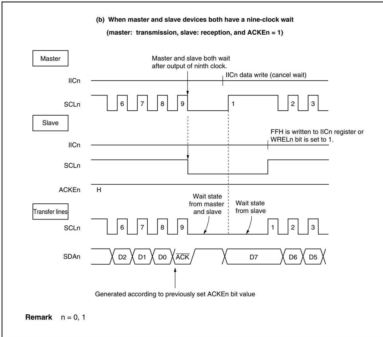
A wait state is automatically generated after a start condition is generated. Moreover, a wait state is automatically generated depending on the setting of the IICn.WTIMn bit.
