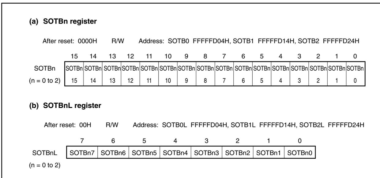
**(6) Clocked serial interface initial transmit buffer registers n, nL (SOTBFn, SOTBFnL)**
