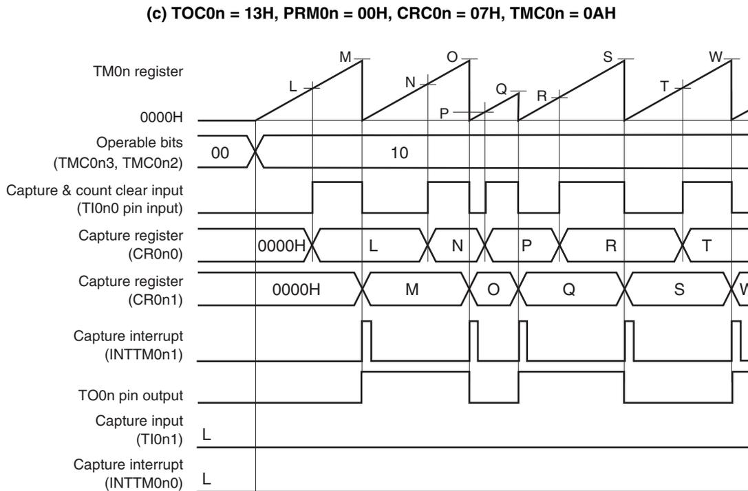
This is an application example where the pulse width of the signal input to the TI0n0 pin is measured.
