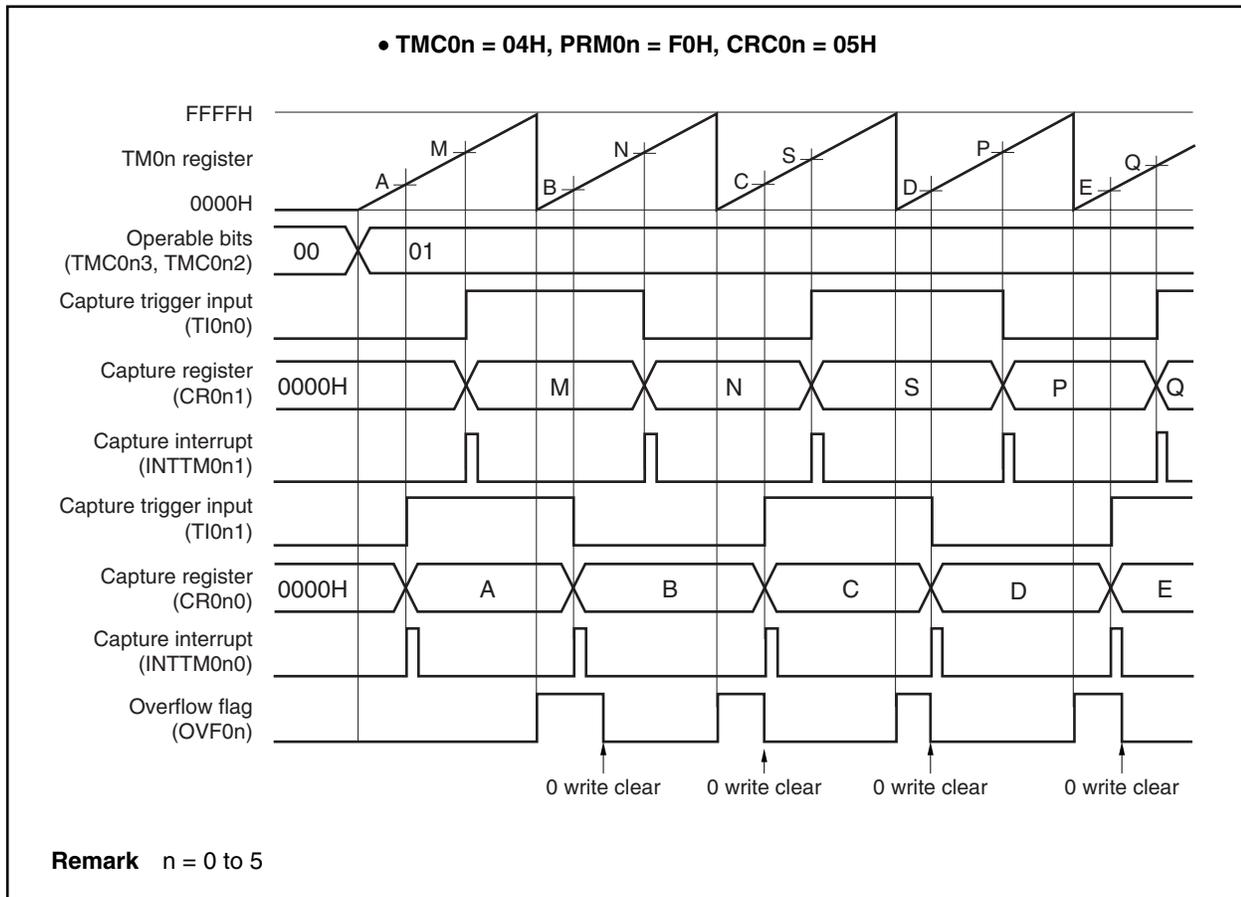
**(2) Measuring the pulse width by using one input signal of the TI0n0 pin (free-running timer mode)**
