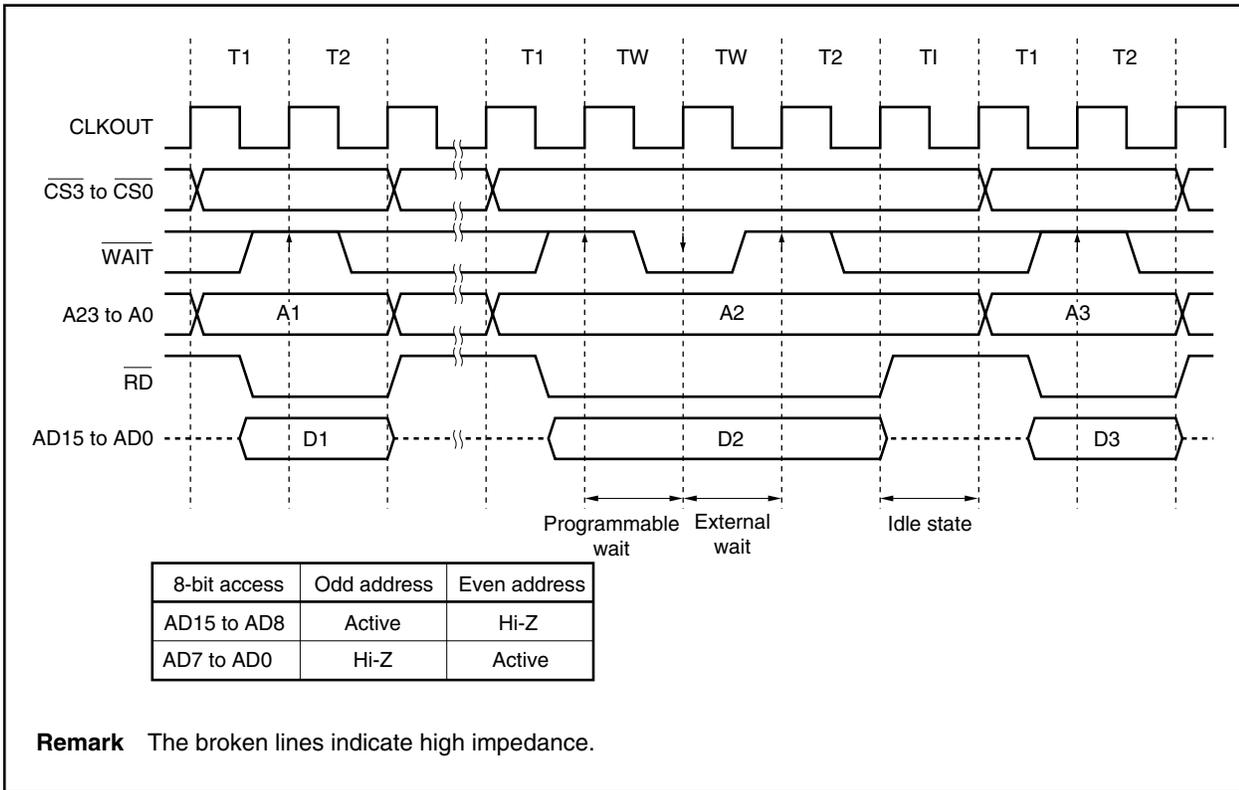
Figure 5-10. Separate Bus Read Timing (Bus Size: 8 Bits)
