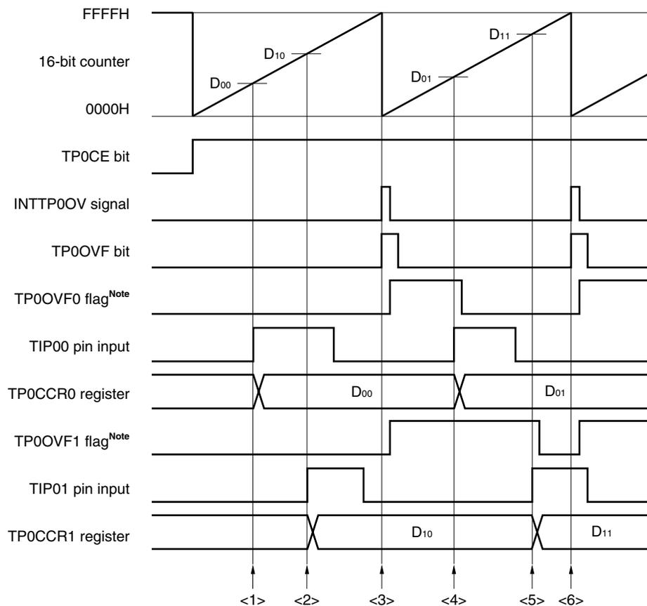
**Note** The TP0OVF0 and TP0OVF1 flags are set on the internal RAM by software.
