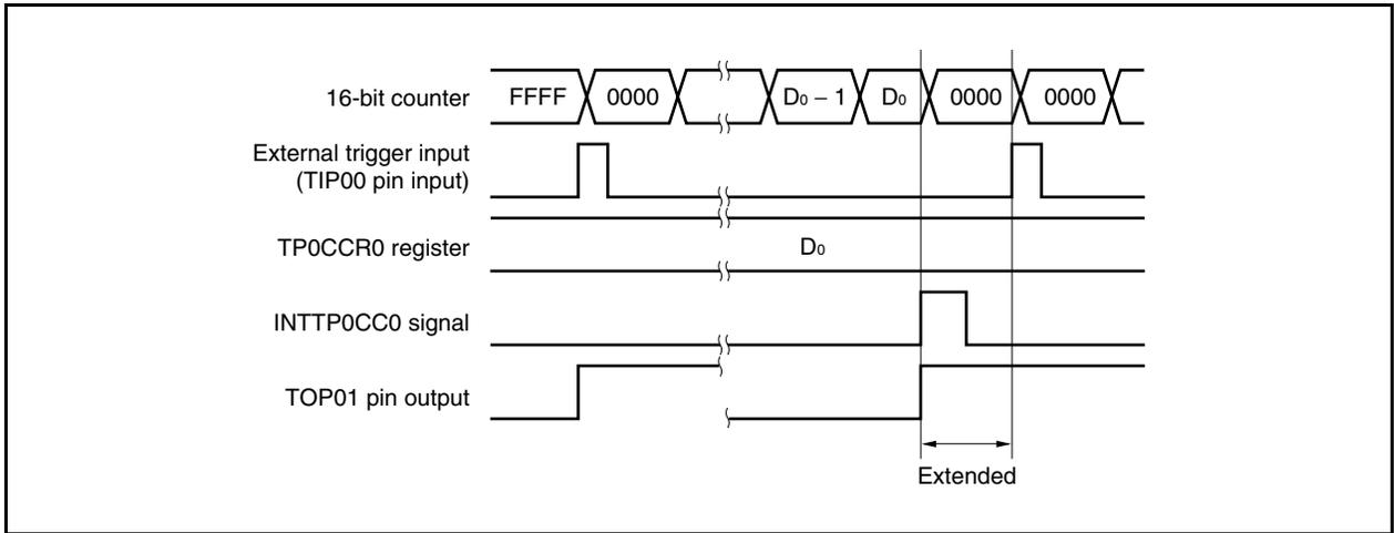
If the trigger is detected immediately before the INTTP0CC0 signal is generated, the INTTP0CC0 signal is not generated. The 16-bit counter is cleared to 0000H, the TOP01 pin is asserted, and the counter continues counting. Consequently, the inactive period of the PWM waveform is shortened.
