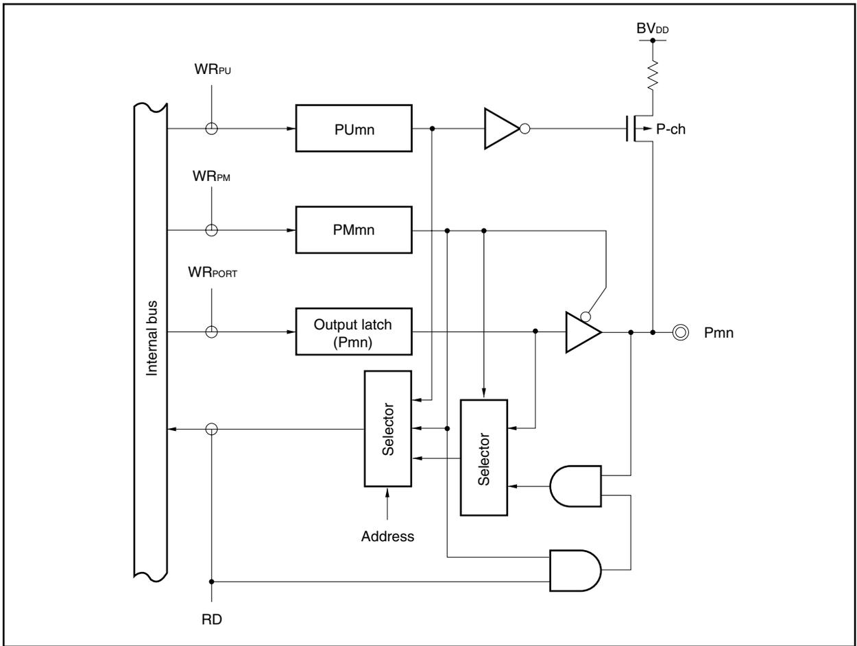
Figure 4-5. Block Diagram of Type C-UA
