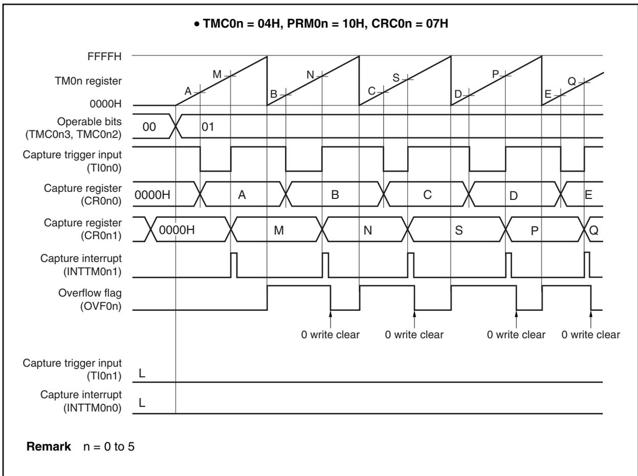
**(3) Measuring the pulse width by using one input signal of the TI0n0 pin (clear & start mode entered by the TI0n0 pin valid edge input)**
