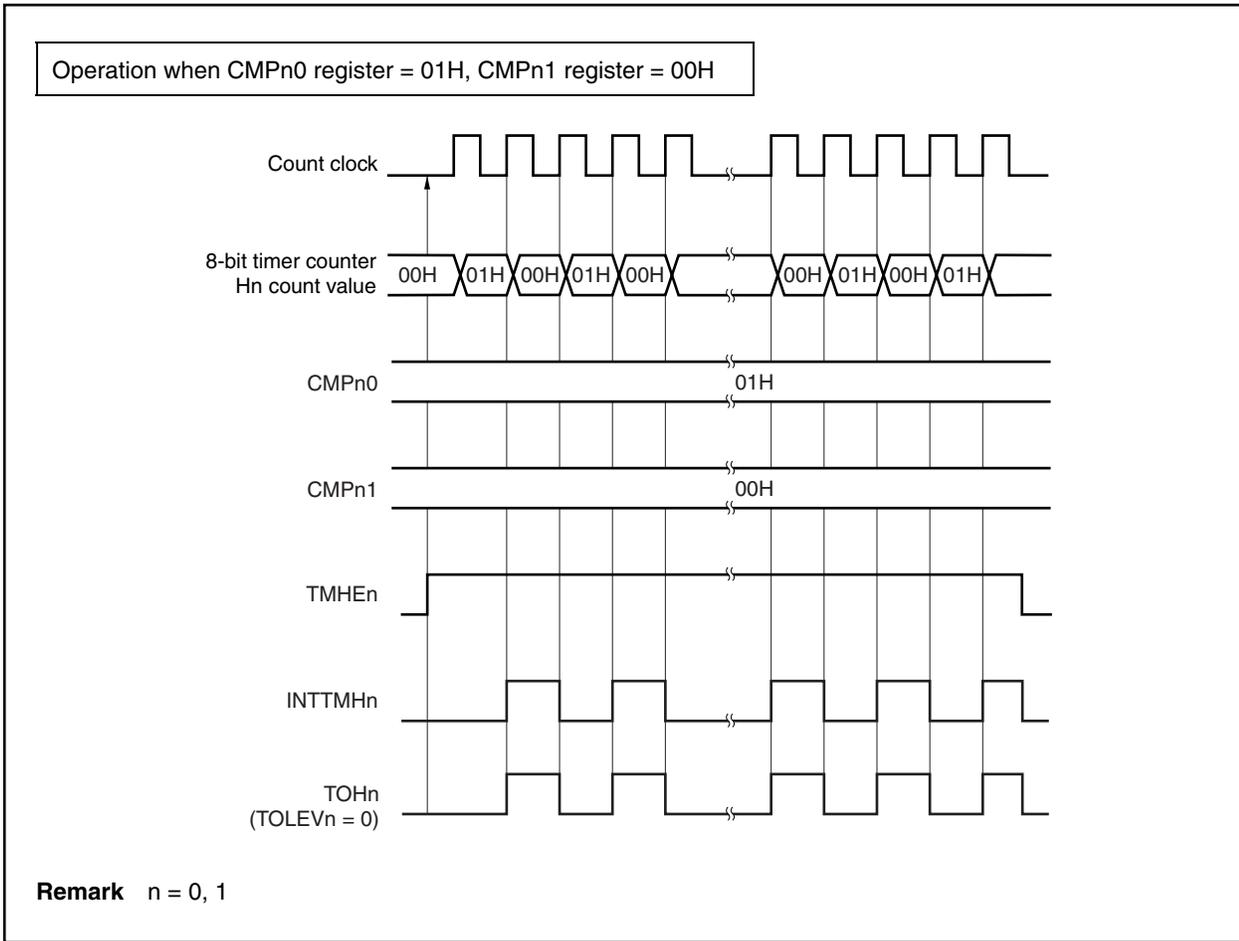
Figure 10-5. Operation Timing in PWM Output Mode (4/4)
