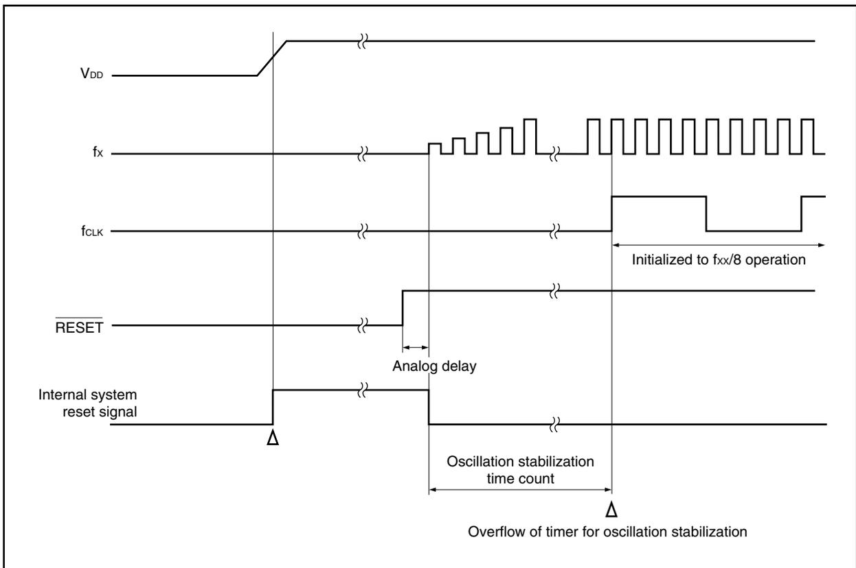
Figure 24-4. Timing of Reset Operation by Watchdog Timer 1
