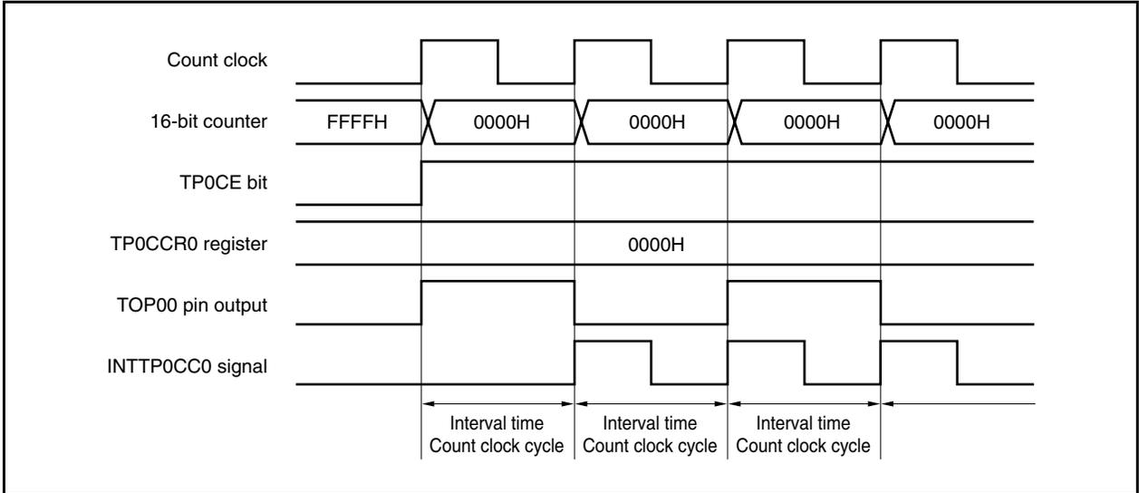
**(b) Operation if TP0CCR0 register is set to FFFFH**
