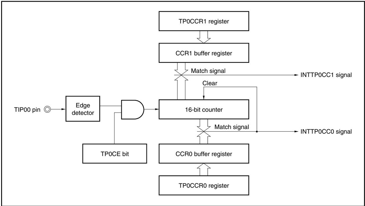
If the set value of the TP0CCR1 register is smaller than the set value of the TP0CCR0 register, the INTTP0CC1 signal is generated once per cycle.
