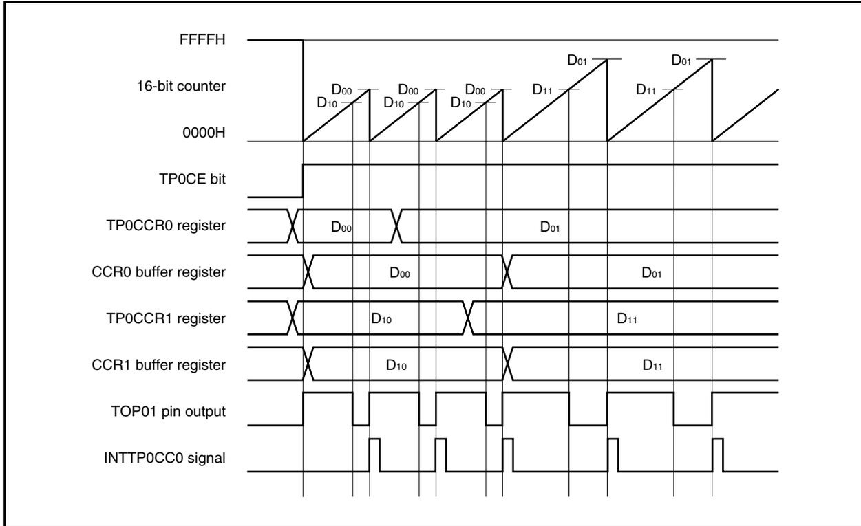
To transfer data from the TP0CCRa register to the CCRa buffer register, the TP0CCR1 register must be written.
