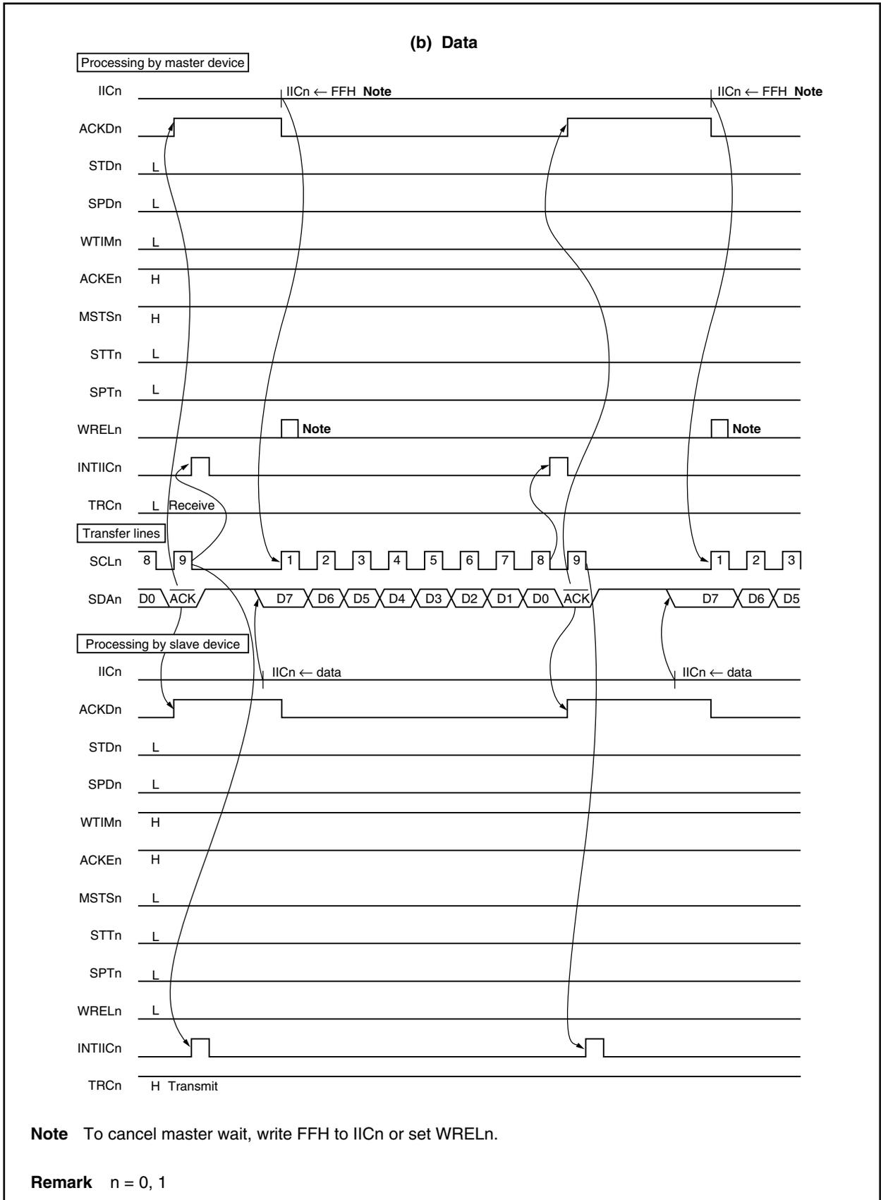
**Figure 19-22. Example of Slave to Master Communication
