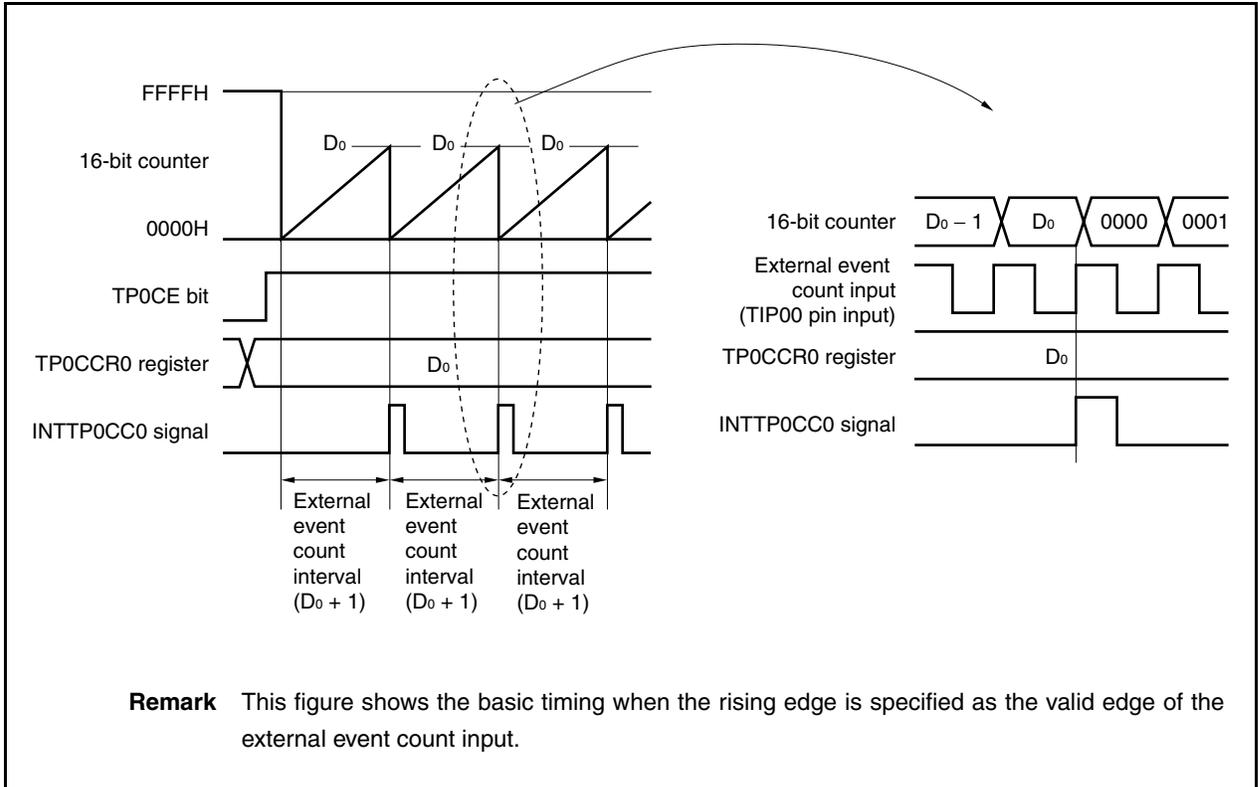
Figure 7-11. Register Setting for Operation in External Event Count Mode (2/2)
