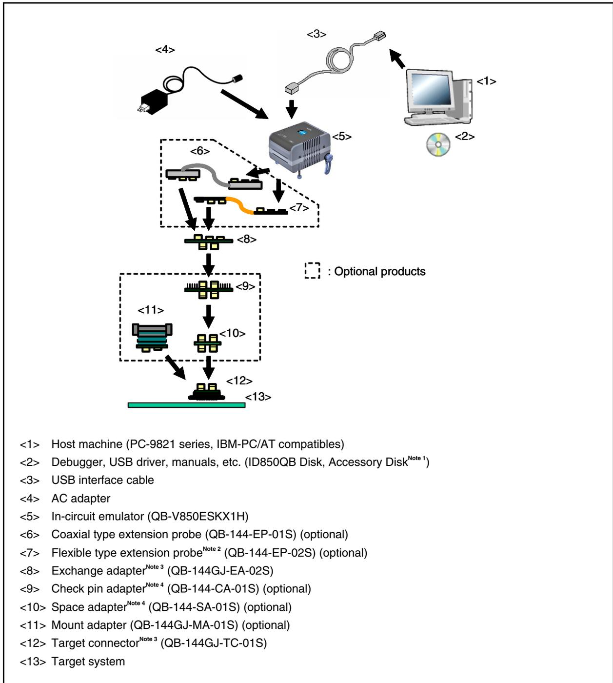
Figure A-2. System Configuration (When Using QB-V850ESKX1H) (2/2)
