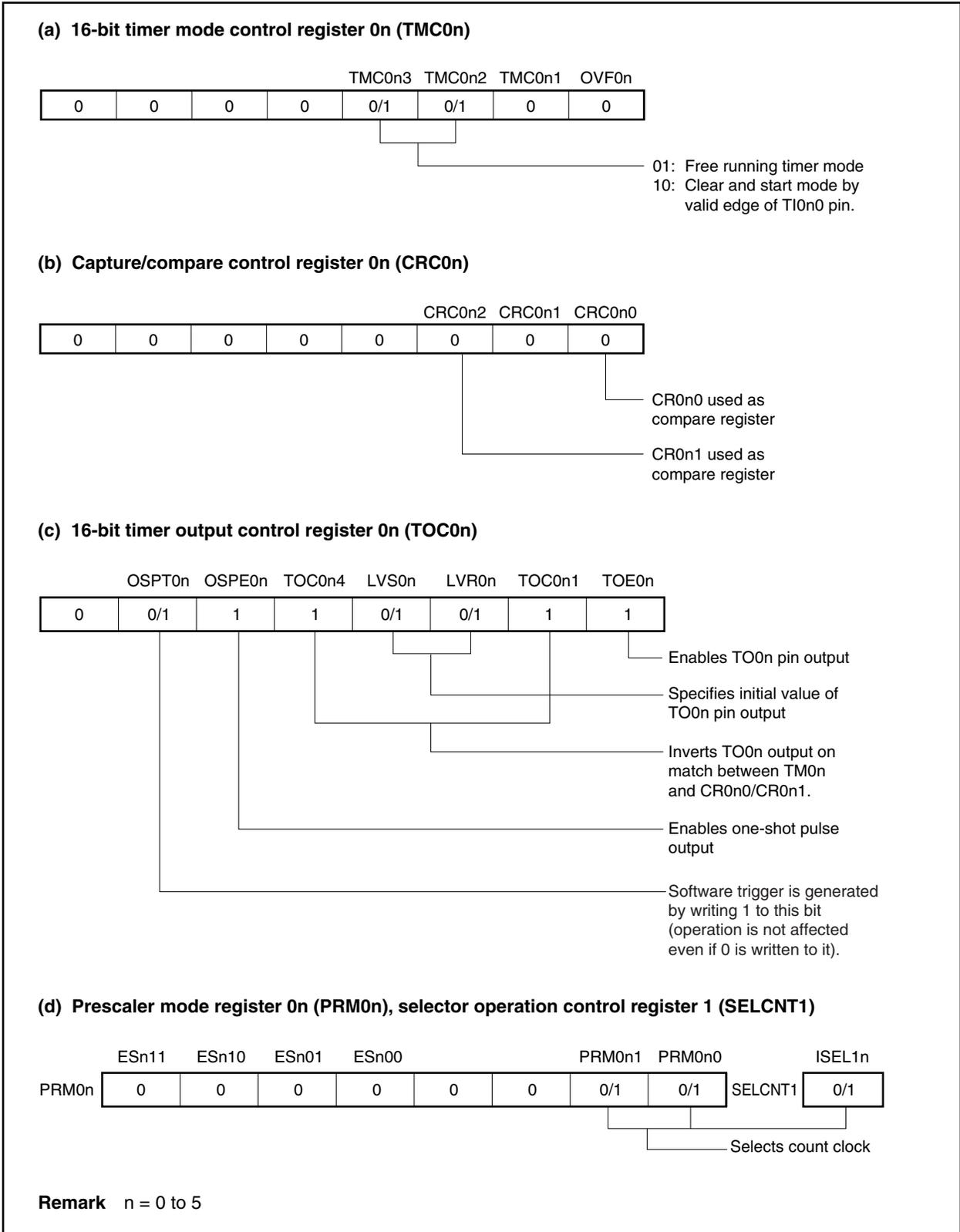
Figure 8-35. Example of Register Settings for One-Shot Pulse Output Operation (2/2)
