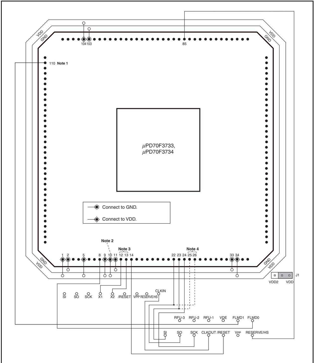
Figure 26-6. Wiring Example of V850ES/KJ2 Flash Writing Adapter (FA-144GJ-UEN-A) (2/2)
