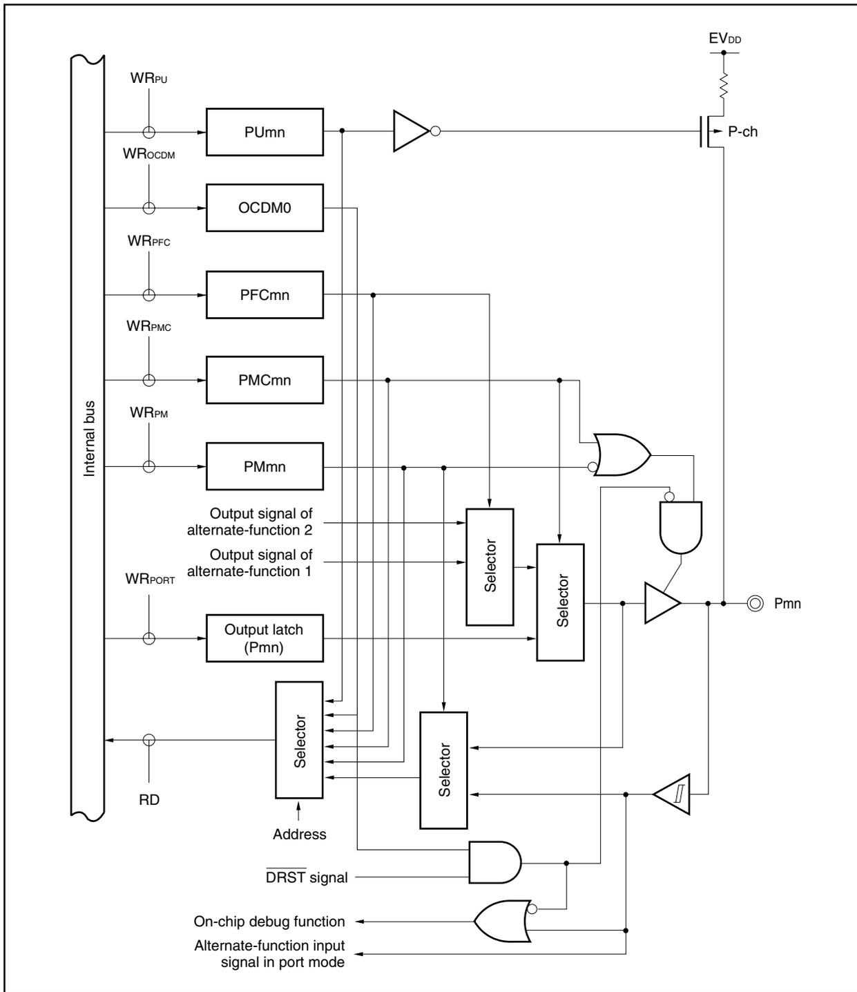
Figure 4-36. Block Diagram of Type OE100-SULT
