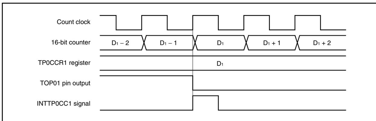
Usually, the INTTP0CC1 signal is generated in synchronization with the next counting up after the count value of the 16-bit counter matches the value of the TP0CCR1 register.
