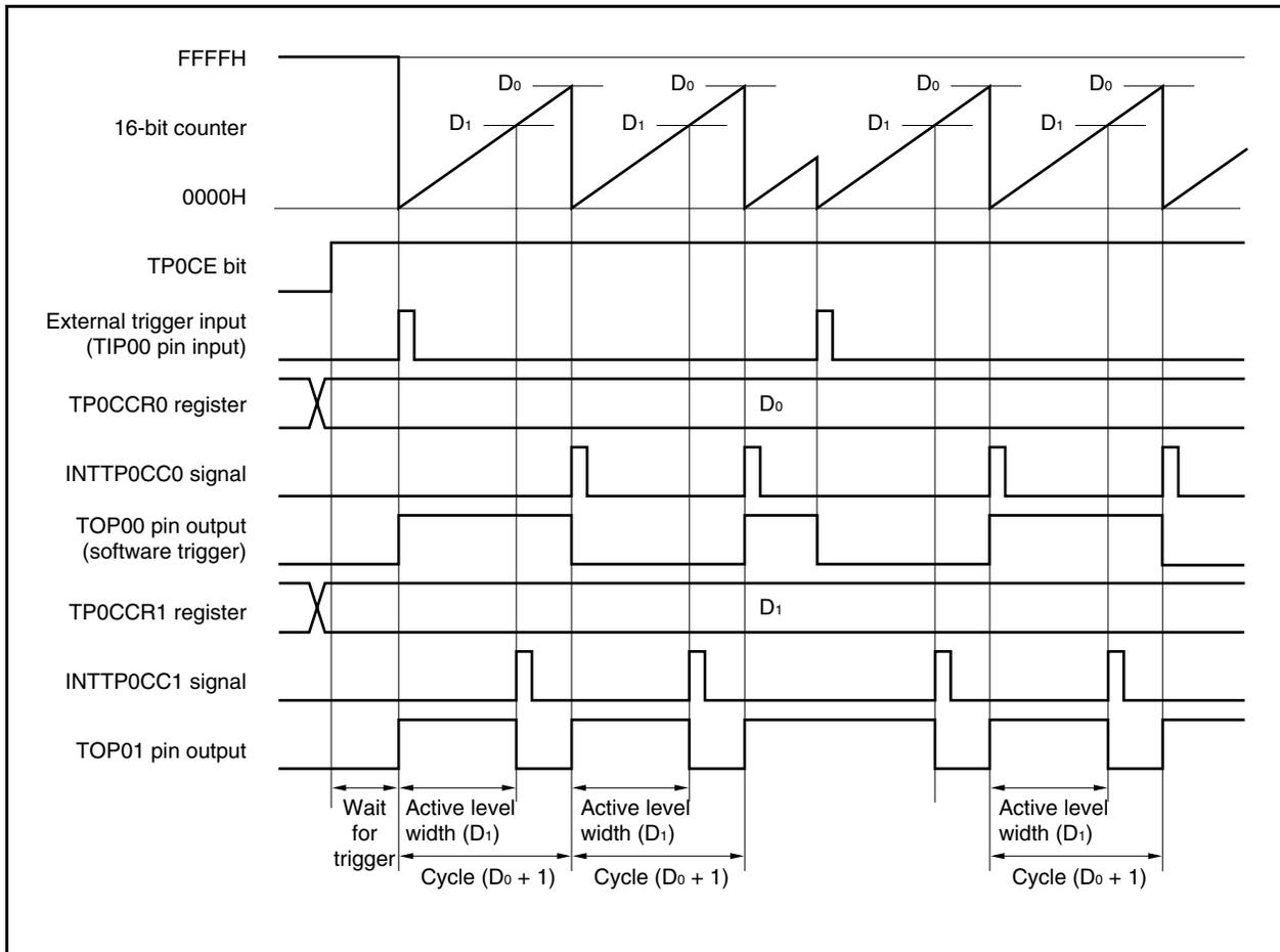
16-bit timer/event counter P waits for a trigger when the TP0CE bit is set to 1. When the trigger is generated, the 16-bit counter is cleared from FFFFH to 0000H, starts counting at the same time, and outputs a PWM waveform from the TOP01 pin. If the trigger is generated again while the counter is operating, the counter is cleared to 0000H and restarted. (The output of the TOP00 pin is inverted. The TOP01 pin outputs a high level regardless of the status (high/low) when a trigger occurs.)
