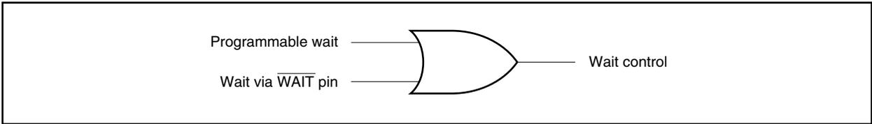
For example, if the timing of the programmable wait and the  $\overline{\text{WAIT}}$  pin signal is as illustrated below, three wait states will be inserted in the bus cycle.
