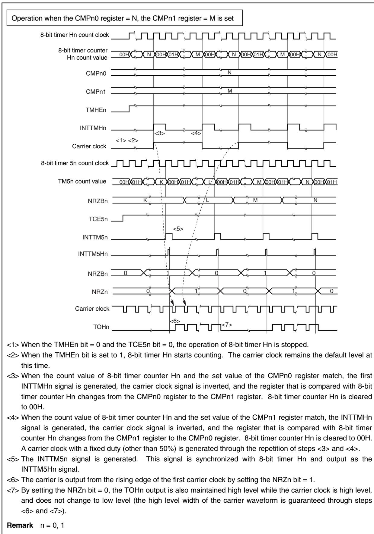
Figure 10-8. Carrier Generator Mode (3/3)
