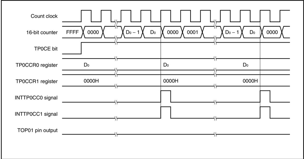
To output a 100% waveform, set a value of (set value of TP0CCR0 register + 1) to the TP0CCR1 register. If the set value of the TP0CCR0 register is FFFFH, 100% output cannot be produced.
