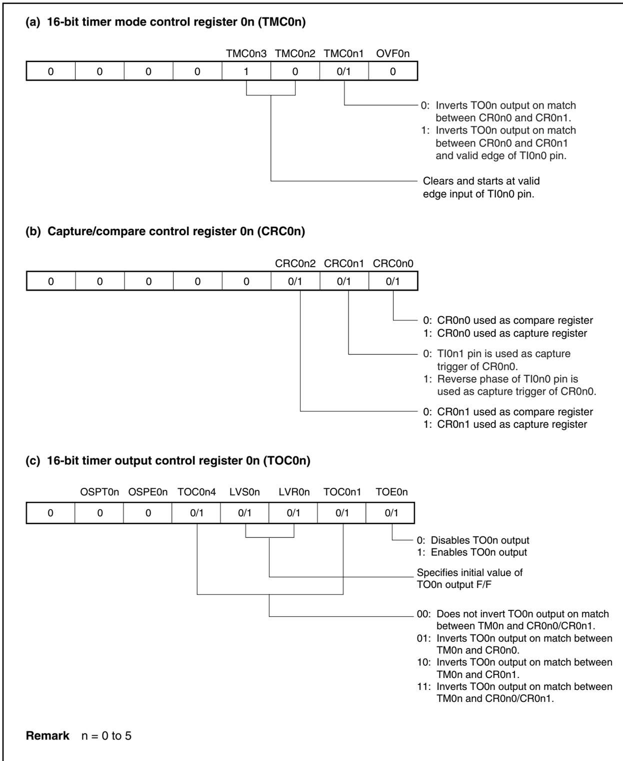
Figure 8-21. Example of Register Settings in Clear &amp; Start Mode Entered by TI0n0 Pin Valid Edge Input (2/2)
