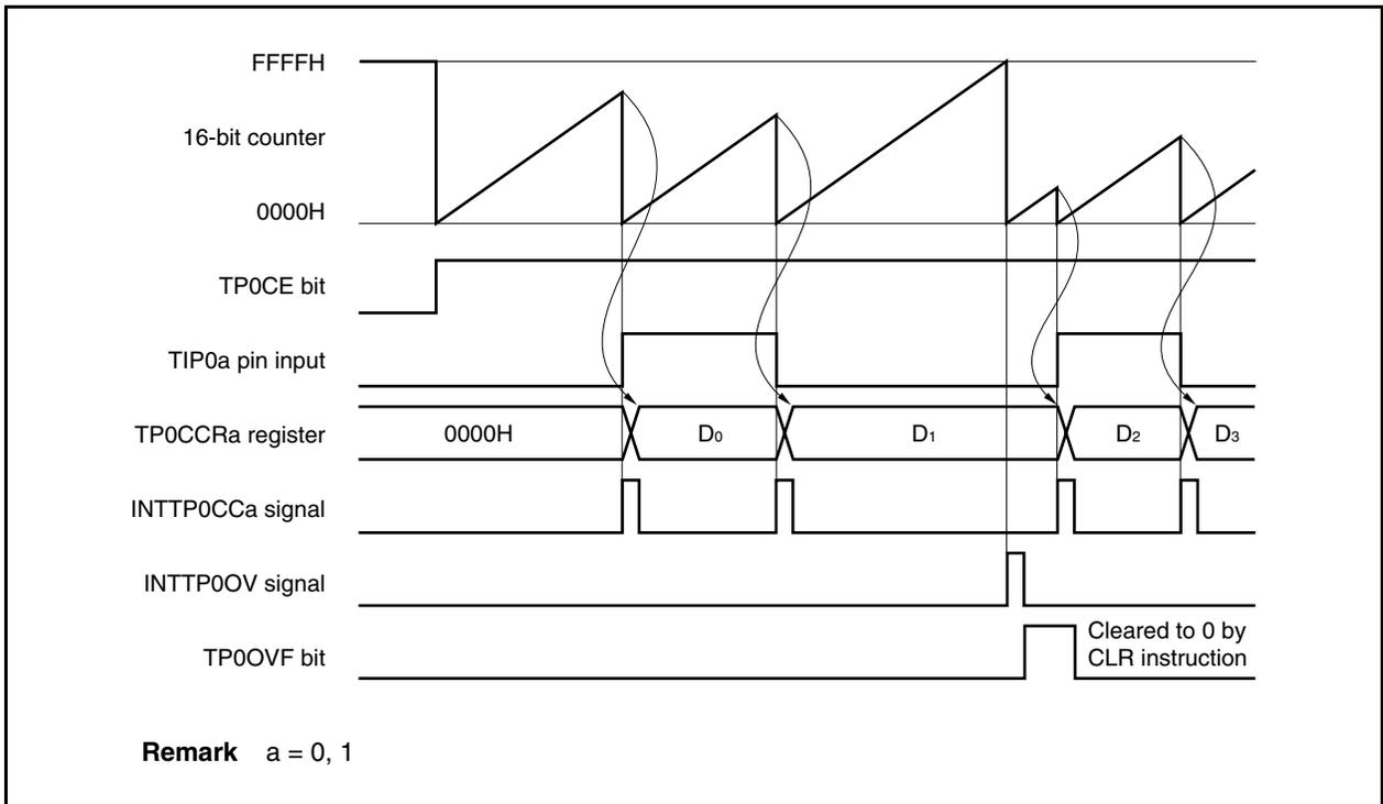
When the TP0CE bit is set to 1, the 16-bit counter starts counting. When the valid edge input to the TIP0a pin is later detected, the count value of the 16-bit counter is stored in the TP0CCRa register, the 16-bit counter is cleared to 0000H, and a capture interrupt request signal (INTTP0CCa) is generated.
