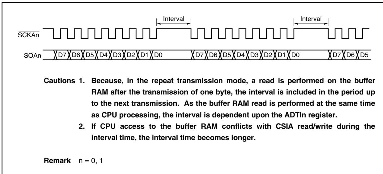
Figure 18-12. Repeat Transmission Mode Flowchart
