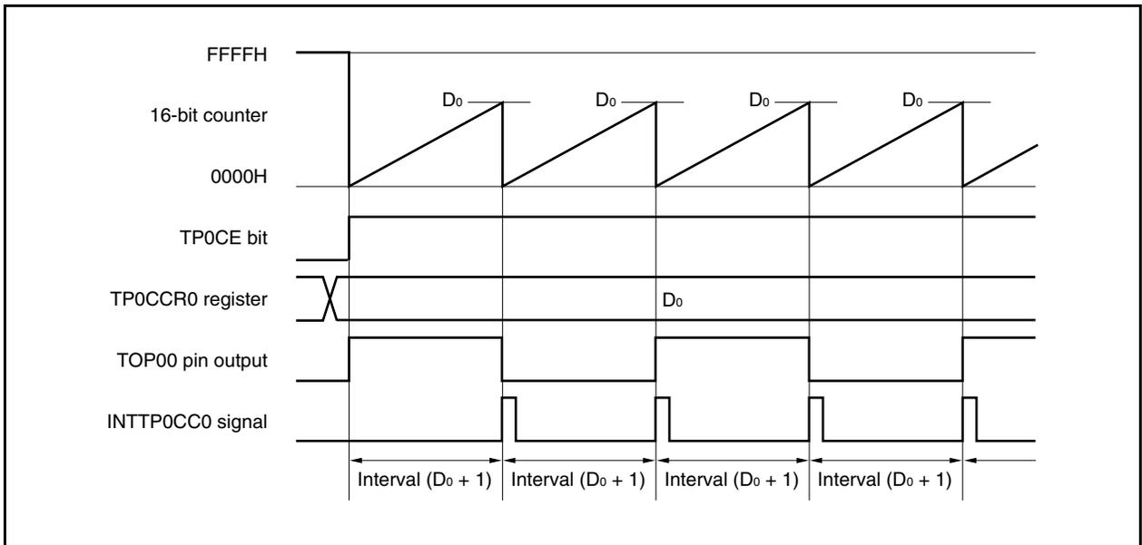
When the TP0CE bit is set to 1, the value of the 16-bit counter is cleared from FFFFH to 0000H in synchronization with the count clock, and the counter starts counting. At this time, the output of the TOP00 pin is inverted. Additionally, the set value of the TP0CCR0 register is transferred to the CCR0 buffer register.
