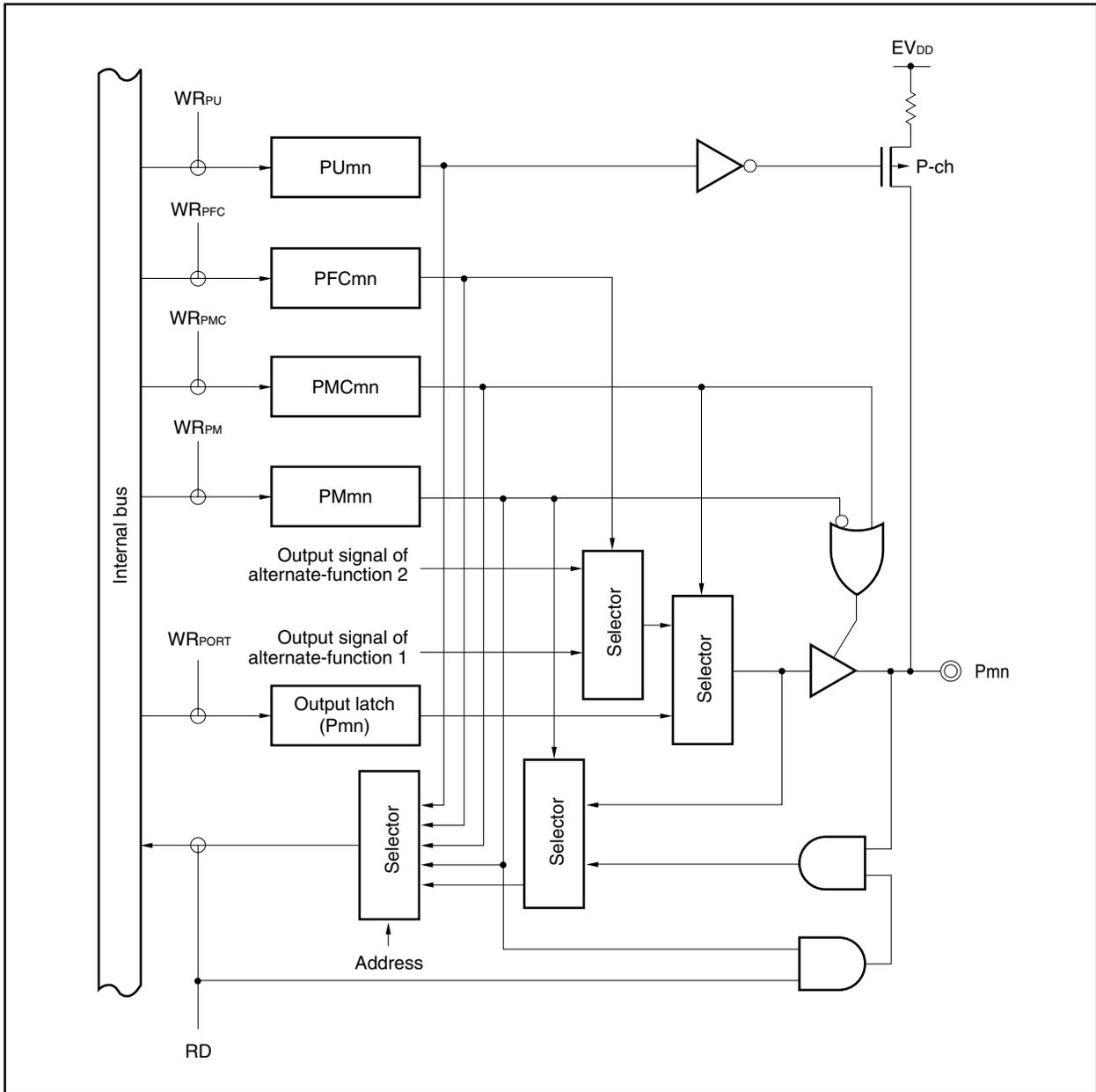
Figure 4-19. Block Diagram of Type E00-UF
