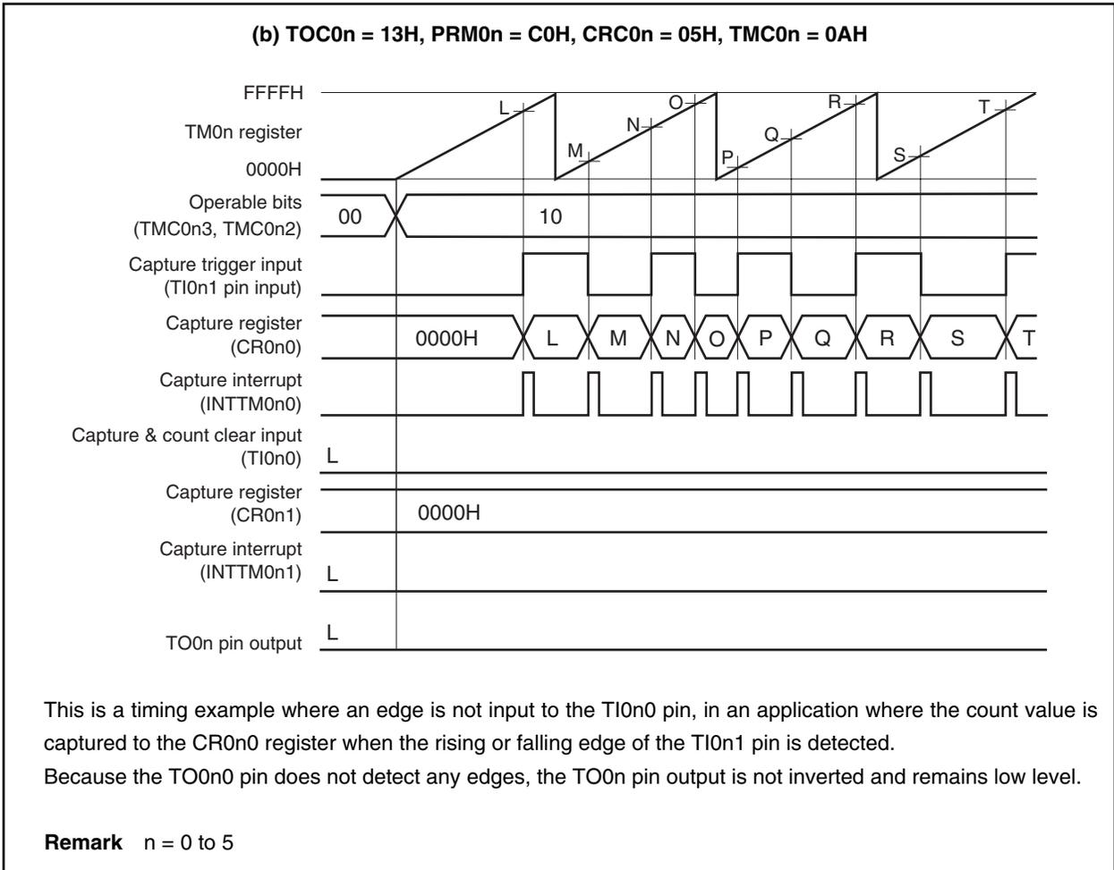
**Figure 8-20. Timing Example of Clear & Start Mode Entered by TI0n0 Pin Valid Edge Input (CR0n0 Register: Capture Register, CR0n1 Register: Capture Register) (3/3)**
