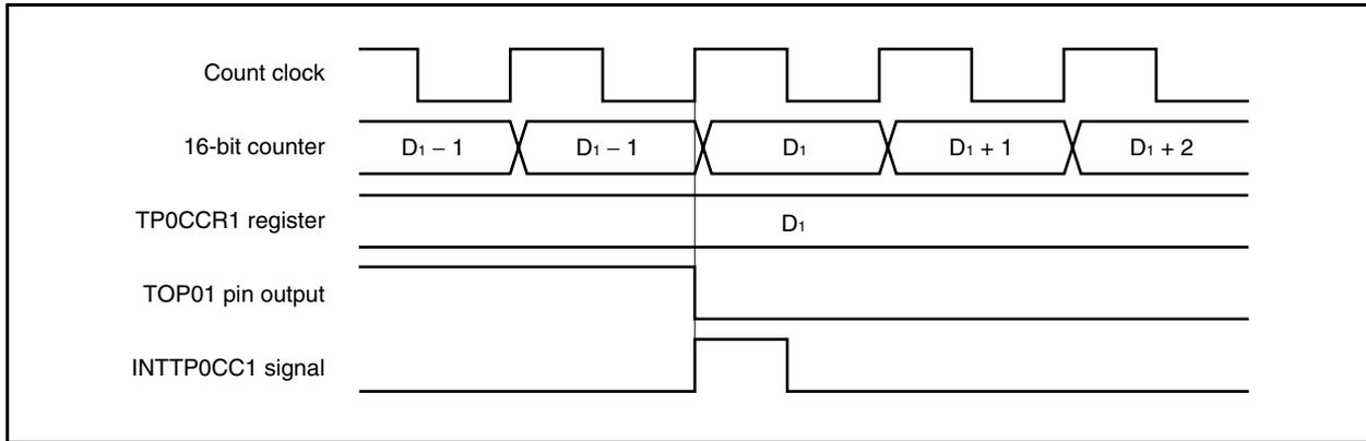
Usually, the INTTP0CC1 signal is generated in synchronization with the next count up, after the count value of the 16-bit counter matches the value of the TP0CCR1 register.
