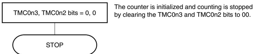
**Note** Care must be exercised when setting the TOC0n register. For details, see 8.3 (3) 16-bit timer output control register 0n (TOC0n).
