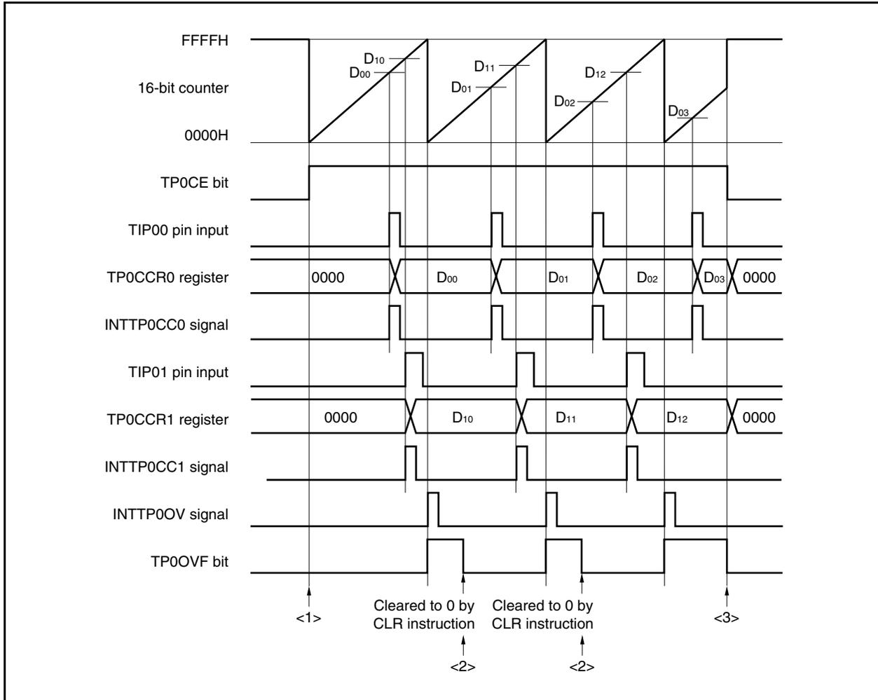
Figure 7-33. Software Processing Flow in Free-Running Timer Mode (Capture Function) (2/2)
