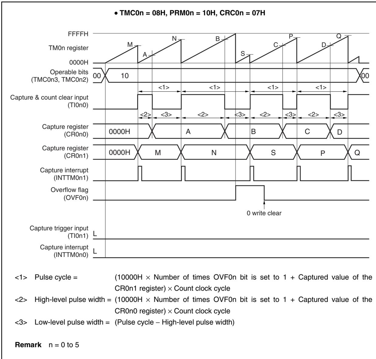
Figure 8-42. Example of Register Settings for Pulse Width Measurement (1/2)
