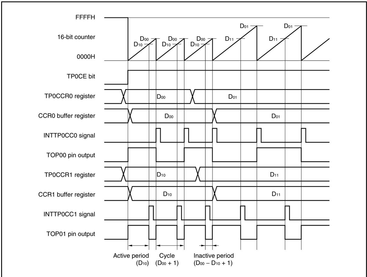
When the TPOCE bit is set to 1, the 16-bit counter is cleared from FFFFH to 0000H, starts counting, and outputs a PWM waveform from the TOP01 pin.
