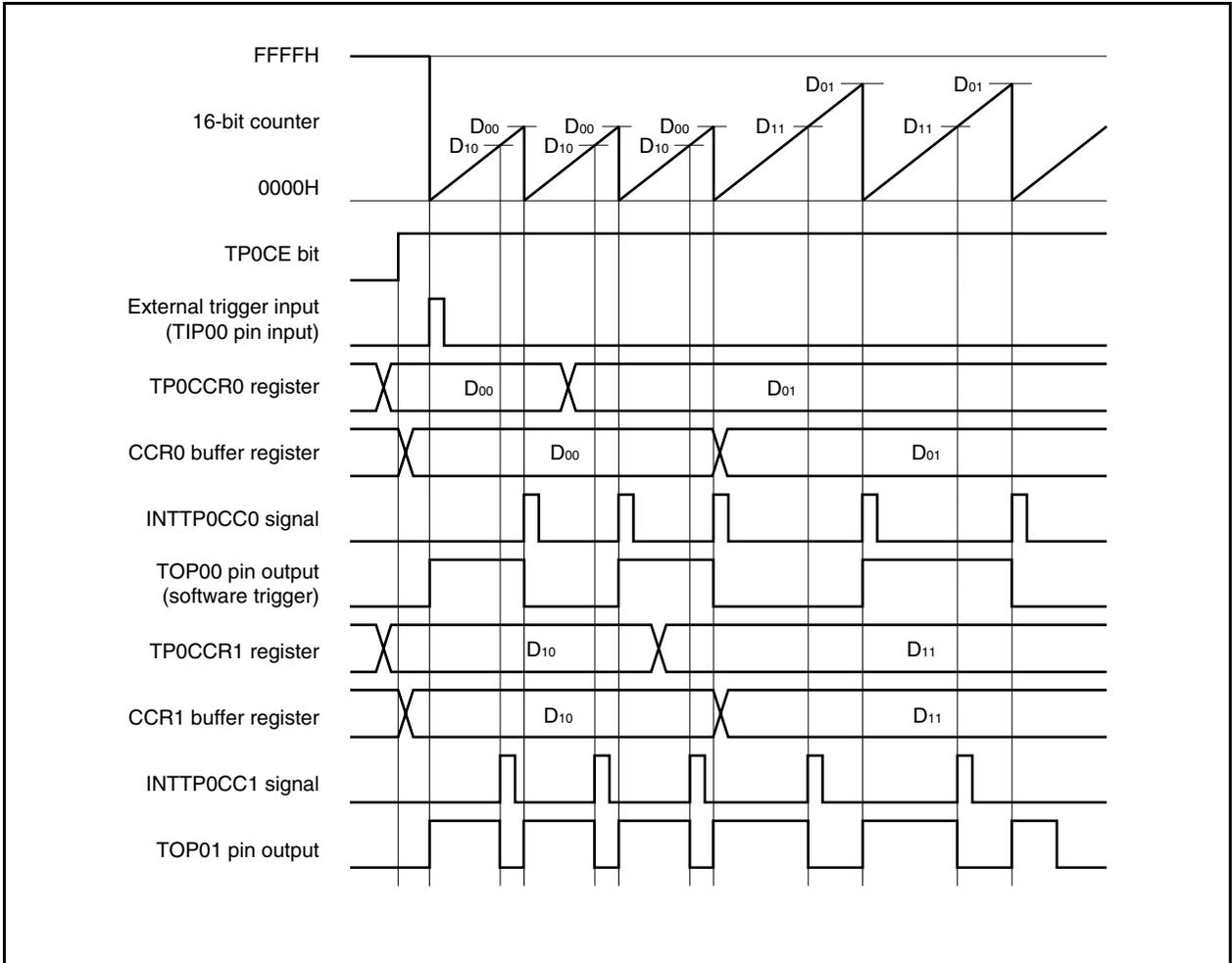
In order to transfer data from the TP0CCRa register to the CCRa buffer register, the TP0CCR1 register must be written.
