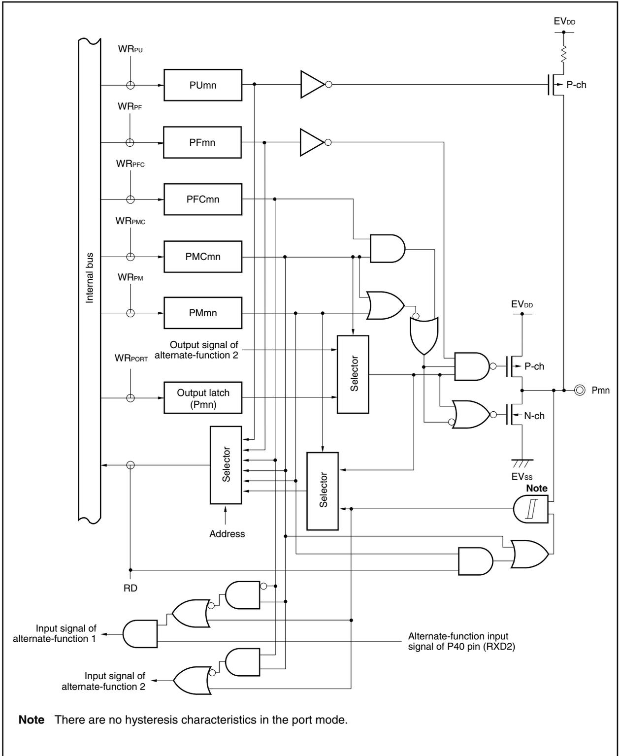
Figure 4-31. Block Diagram of Type E20-SUFLT
