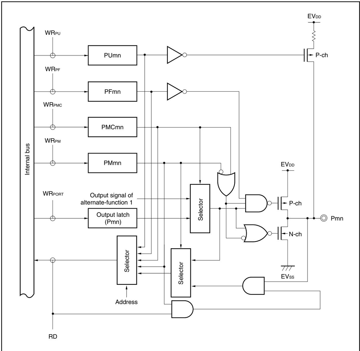
Figure 4-8. Block Diagram of Type D0-UZ
