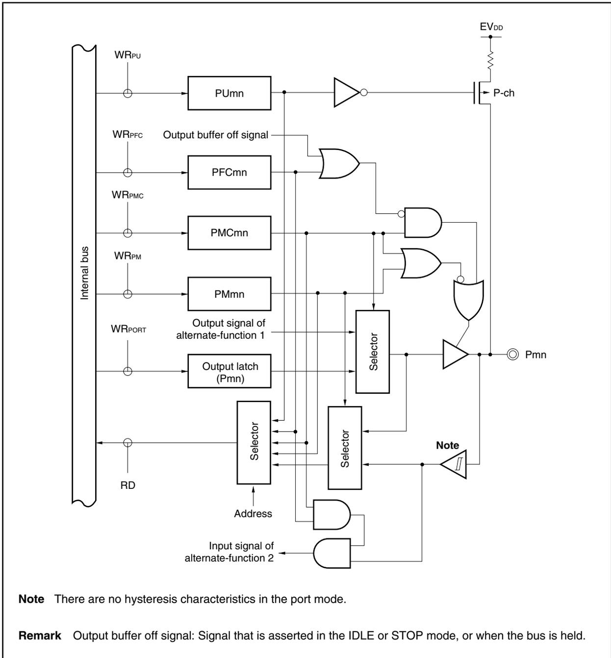
Figure 4-24. Block Diagram of Type E02-SUFH
