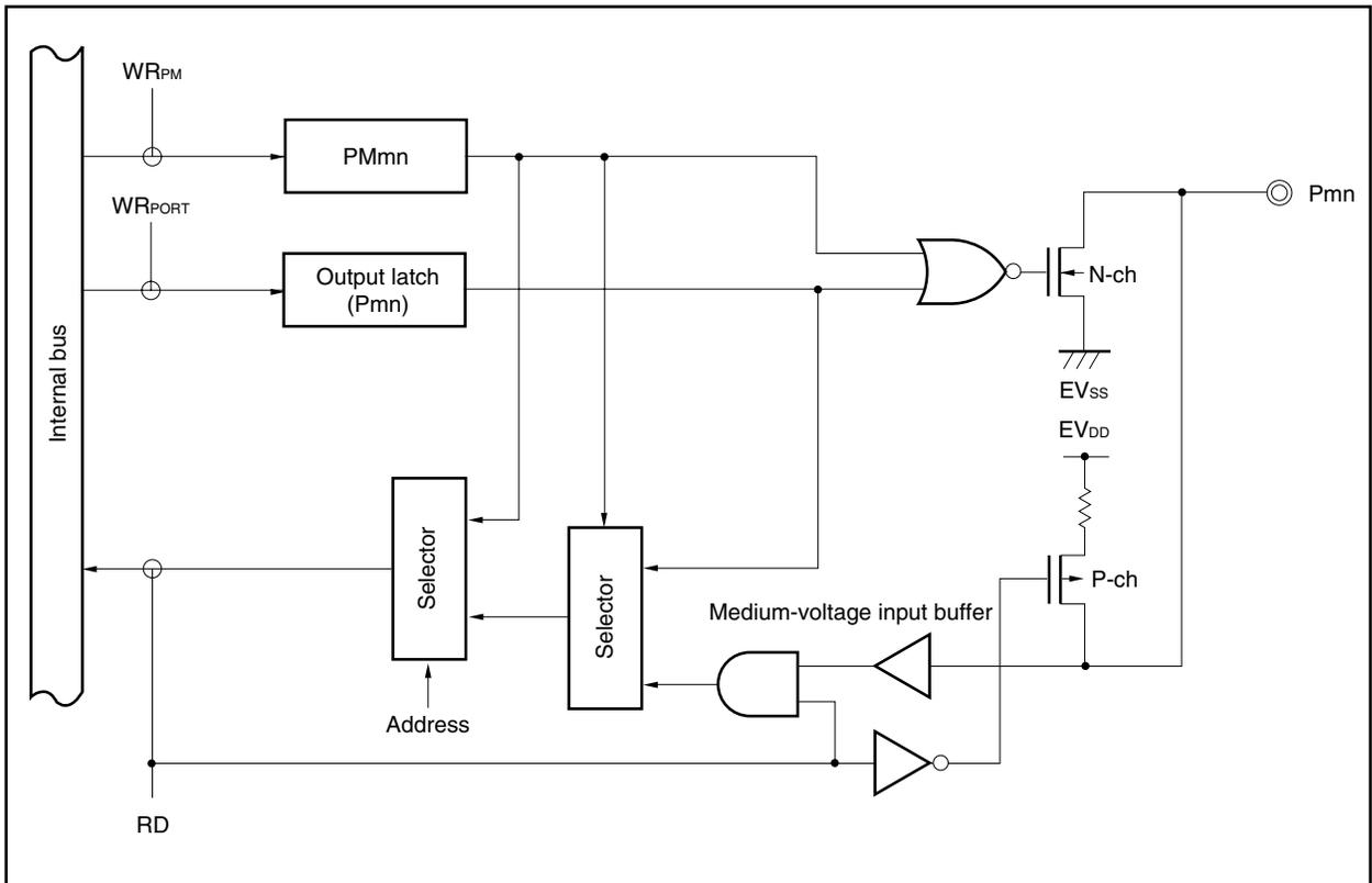
Figure 4-4. Block Diagram of Type C-U
