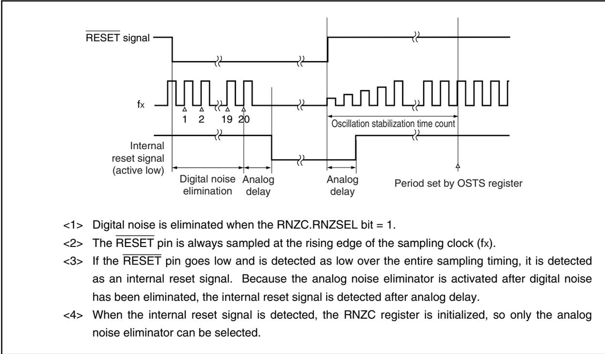
**(b) Operation when sampling clock is stopped**
