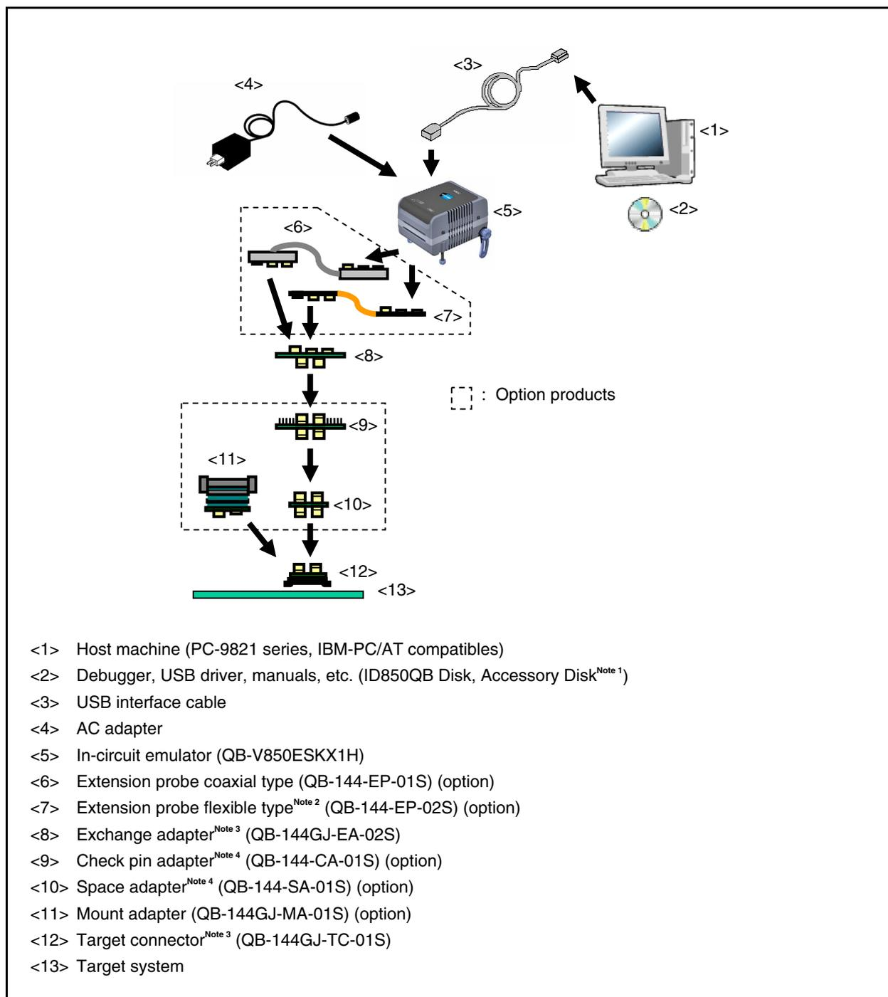
Figure A-2. System Configuration (QB-V850ESKX1H Used) (2/2)
