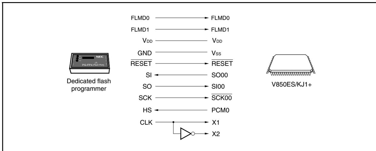
The dedicated flash programmer outputs the transfer clock, and the V850ES/KJ1+ operates as a slave.
