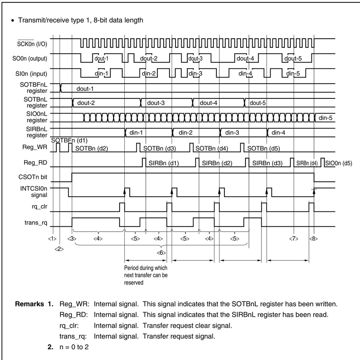
In the case of the continuous transfer mode, two transfer requests are set at the start of the first transfer. Following the INTCSI0n signal, transfer is continued if the SOTBnL register can be written within the next transfer reservation period. If the SOTBnL register cannot be written, transfer ends and the SIRBnL register does not receive the new value of the SIO0nL register.
