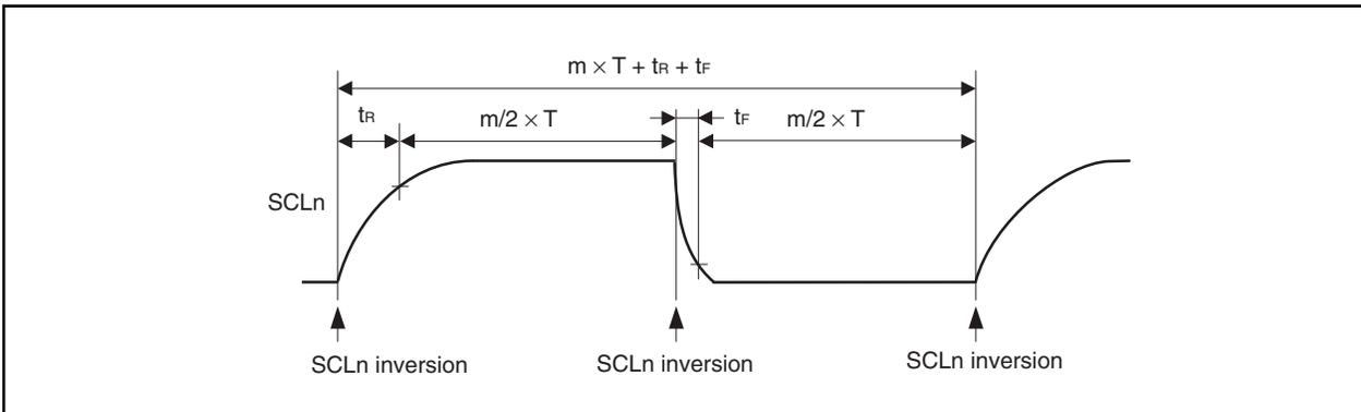
The selection clock is set using a combination of the IICCLn.SMCn, IICCLn.CLn1, and IICCLn.CLn0 bits and the IICXn.CLXn bit.
