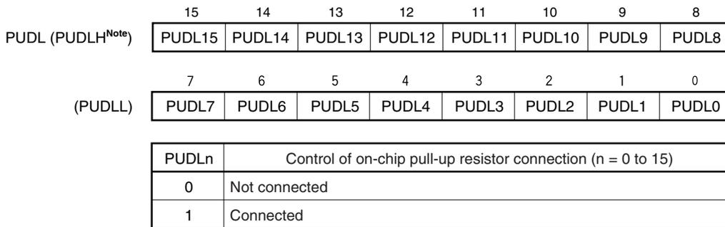
**Note** When reading from or writing to bits 8 to 15 of the PUDL register in 8-bit or 1-bit units, specify these bits as bits 0 to 7 of the PUDLH register.
