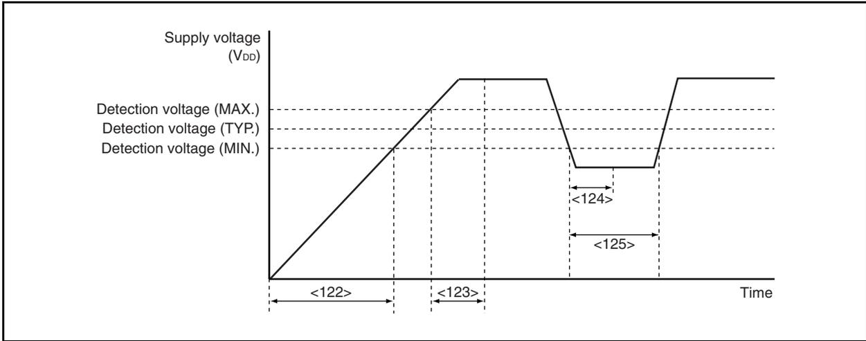
**Low-Voltage Detector Characteristics**
