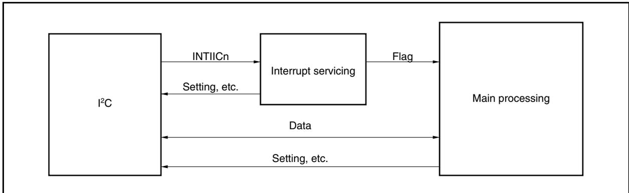
Therefore, the following three flags are prepared so that the data transfer processing can be performed by transmitting these flags to the main processing instead of the INTIICn signal.
