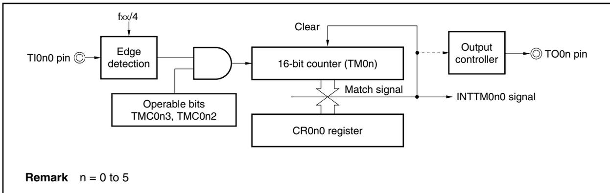
Figure 8-11. Example of Register Settings in External Event Counter Mode
