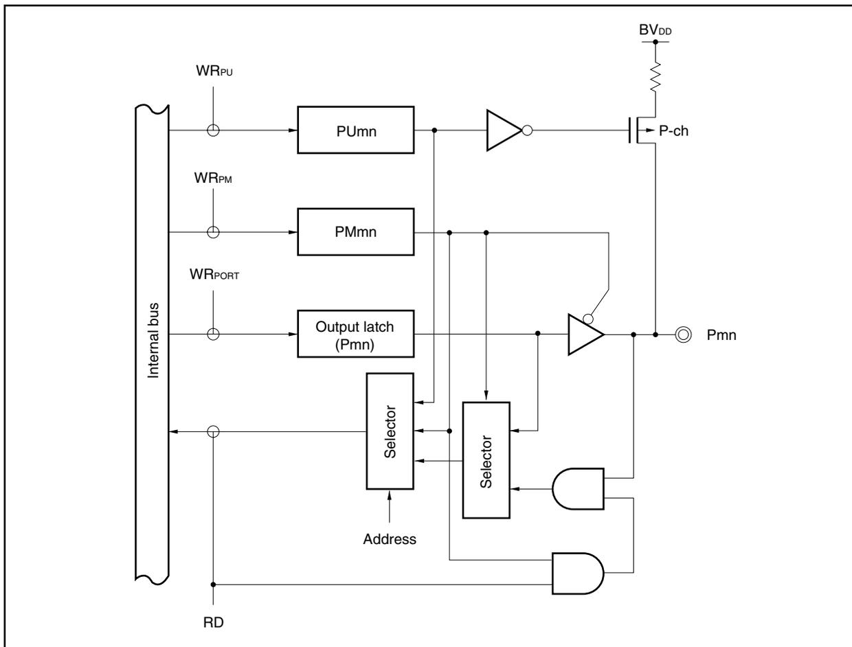
Figure 4-5. Block Diagram of Type C-UA
