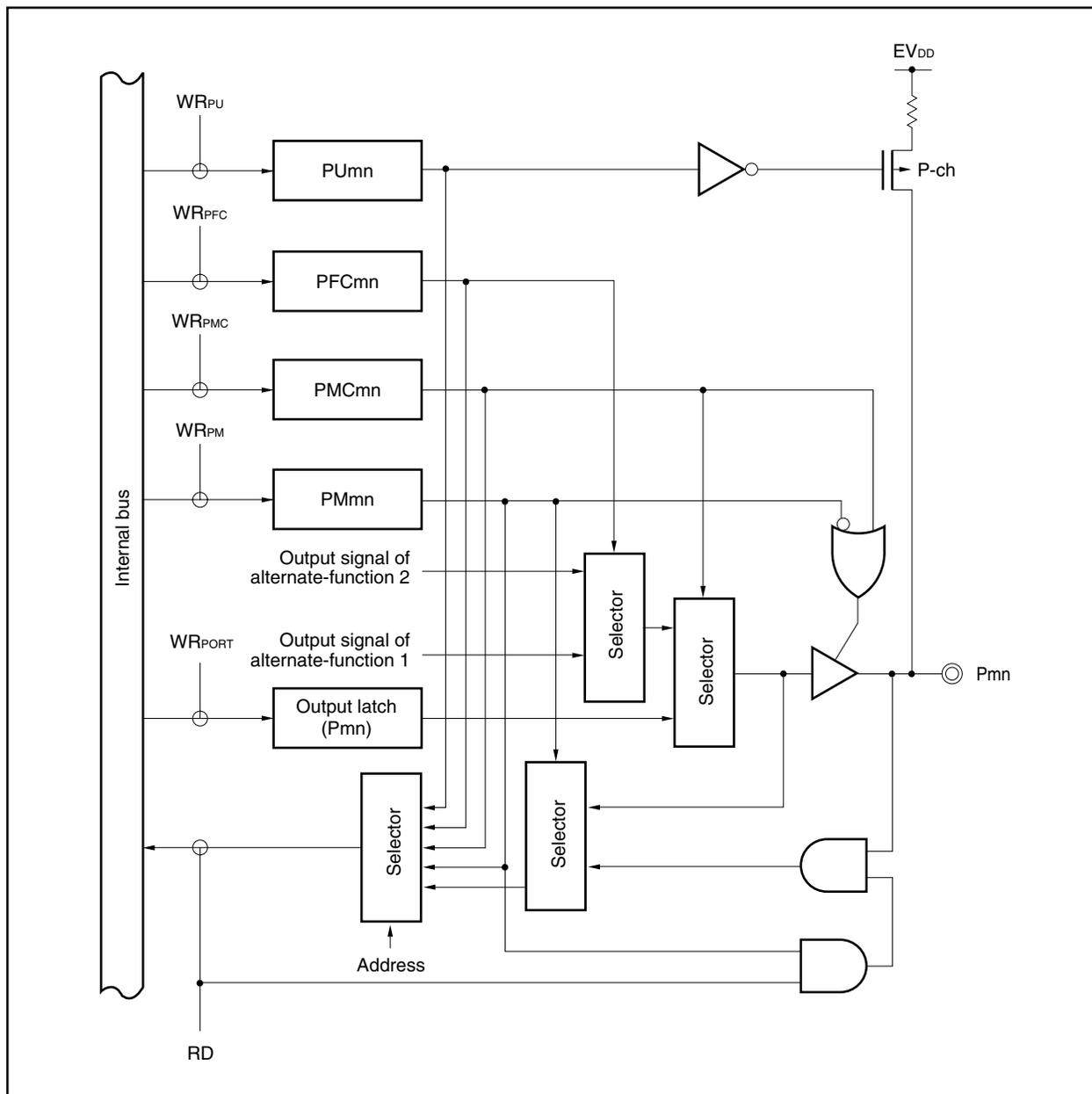
Figure 4-19. Block Diagram of Type E00-UF
