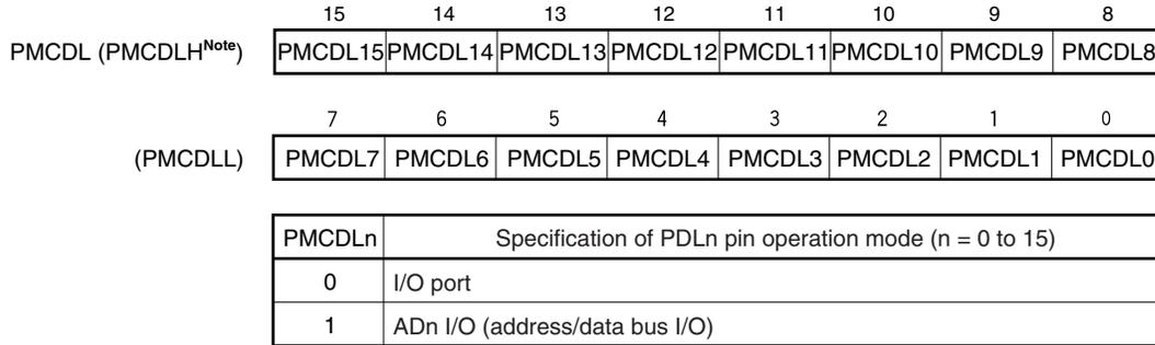
**Note** When reading from or writing to bits 8 to 15 of the PMCDL register in 8-bit or 1-bit units, specify these bits as bits 0 to 7 of the PMCDLH register.
