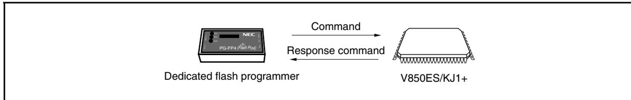
The following shows the commands for flash memory control in the V850ES/KJ1+. All of these commands are issued from the dedicated flash programmer, and the V850ES/KJ1+ performs the processing corresponding to the commands.
