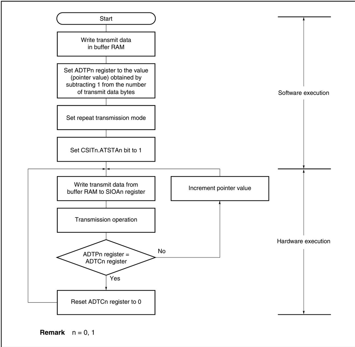
In 6-byte transmission (CSIMAn.ATMn bit = 1, CSIMAn.RXEAn bit = 0, CSIMAn.TXEAn bit = 1, CSIMAn.ATEn bit = 1) in repeat transmission mode, buffer RAM operates as follows.
