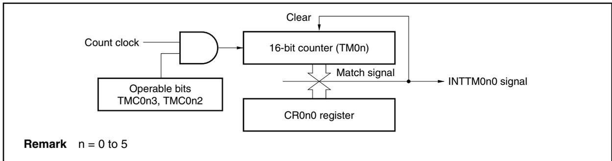
**Figure 8-3. Basic Timing Example of Interval Timer Operation**
