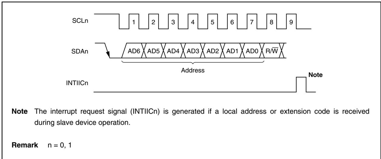
The slave address and the eighth bit, which specifies the transfer direction as described in **19.6.3 Transfer direction specification** below, are together written to the IICn register and are then output. Received addresses are written to the IICn register.
