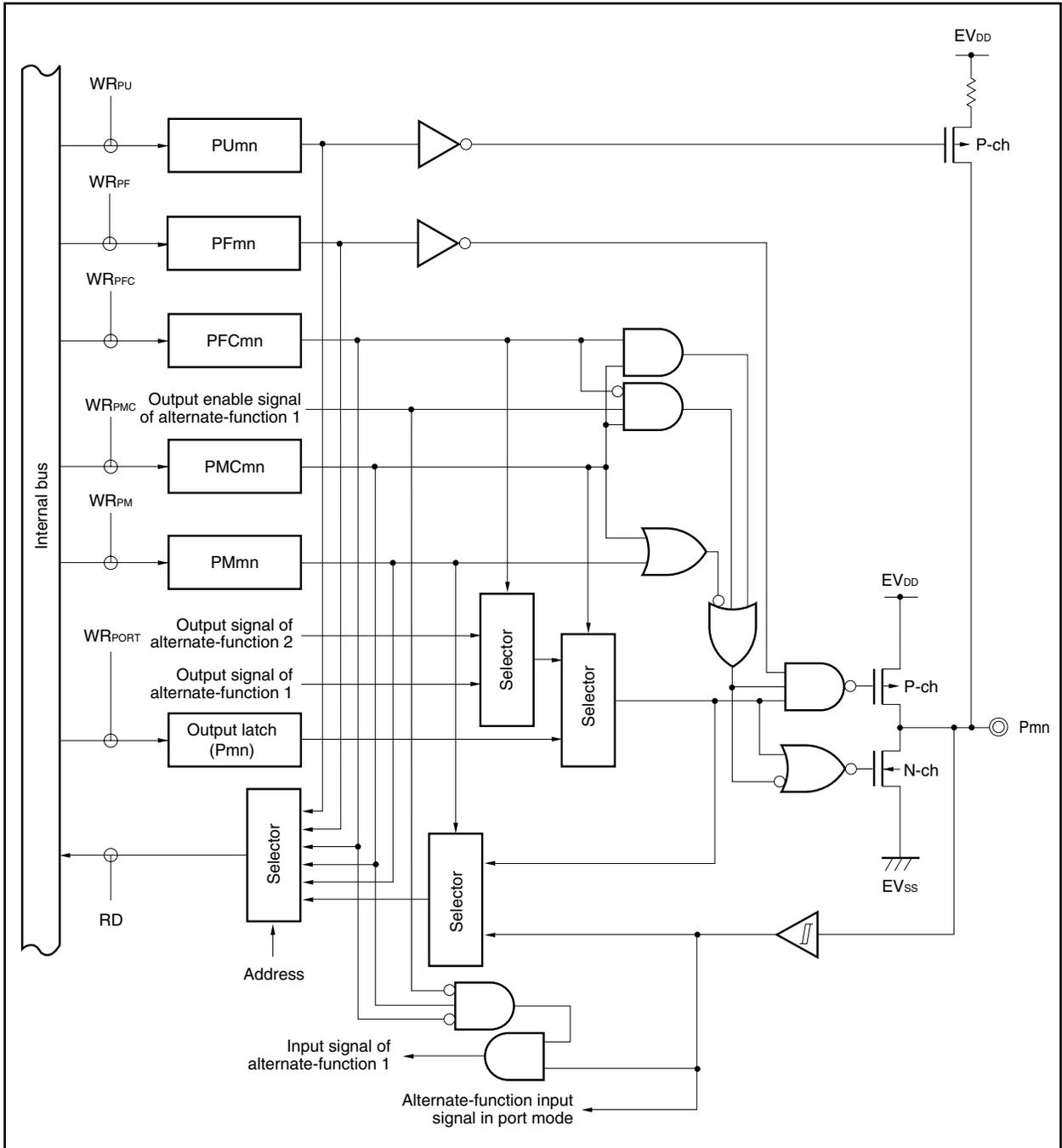
Figure 4-32. Block Diagram of Type G1010-SUL
