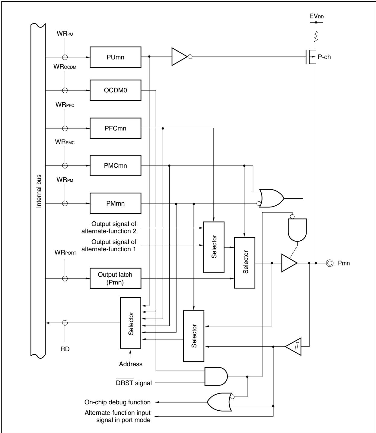
Figure 4-36. Block Diagram of Type OE100-SULT
