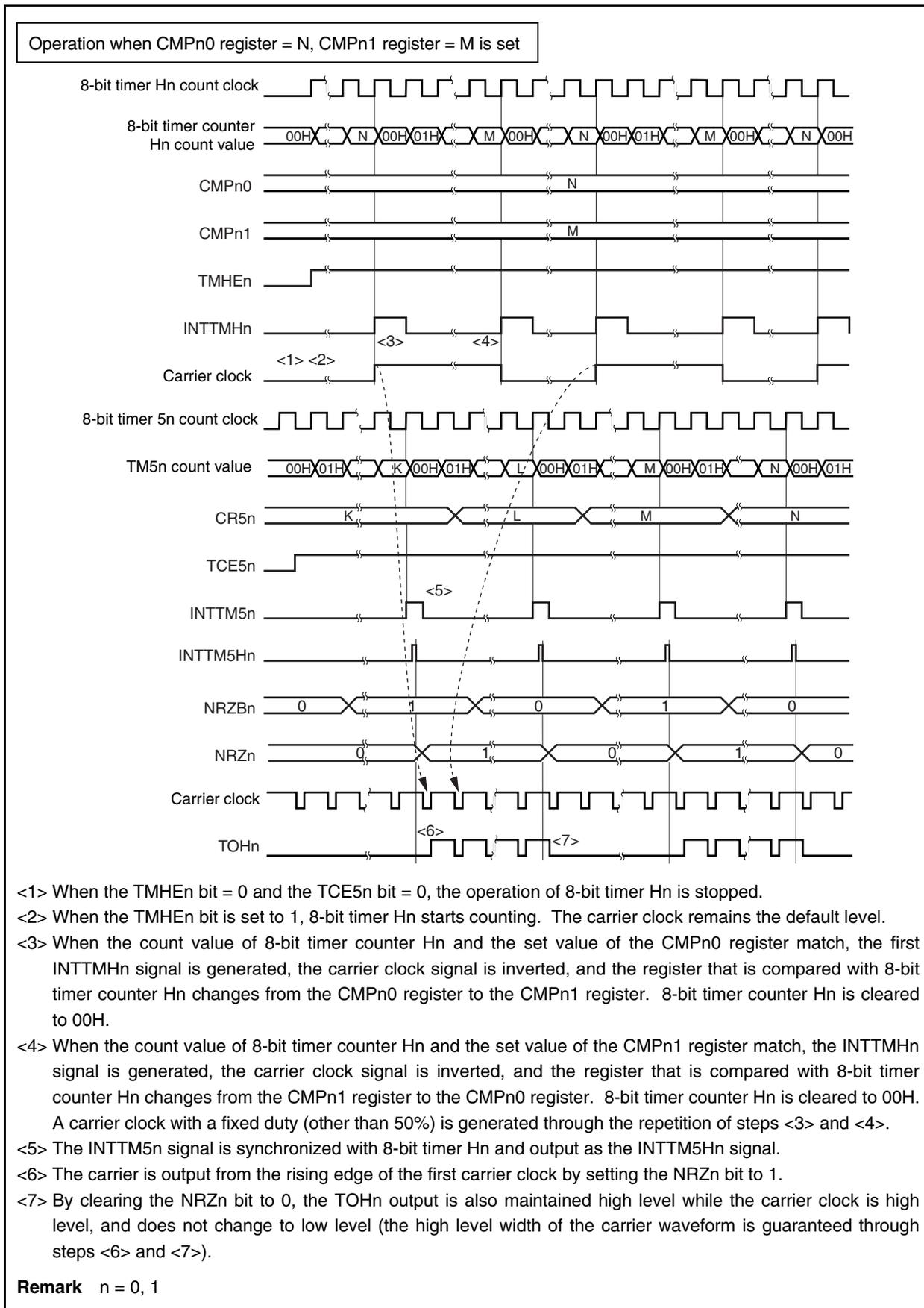
Figure 10-8. Carrier Generator Mode (3/3)
