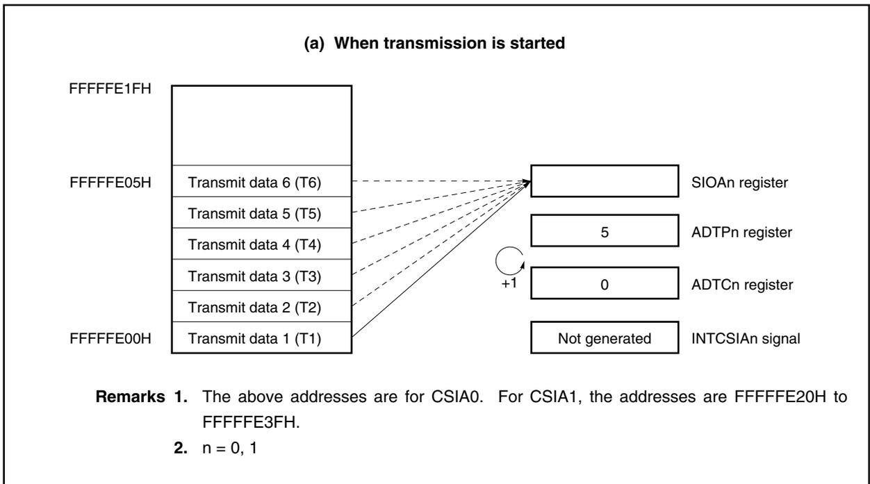
**Figure 18-13. Buffer RAM Operation in 6-Byte Transmission (in Repeat Transmission Mode) (2/2)**
