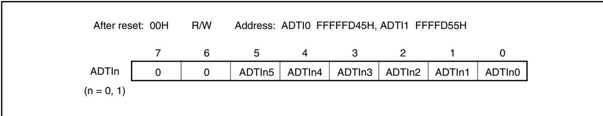
The specified interval time is the transfer clock (specified by the BRGCAn register) multiplied by an integer value.
