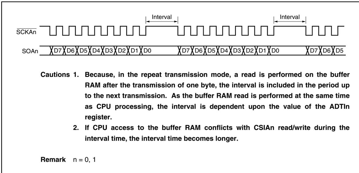
Figure 18-12. Repeat Transmission Mode Flowchart
