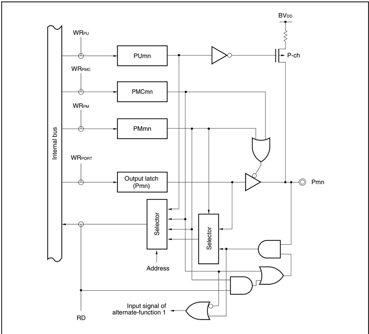
Figure 4-12. Block Diagram of Type D2-SNFH
