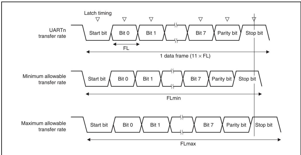
As shown in Figure 16-19, after the start bit is detected, the receive data latch timing is determined according to the counter that was set by the BRGCn register. If all data up to the final data (stop bit) is in time for this latch timing, the data can be received normally.
