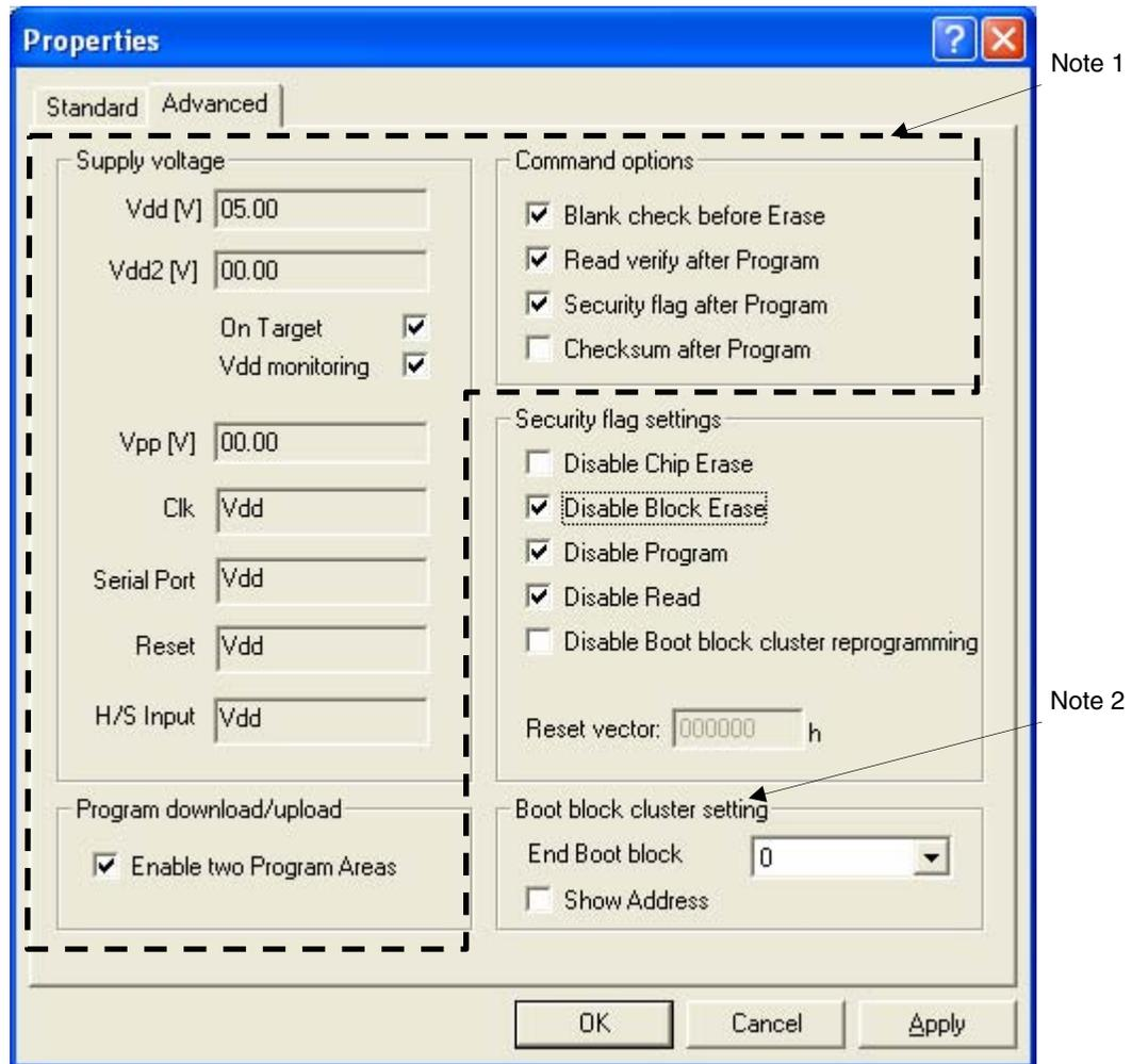
**Notes 1.** Set “Supply voltage”, “Program download/upload”, and “Command options” in broken lines in accordance with the use conditions.
