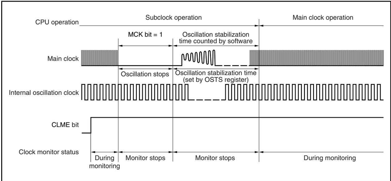
**(d) Operation when CPU operates on internal oscillation clock (CCLS.CCLS bit = 1)**
