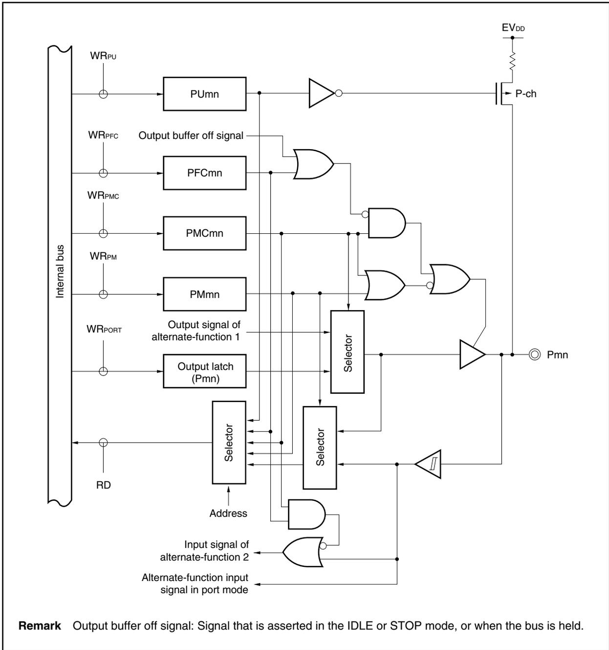
Figure 4-22. Block Diagram of Type E01-SUILZ
