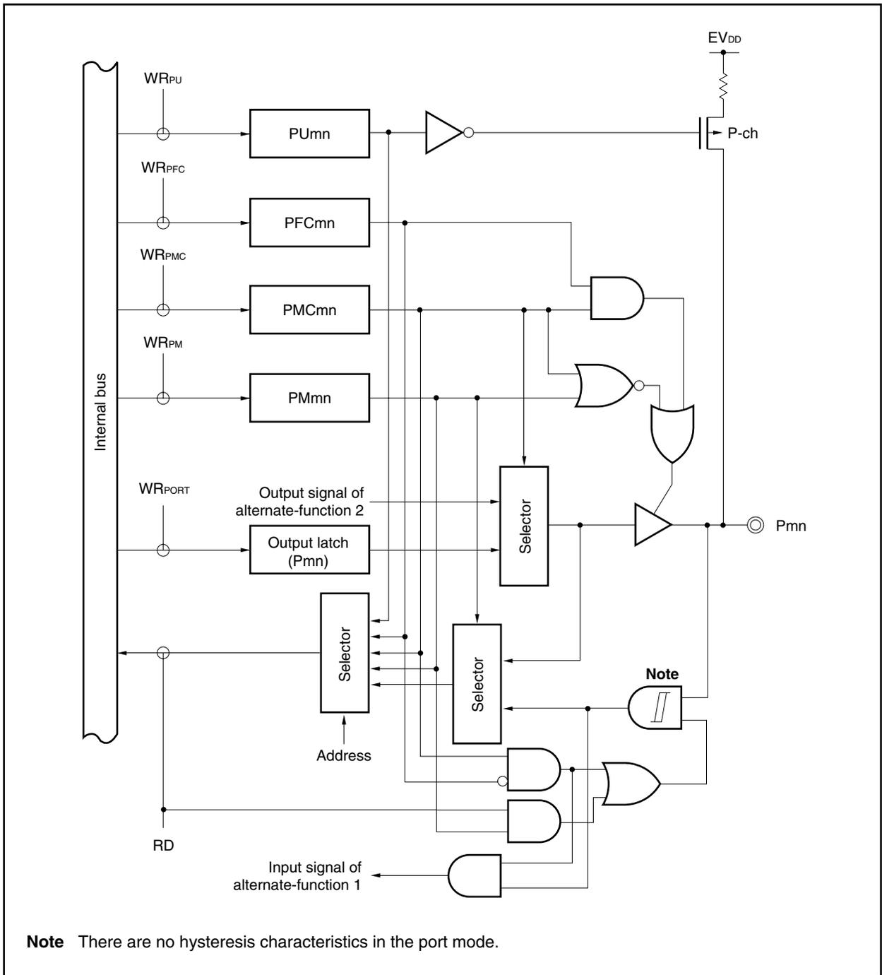
Figure 4-28. Block Diagram of Type E10-SULT
