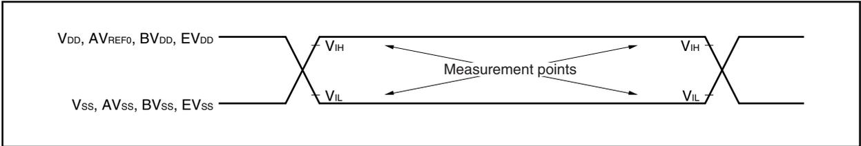
**AC Test Output Measurement Points**
