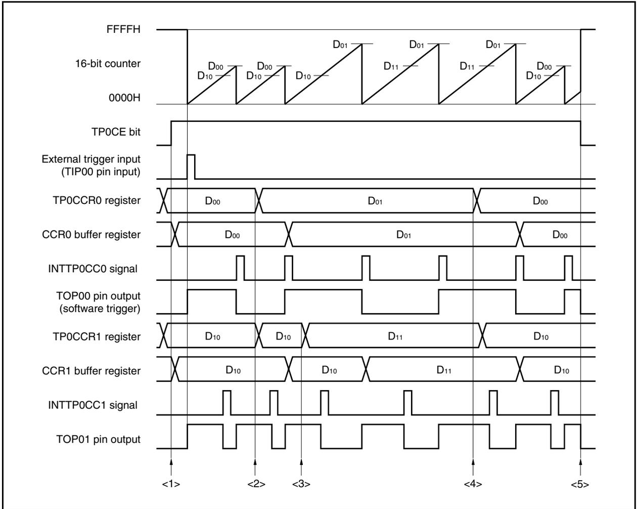
Figure 7-19. Software Processing Flow in External Trigger Pulse Output Mode (2/2)
