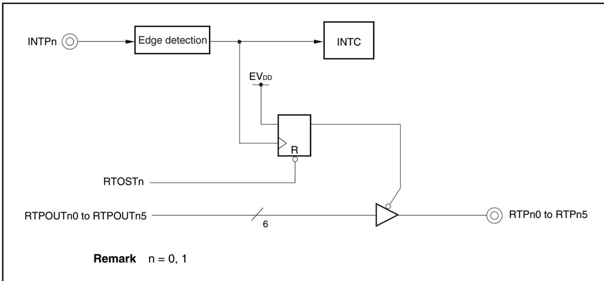
This function is set with the PLLCTL.RTOST1 and PLLCTL.RTOST0 bits.
