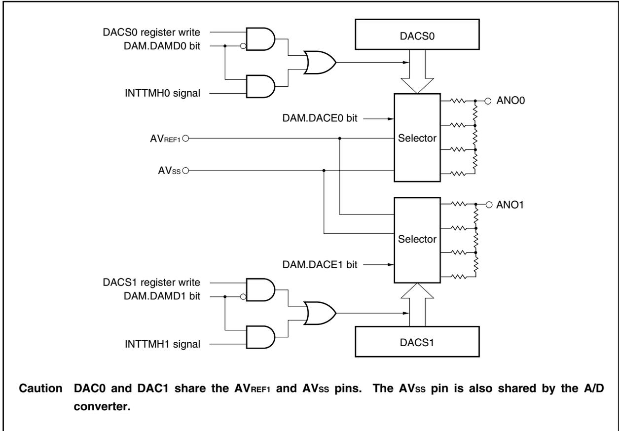
The D/A converter includes the following hardware.
