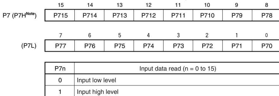
**Note** When reading from bits 8 to 15 of the P7 register in 8-bit or 1-bit units, specify these bits as bits 0 to 7 of the P7H register.
