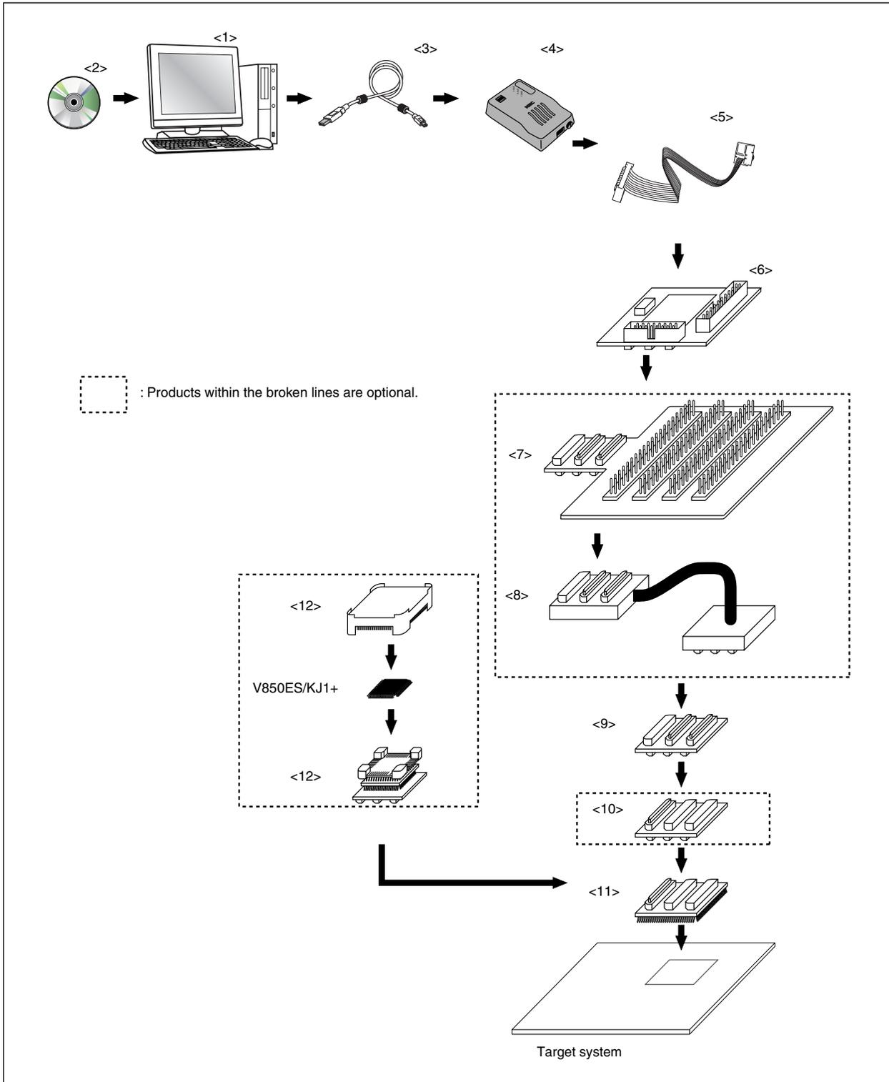
Figure A-5. Example of System Configuration Using QB-V850ESKX1H-DA (Not Using Optional Products)
