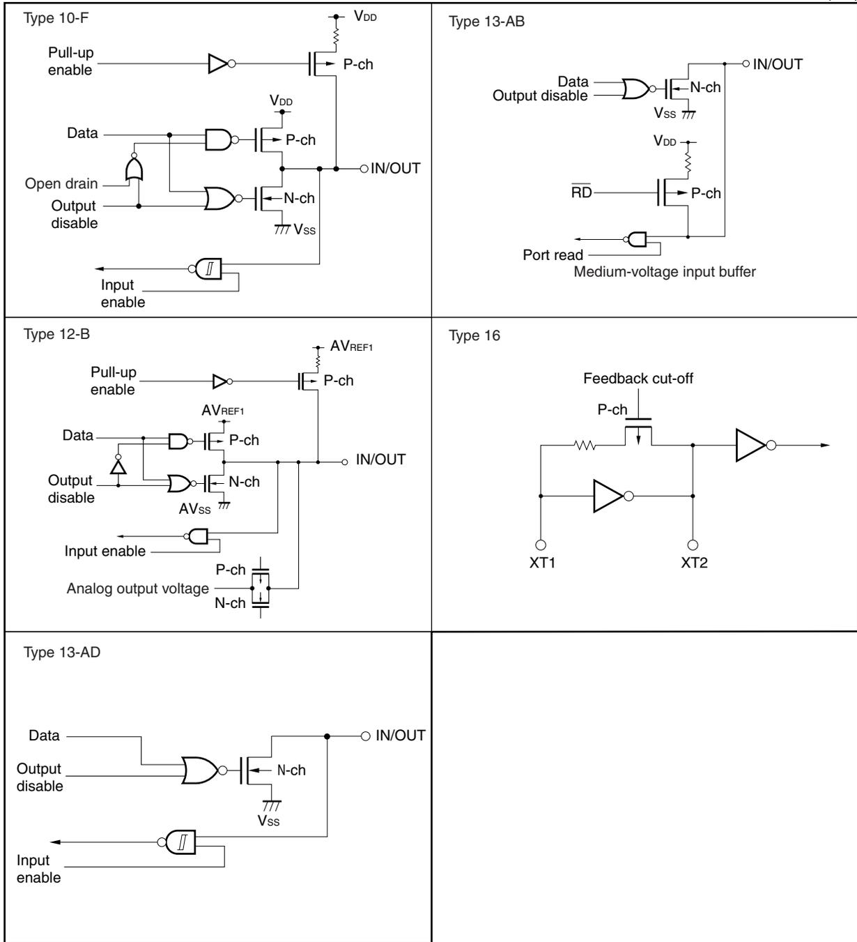
**Remark** Read  $V_{DD}$  as  $EV_{DD}$  or  $BV_{DD}$ . Also, read  $V_{SS}$  as  $EV_{SS}$  or  $BV_{SS}$ .
