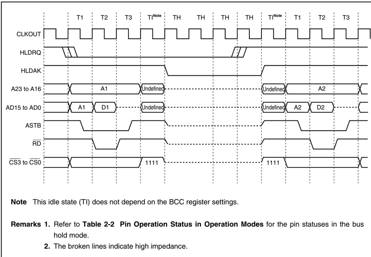
Figure 5-9. Separate Bus Read Timing (Bus Size: 16 Bits, 16-bit Access)
