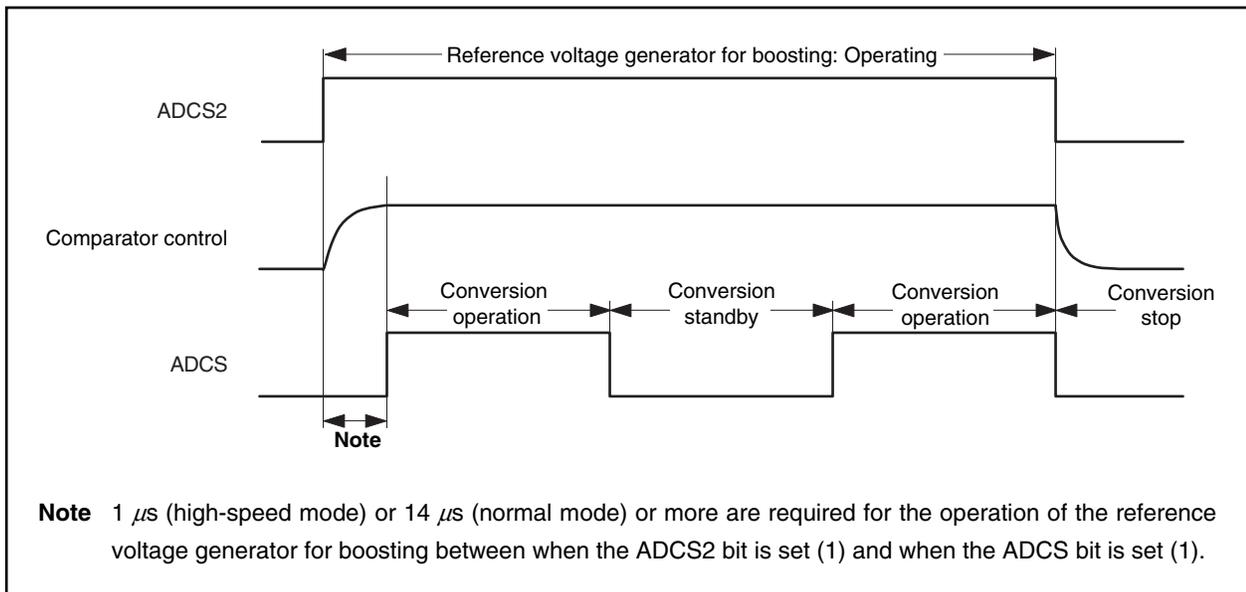
**Note** 1  $\mu$ s (high-speed mode) or 14  $\mu$ s (normal mode) or more are required for the operation of the reference voltage generator for boosting between when the ADCS2 bit is set (1) and when the ADCS bit is set (1).
