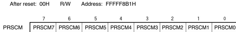
**Caution** Do not rewrite the PRSCM register while interval timer BRG is operating (PRSM.BGCE bit = 1). Set the PRSCM register before setting (1) the BGCE bit.
