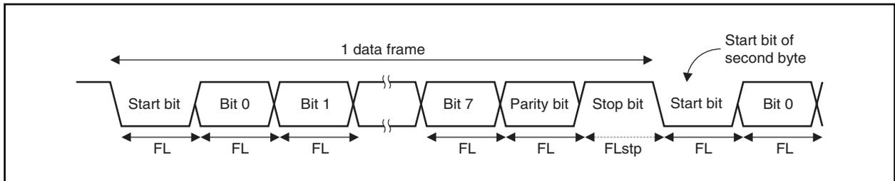
Representing the 1-bit data length by FL, the stop bit length by FLstp, and the base clock frequency by  $f_{uCLK}$  yields the following equation.
