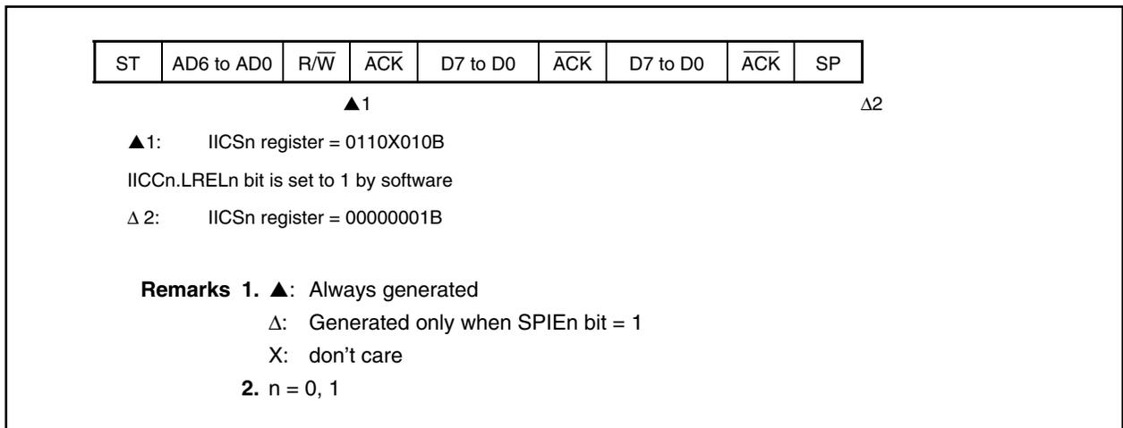
**(3) When arbitration loss occurs during data transfer****<1> When IICSn.WTIMn bit = 0**
