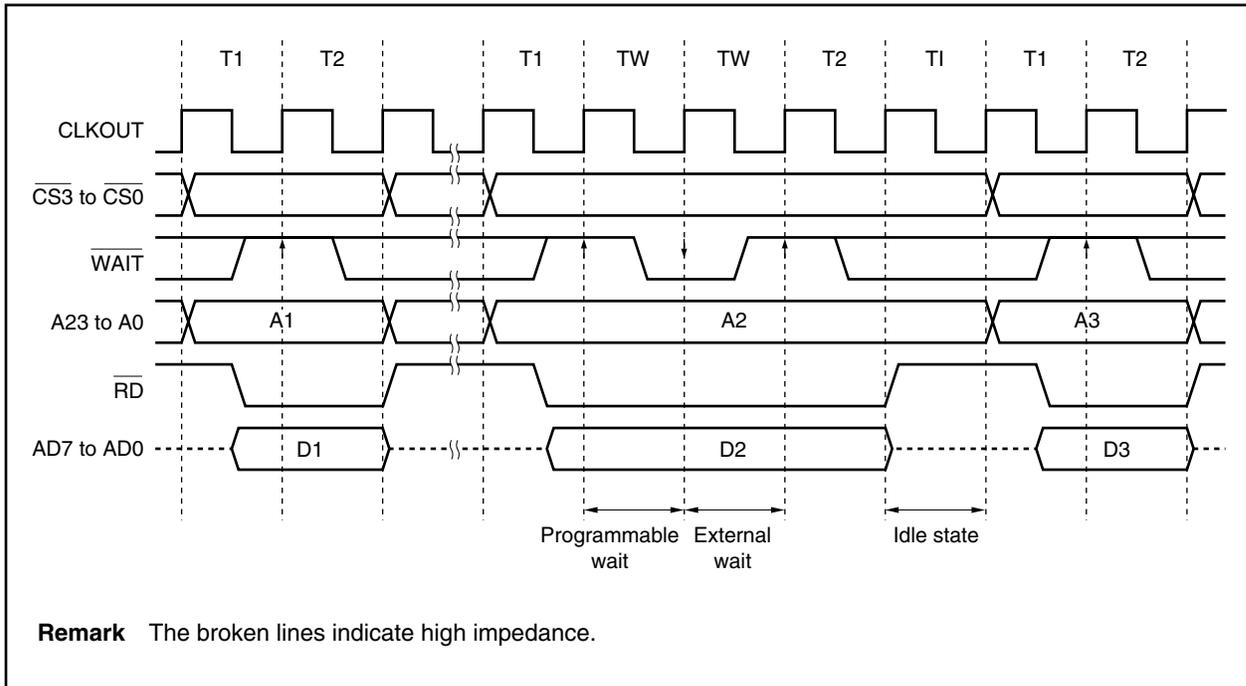
Figure 5-11. Separate Bus Write Timing (Bus Size: 16 Bits, 16-bit Access)
