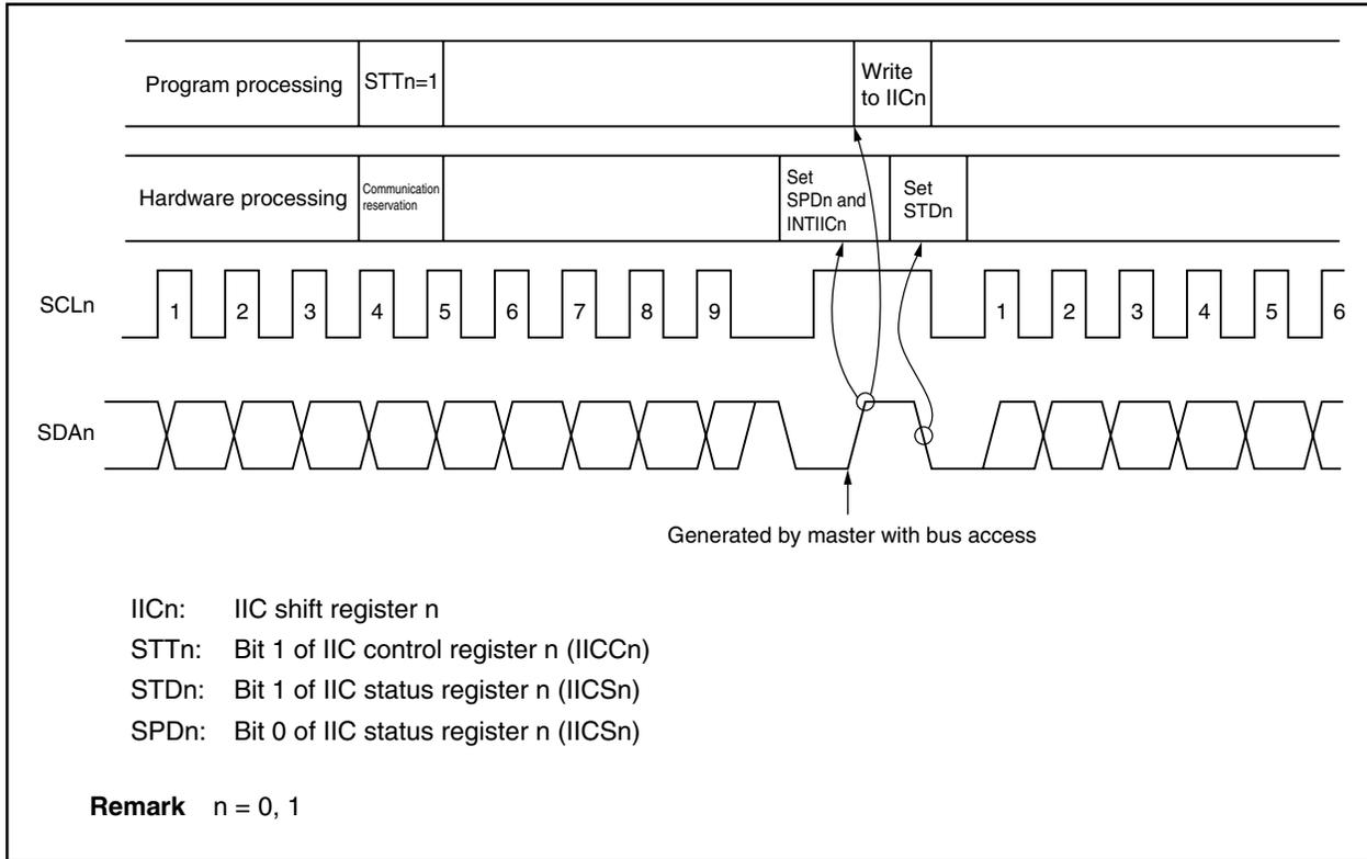
Communication reservations are accepted via the following timing. After the IICSn.STDn bit is set to 1, a communication reservation can be made by setting the IICCn.STTn bit to 1 before a stop condition is detected (n = 0, 1).
