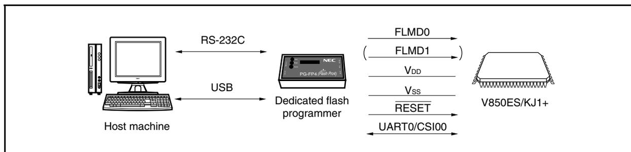
A host machine is required for controlling the dedicated flash programmer.
