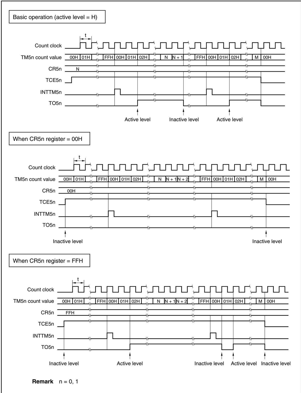
(b) Operation based on CR5n register transitions
