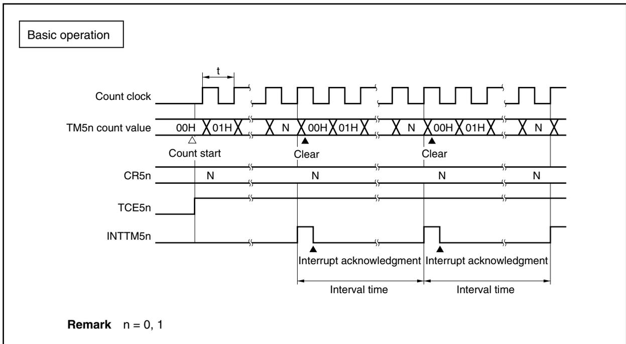
Figure 9-2. Timing of Interval Timer Operation (2/2)
