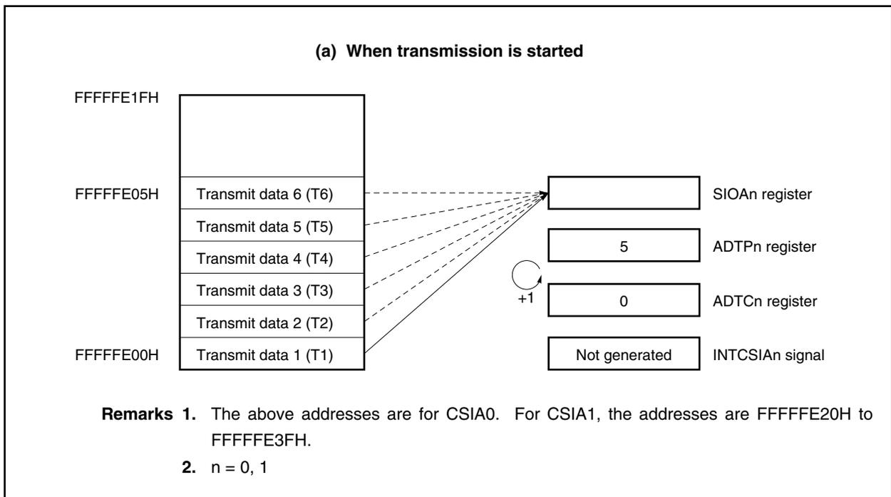
**Figure 18-10. Buffer RAM Operation in 6-Byte Transmission
