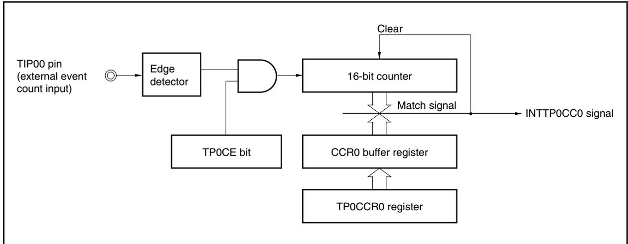
Figure 7-10. Basic Timing in External Event Count Mode
