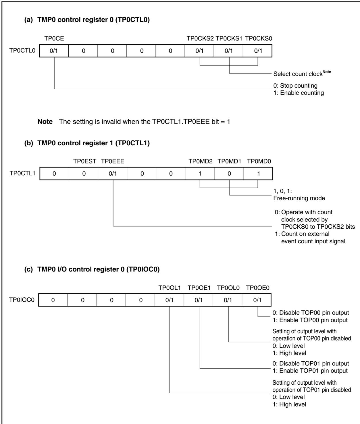
Figure 7-31. Register Setting in Free-Running Timer Mode (2/2)
