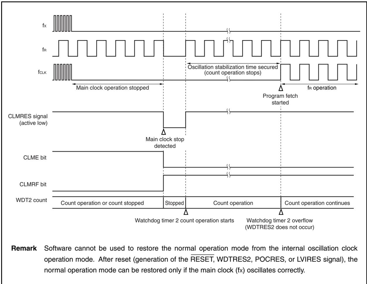
Table 25-3. Operation Status in Internal Oscillation Clock Operation Mode
