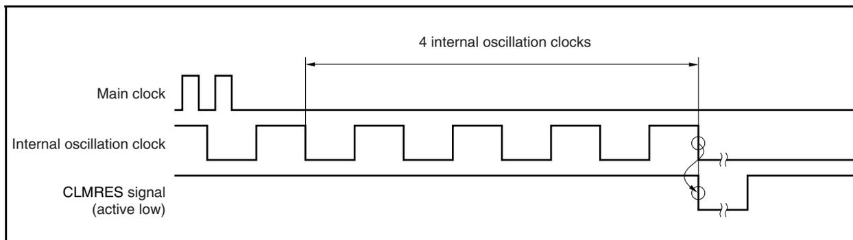
**(b) Operation in STOP mode and after STOP mode is released**
