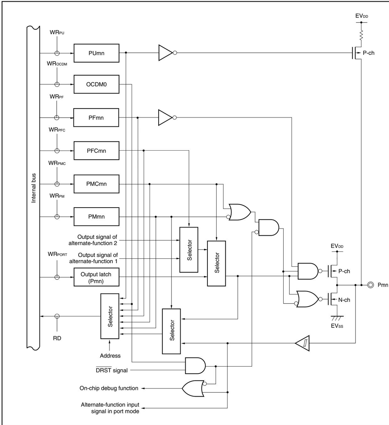
Figure 4-35. Block Diagram of Type OE001-SUT
