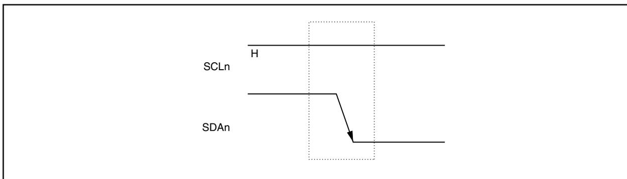
A start condition is generated when the IICn.STTn bit is set to 1 after a stop condition has been detected (IICn.SPdn bit = 1). When a start condition is detected, the IICn.STDn bit is set to 1.
