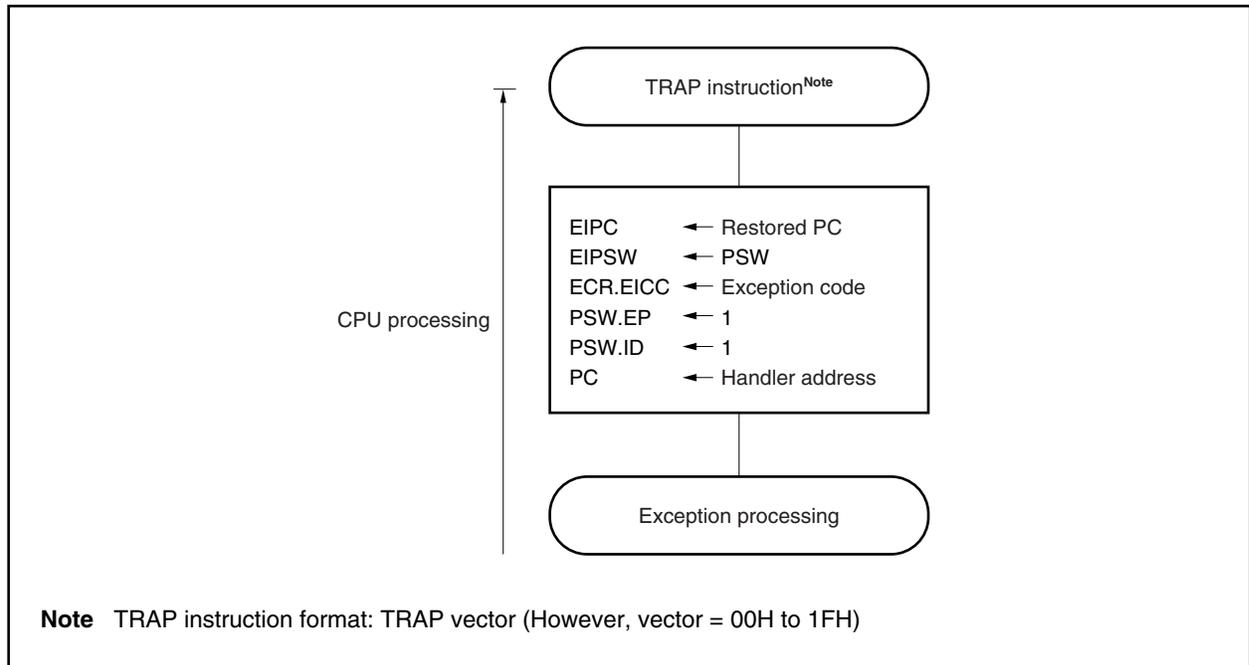
The handler address is determined by the operand (vector) of the TRAP instruction. If the vector is 00H to 1FH, the handler address is 00000040H, and if the vector is 10H to 1FH, the handler address is 00000050H.
