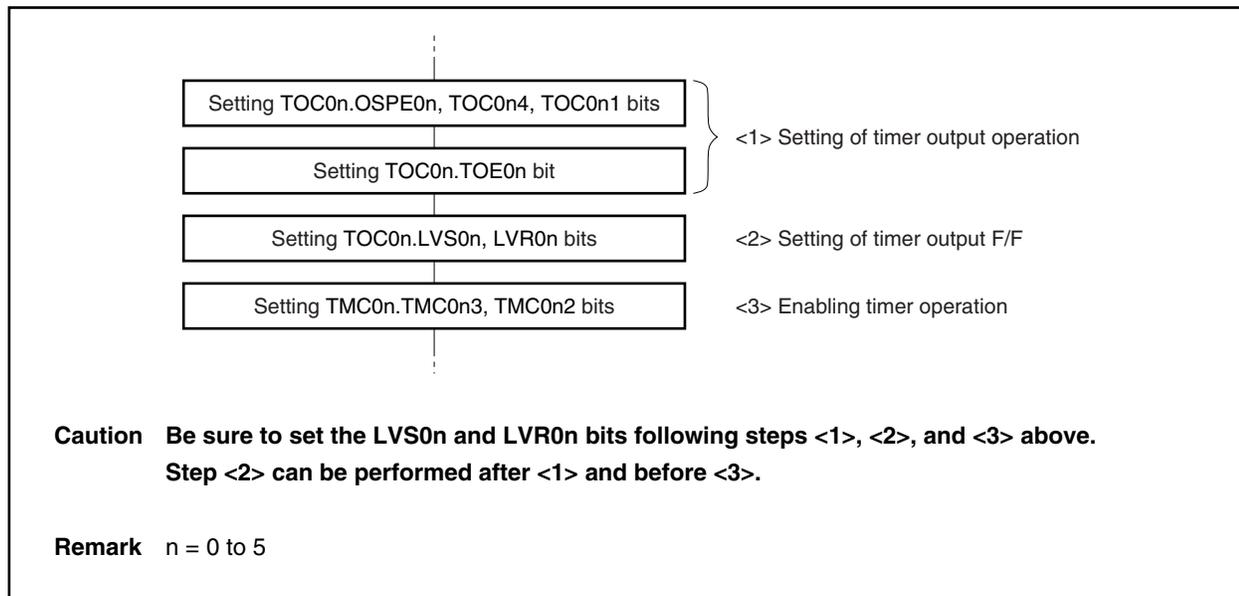
**Figure 8-45. Timing Example of LVR0n and LVS0n Bits**
