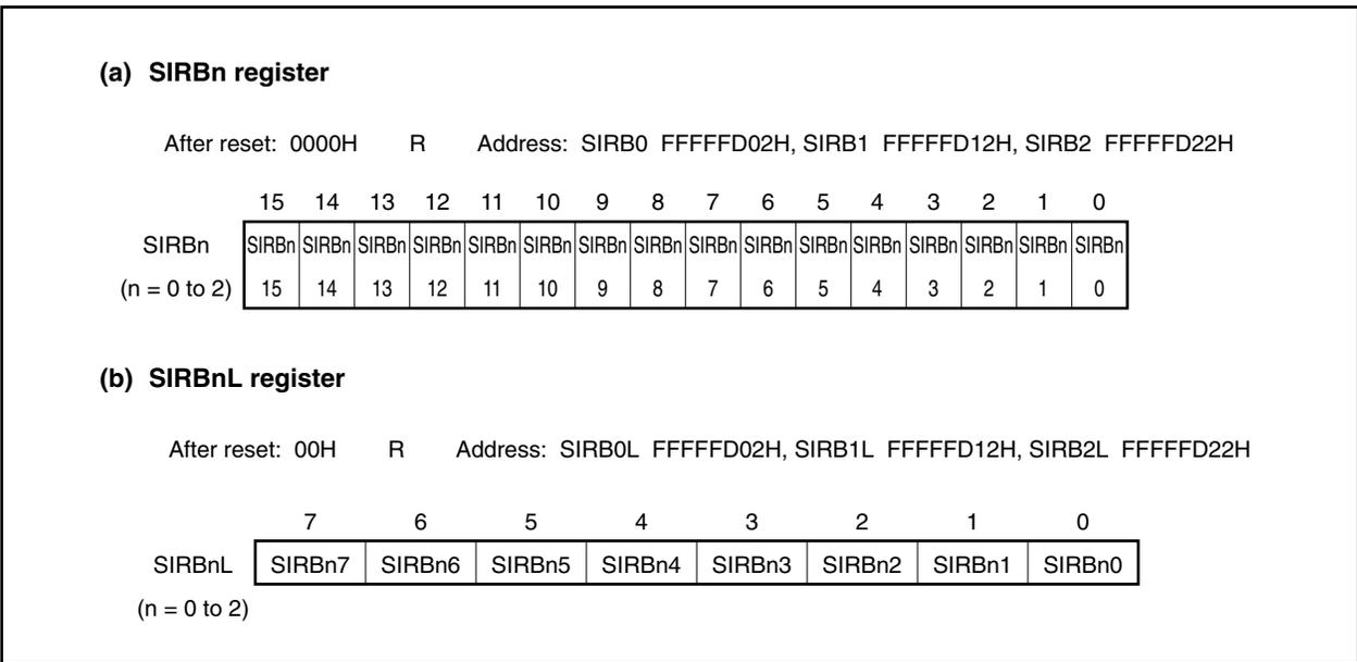
**(4) Clocked serial interface read-only receive buffer registers n, nL (SIRBEn, SIRBEnL)**
