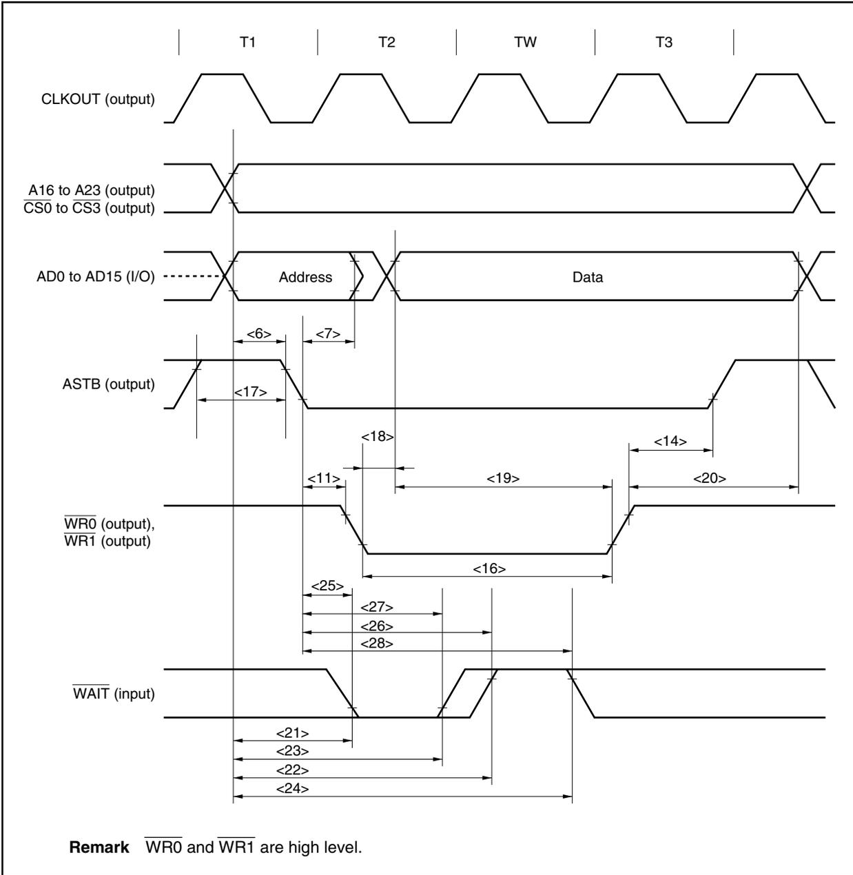
**(b) Read/write cycle (CLKOUT synchronous): In multiplex bus mode**
