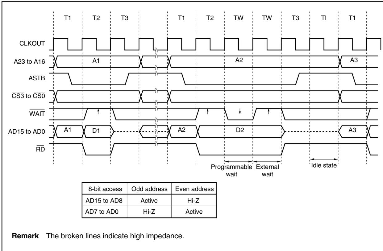
Figure 5-5. Multiplex Bus Read Timing (Bus Size: 8 Bits)
