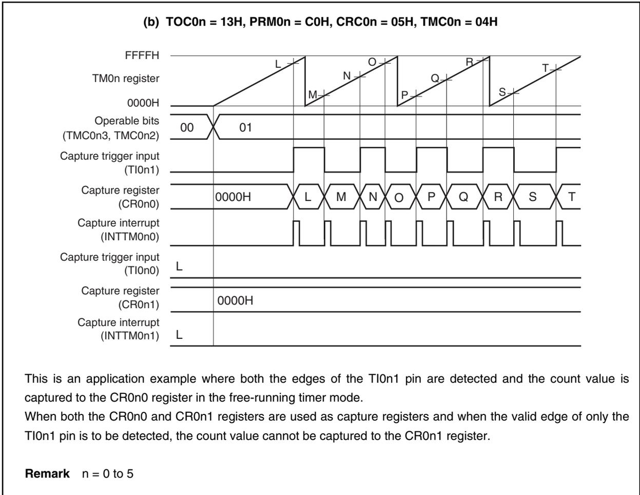
Figure 8-29. Example of Register Settings in Free-Running Timer Mode (1/2)
