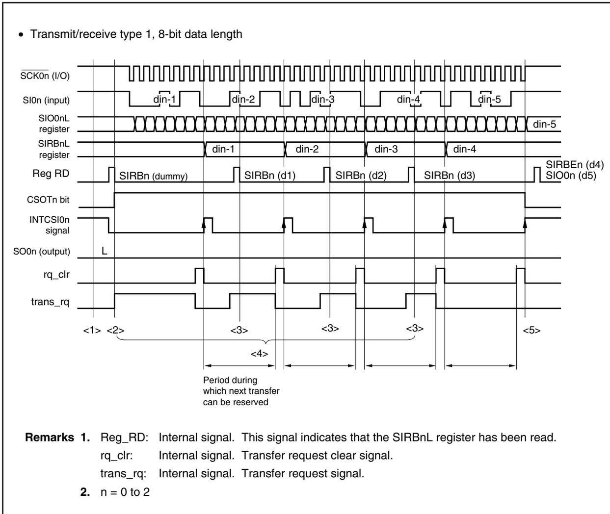
In the case of the continuous transfer mode, two transfer requests are set at the start of the first transfer. Following the INTCSI0n signal, transfer is continued if the SIRBnL register can be read within the next transfer reservation period. If the SIRBnL register cannot be read, transfer ends and the SIRBnL register does not receive the new value of the SIO0nL register.
