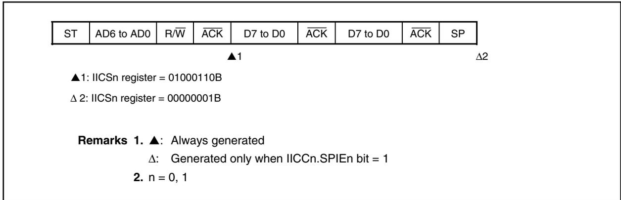
**(2) When arbitration loss occurs during transmission of extension code**
