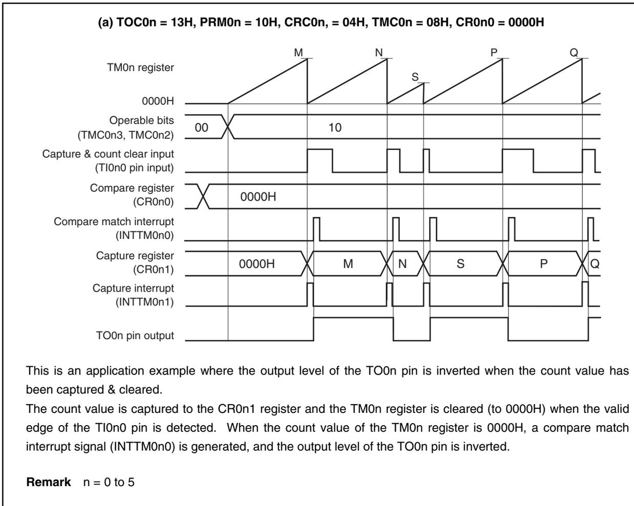
**Figure 8-16. Timing Example of Clear & Start Mode Entered by TI0n0 Pin Valid Edge Input (CR0n0 Register: Compare Register, CR0n1 Register: Capture Register) (2/2)**
