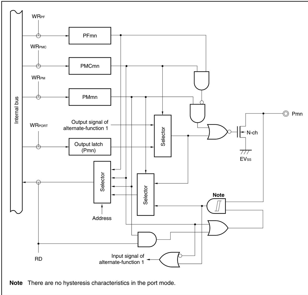
Figure 4-13. Block Diagram of Type D2-SUFL
