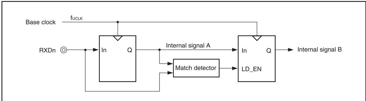
**Figure 16-13. Timing of RXDn Signal Judged as Noise**
