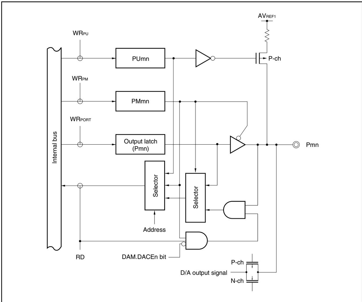
Figure 4-6. Block Diagram of Type D0-U
