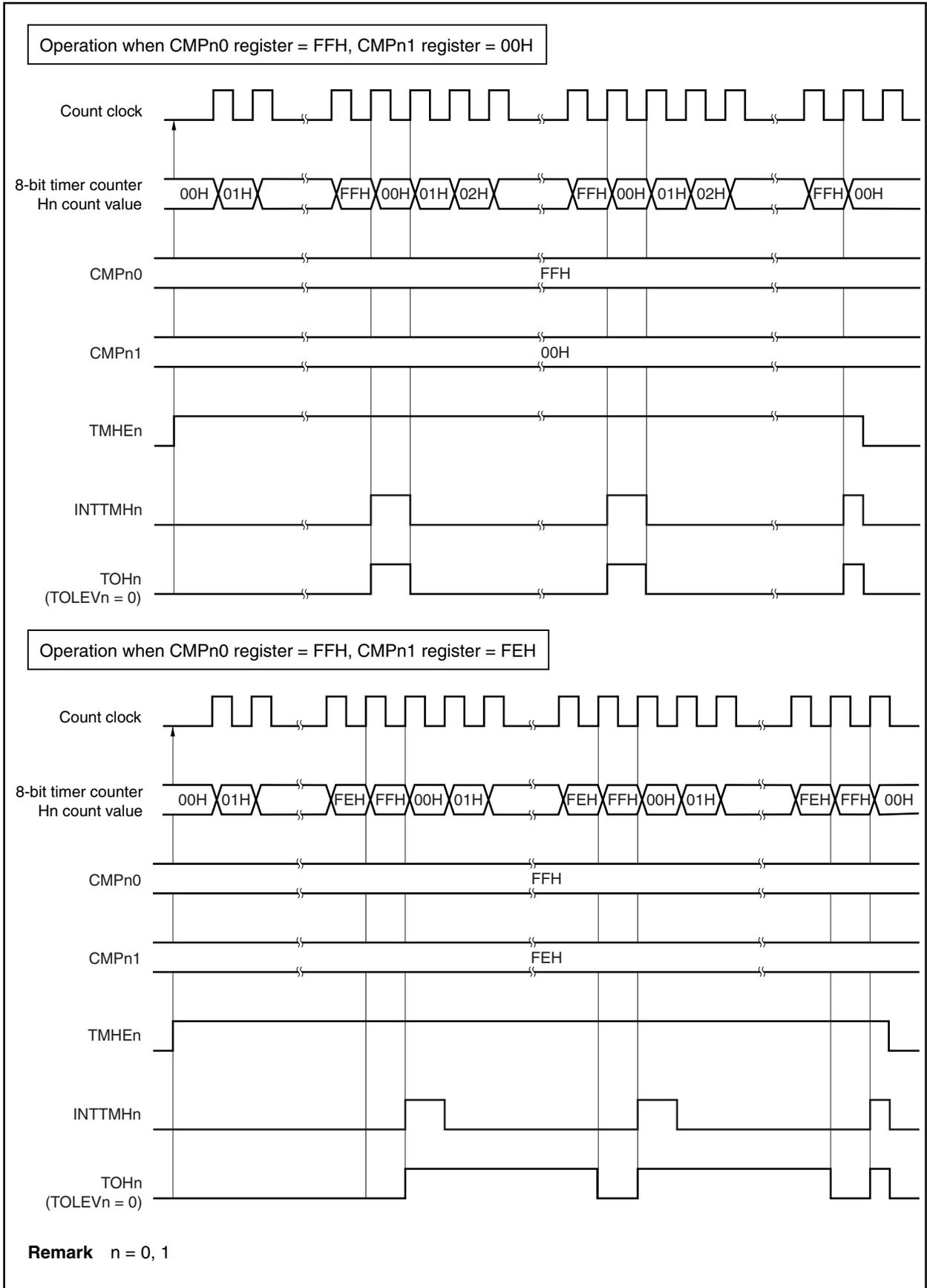
Figure 10-5. Operation Timing in PWM Output Mode (3/4)
