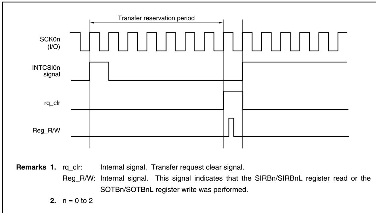
(ii) **In case of conflict between transmission/reception completion interrupt request signal (INTCSI0n) generation and register access**
