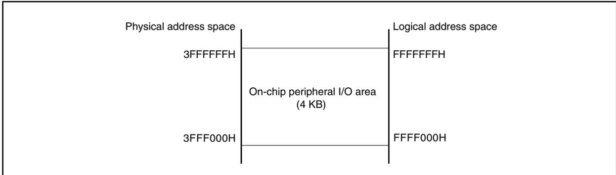
Peripheral I/O registers assigned with functions such as on-chip peripheral I/O operation mode specification and state monitoring are mapped to the on-chip peripheral I/O area. Program fetches are not allowed in this area.
