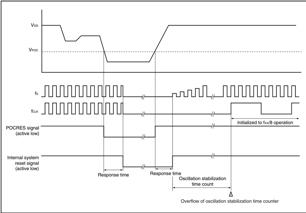
Figure 24-8. Reset Timing on Power Application
