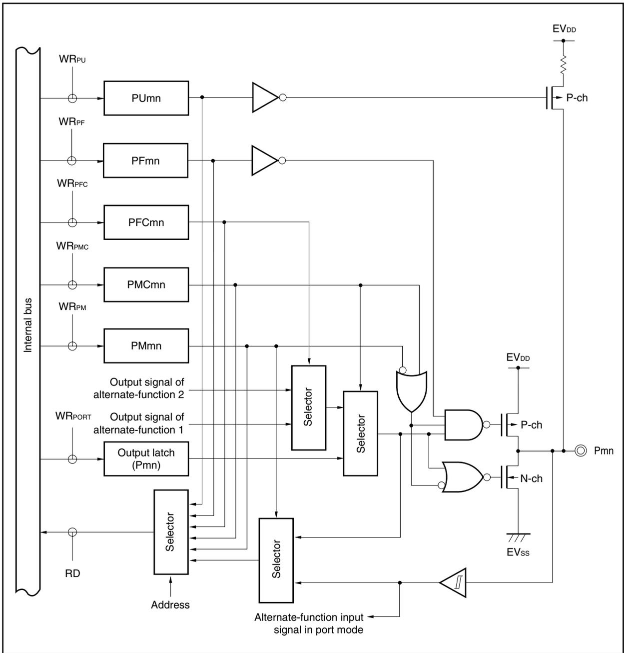
Figure 4-16. Block Diagram of Type E00-SUT
