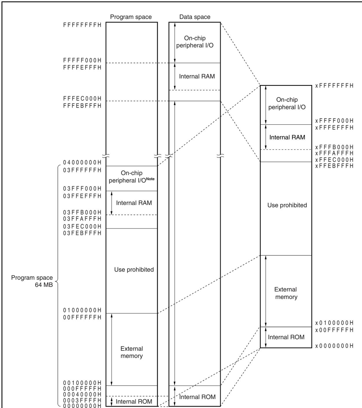
**Note** Access to this area is prohibited. To access the on-chip peripheral I/O in this area, specify addresses FFFF000H to FFFFFFFFH.
