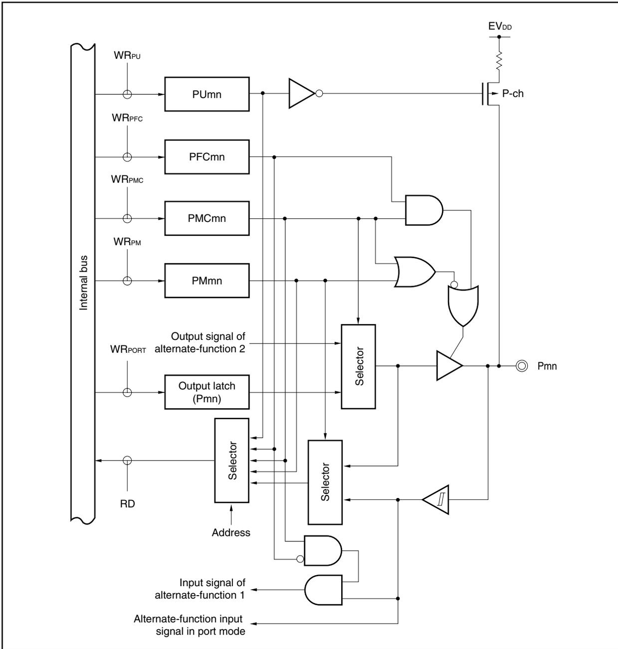
Figure 4-30. Block Diagram of Type E12-SUFHH
