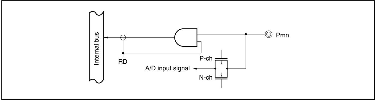
Figure 4-3. Block Diagram of Type C-N
