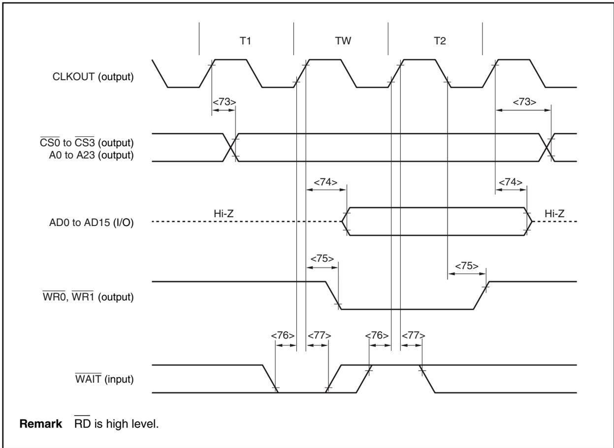
**(3) Bus hold****(a) CLKOUT asynchronous**
