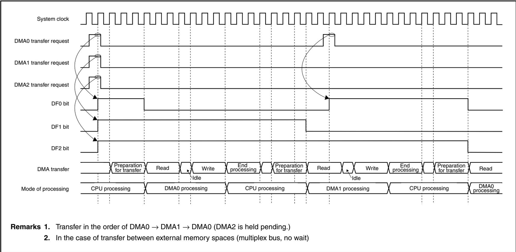
Figure 20-3. Period in Which DMA Transfer Request Is Ignored (1)
