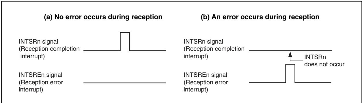
**Figure 16-11. When Reception Error Interrupt Request Signal Is Included in INTSRn Signal (ISRMn Bit = 1)**
