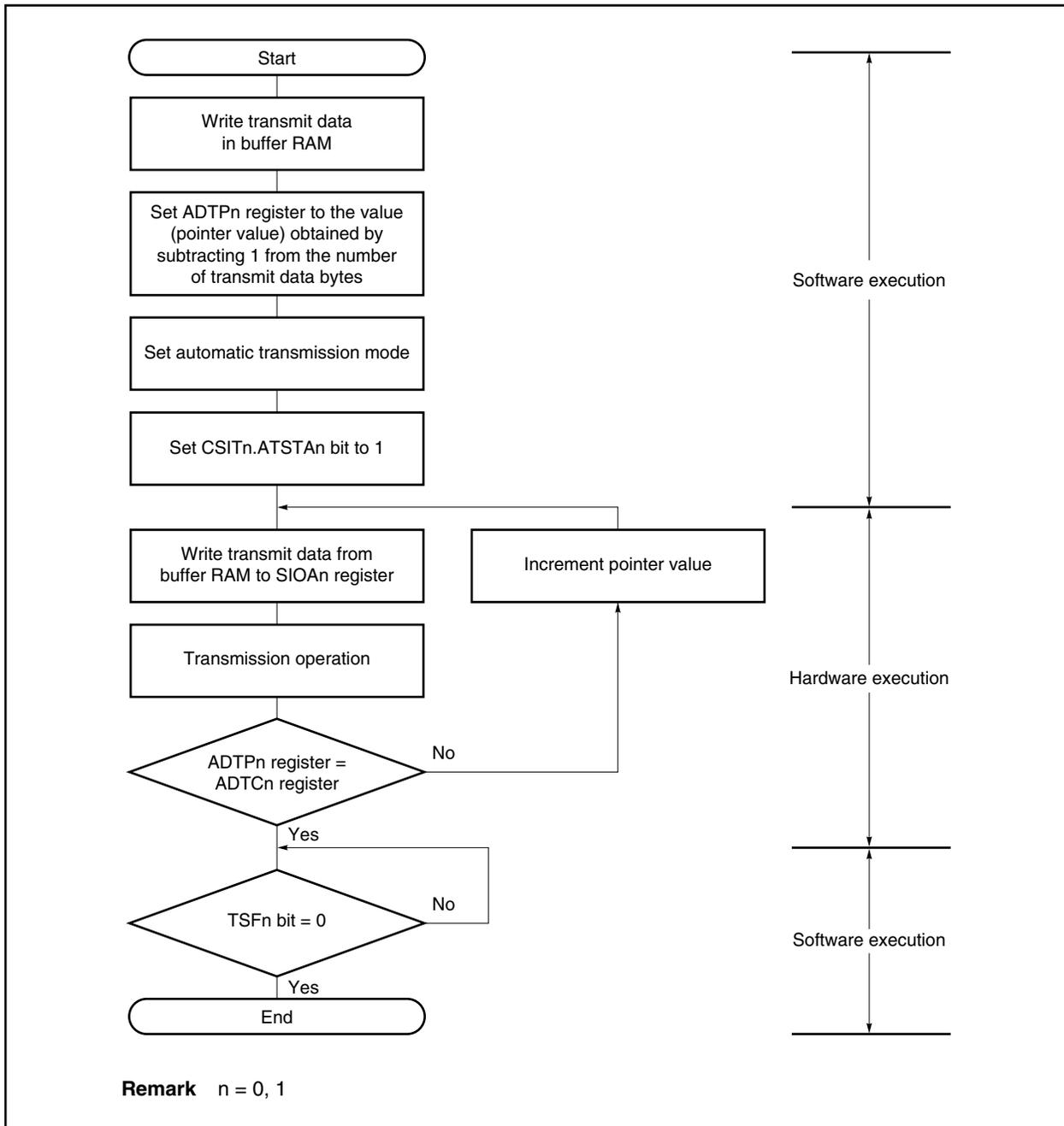
In 6-byte transmission (CSIMAn.ATMn bit = 0, CSIMAn.RXEAn bit = 0, CSIMAn.TXEAn bit = 1, CSIMAn.ATEn bit = 1) in automatic transmission mode, buffer RAM operates as follows.
