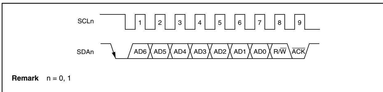
When the local address is received,  $\overline{\text{ACK}}$  is automatically generated regardless of the value of the ACKEn bit. No  $\overline{\text{ACK}}$  is generated if the received address is not a local address (NACK).
