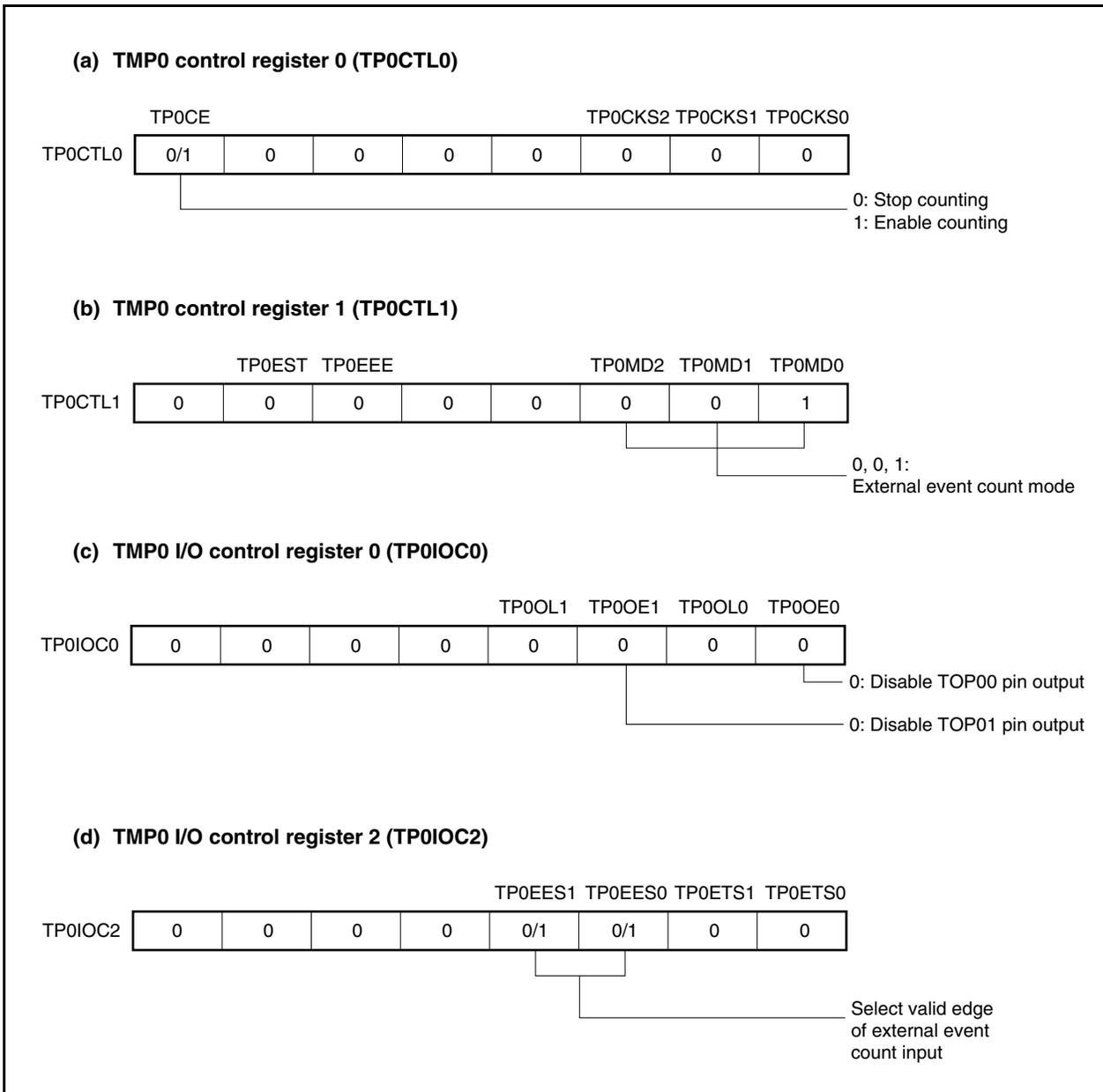
Figure 7-11. Register Setting for Operation in External Event Count Mode (2/2)
