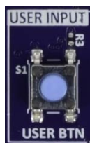
Figure 16. User Switch (S1) on Target Board
