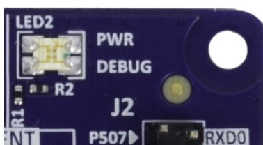
Figure 10. LED2 on Target Board (Top Side)
