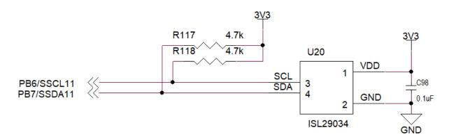
Figure 5-15. Light Sensor Connection Diagram
