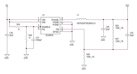
Figure 5-3. 3.3 V Power Supply Circuit
