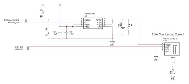
Figure 5-11. USB Host Interface Connection Diagram
