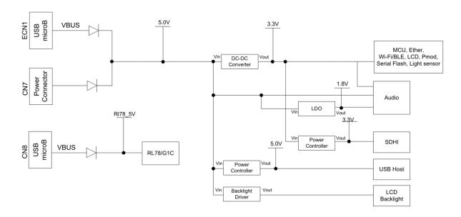
Figure 5-1. RX72N Envision Kit Power Supply System Diagram
