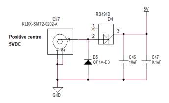
Figure 5-2. CN7 External Power Supply Connector Circuit
