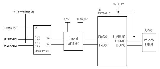
Figure 5-6. USB Serial Interface
