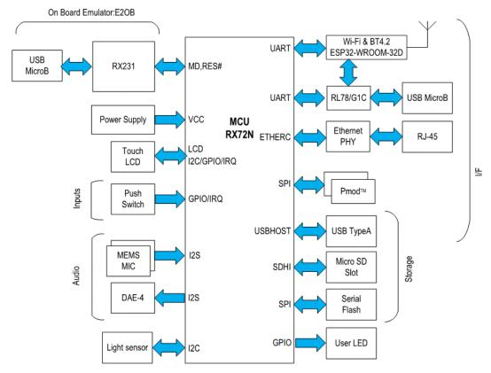
Figure 1-1. Block Diagram
