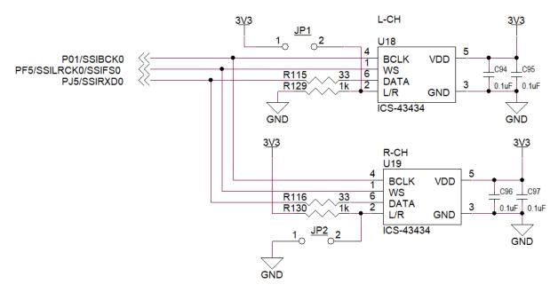
Figure 5-14. MEMS Microphone Connection Diagram
