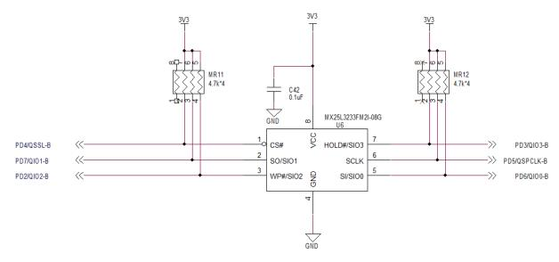
Figure 5-12. Serial Flash Connection Diagram
