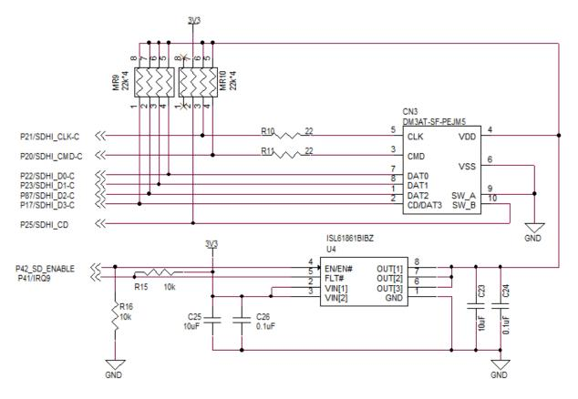
Figure 5-10. microSD Slot Connection Diagram
