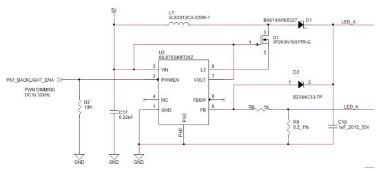
Figure 5-4. LCD Backlight Power Supply Circuit
