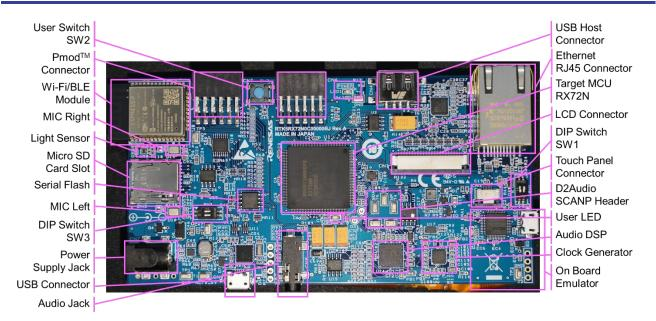
Figure 2-3. External View of Component Side (without LCD)
