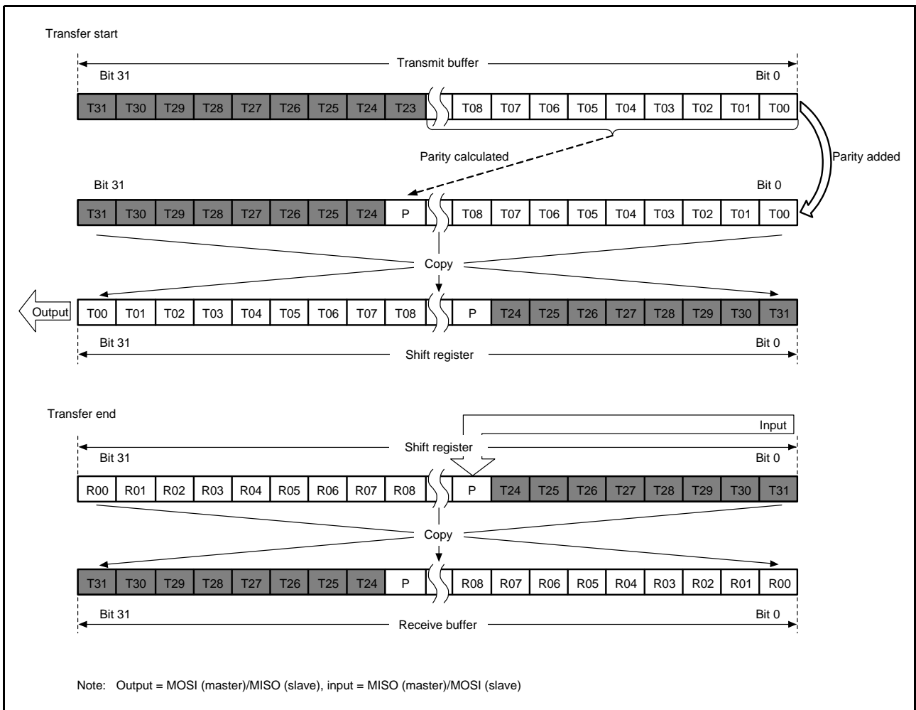
Figure 32.21 LSB First Transfer (24-Bit Data, Parity Enabled)
