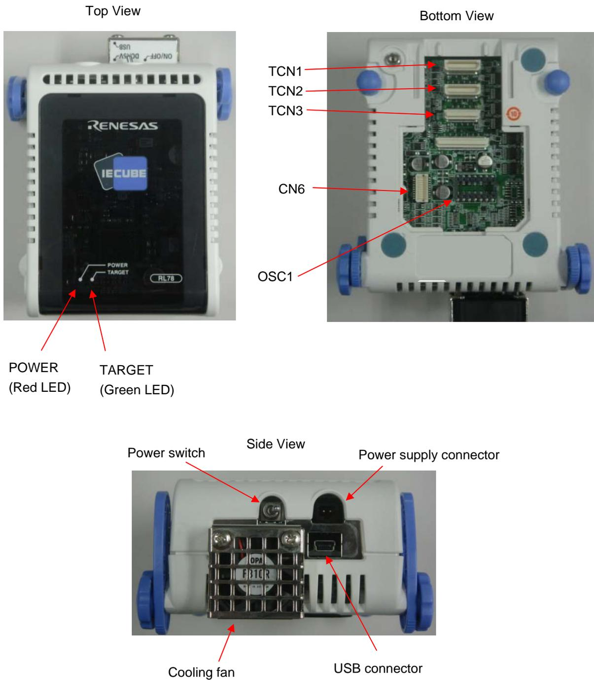
Figure 1-1. Names of Parts of QB-RL78G1A
