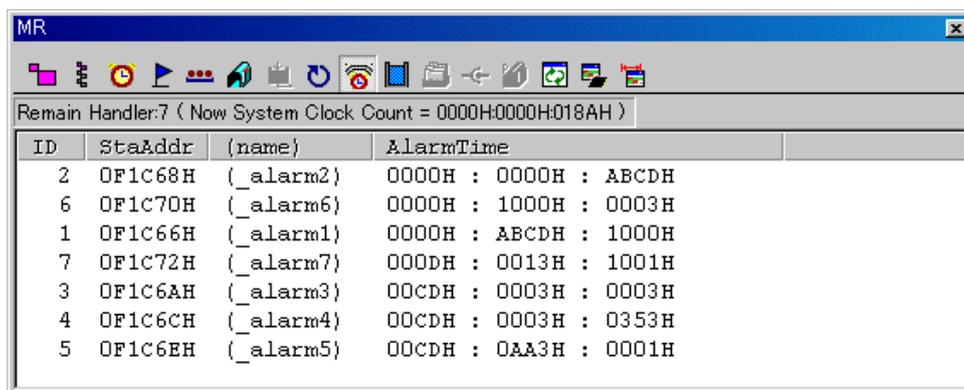
When the realtime OS is MRxx conformed to uITRON specifications V.3.0, the following data is displayed in the status bar.
