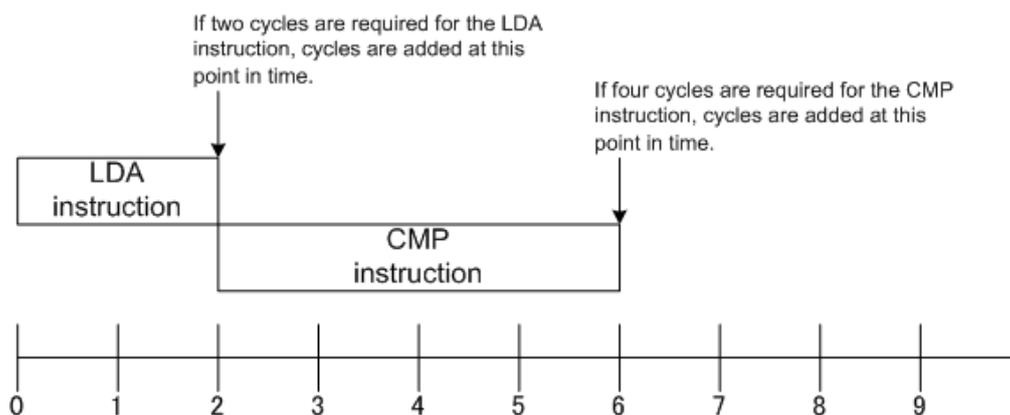
In the above example, no cycles are added while the LDA or CMP instruction is being executed. The cycles required for each instruction are added after instruction execution.
