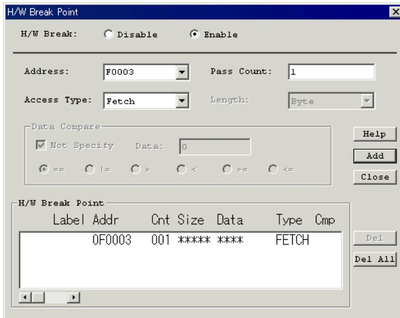
When the Add button is clicked, the breakpoint is added to the breakpoint list under the dialog. Please click the Close button after completing the hardware breakpoint setting.
