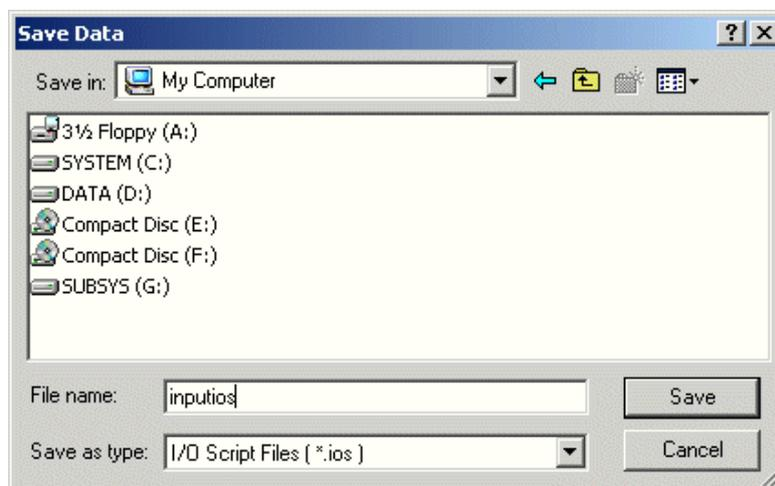
Here, enter the directory and file names in which you want the data you've set to be saved. The saved file can be loaded into the simulator debugger back again by using the [Load...] menus in the I/O Timing Setting window.
