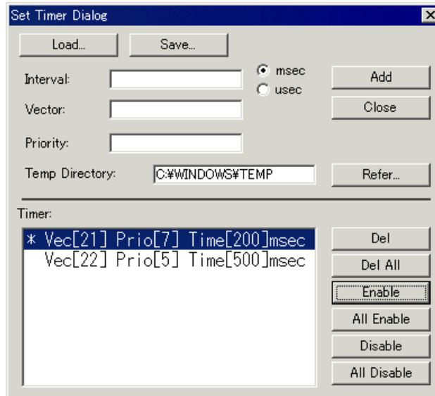
The reenabled virtual interrupt has its asterisk (\*) shown to the left of the virtual interrupt list disappeared. To reenable all virtual interrupts, click the All Enable button. When you've finished setting virtual interrupts, click the Close button.
