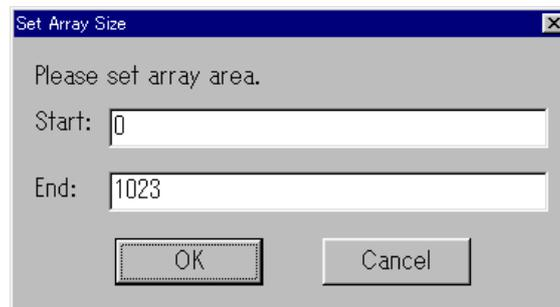
The elements from the index specified in "Start" to the index specified in "End" are displayed. If you specify the value more than the max index of the array, the value is regarded as max index of the array. When you click the "Cancel" button, the elements are not displayed.
