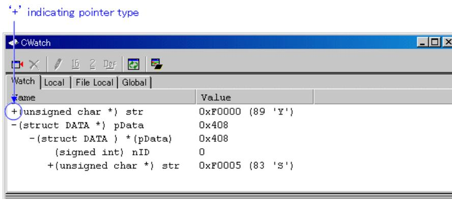
You can double-click on lines indicated by a '+' to see the members of that structure or union. The '+' changes to a '-' while the members are displayed. To return to the original display, double click the line, now indicated by the '-'.
