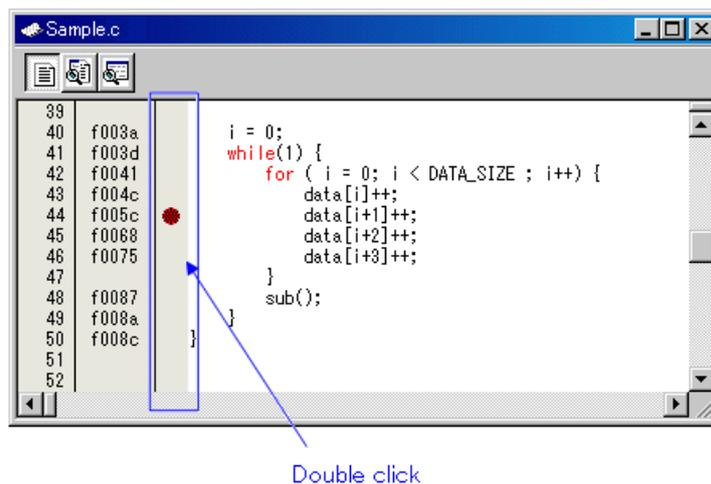
You can delete the break point by double-clicking again in the break point setting area ("S/W breakpoints" column).
