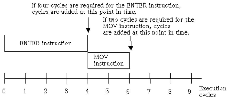
In the above example, no cycles are added while the ENTER or MOV instruction is being executed. The cycles required for each instruction are added after instruction execution.
