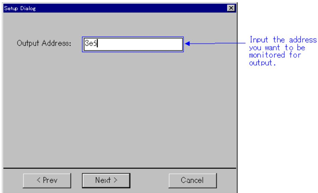
Input the address you want to be monitored for virtual port output in the Output Address column. Then press the Next button.
