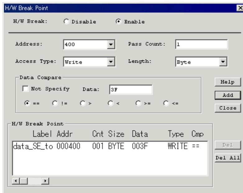
Example) Write data equal to or greater than 3Fh to address 400h
