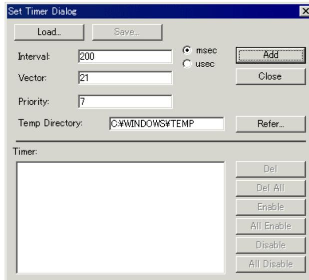
Click the Add button, and the virtual interrupt you've set is added to the list of virtual interrupts in the lower part of the dialog box.
