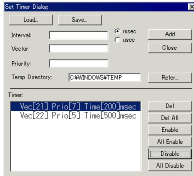
The temporarily disabled virtual interrupt is marked with an asterisk (\*) to the left of the virtual interrupt list.
