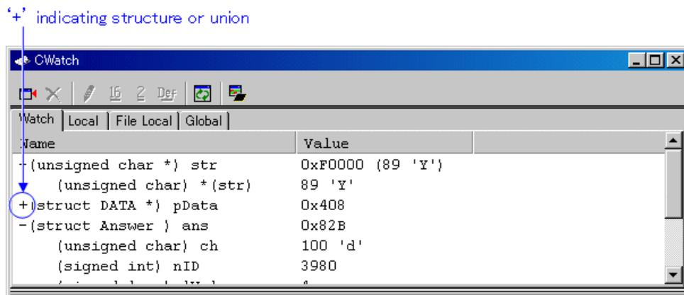
You can double-click on lines indicated by a '+' to see the members of that structure or union. The '+' changes to a '-' while the members are displayed. To return to the original display, double click the line, now indicated by the '-'. This function allows you to check the members of structures and unions.
