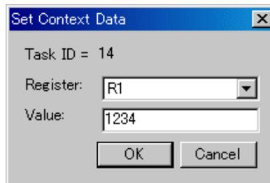
Specify the register to be changed in the Register field list box and enter the value to be set in the "Value:" field.
