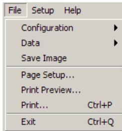
The file menu allows the user to load or save a data record or configuration file as well as print the current display. Data is stored as an ASCII file in comma-separated value (CSV) format. Configuration files are binary.
