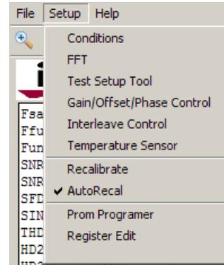
The Conditions dialog sets up the basic operating parameters of the system based on the installed daughter card (see Figure 6). Most of these settings are automatically detected by reading an EEPROM on the daughter card and should not be changed. The current state of the daughter card is indicated in red text under 'Current ADC Configuration'. This information can help guide the selection of motherboard modes to match the ADC operating state.
