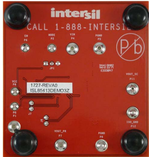
Figure 3. ISL85413DEMO3Z Evaluation Board Bottom View
