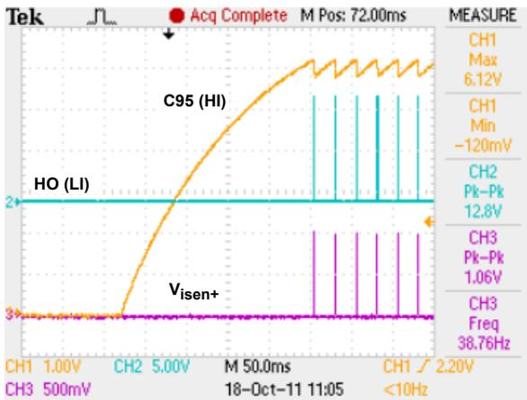
FIGURE 10. START-UP TIMING DIAGRAM FOR LOAD CYCLE
