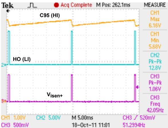
FIGURE 11. STEADY STATE TIMING DIAGRAM FOR LOAD CYCLE
