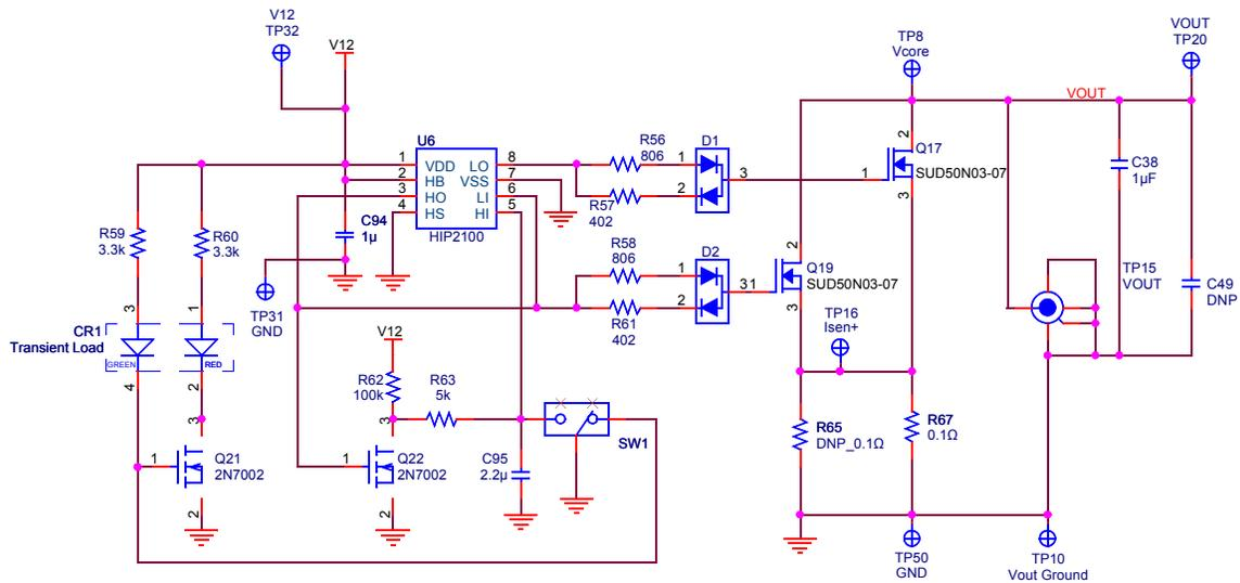
FIGURE 4. TRANSIENT LOAD GENERATOR SCHEMATIC ON ISL8200MEVAL2PHZ
