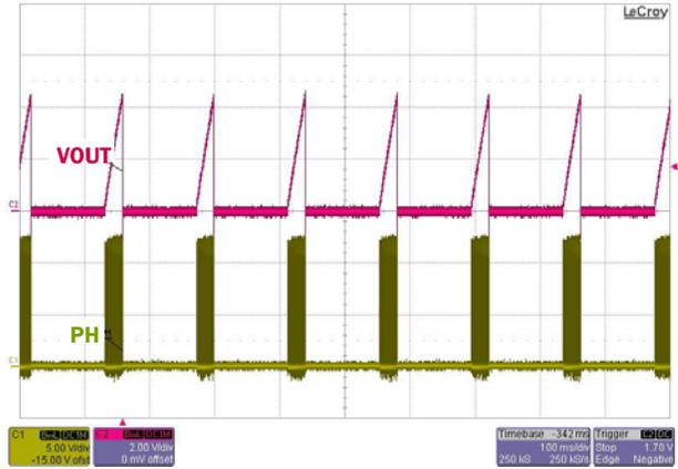
FIGURE 7. OVERCURRENT PROTECTION ( $V_O = 5V$ ,  $LOAD = 40A$ )
