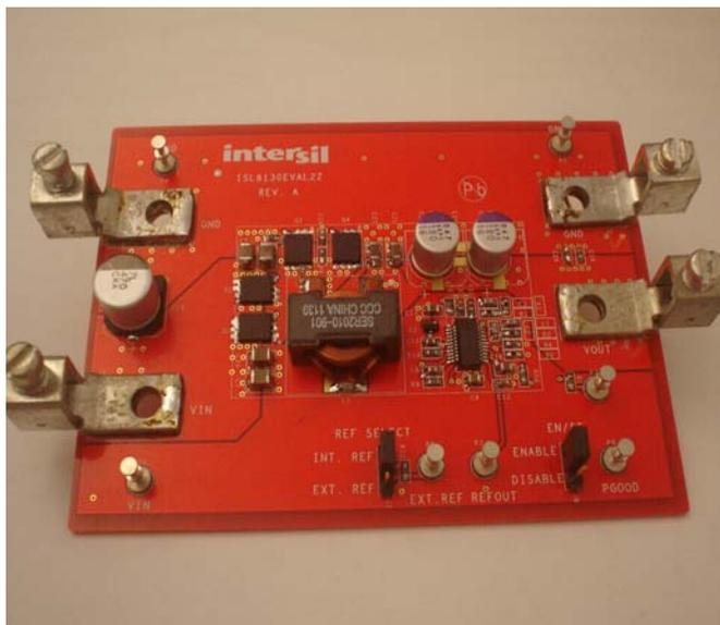
FIGURE 1. PHOTOGRAPH OF THE ISL8130EVAL2Z EVALUATION BOARD
