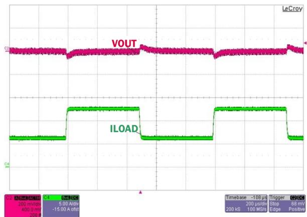
FIGURE 9. LOAD TRANSIENT (25% TO 50% AT 2A/ $\mu$ s)
