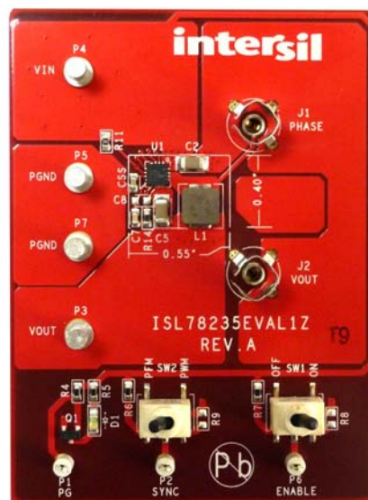
FIGURE 1. ISL78235EVAL1Z EVALUATION BOARD PHOTO
