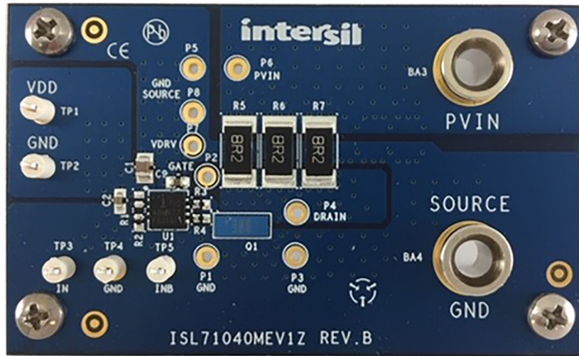
Figure 2. ISL71040MEV1Z Evaluation Board, Top View
